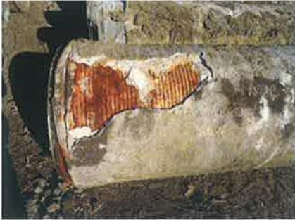
Figure 2- Typical External Corrosion
