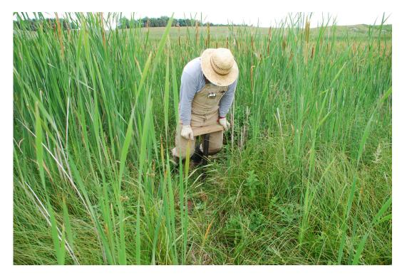
*Figure 2. Fred Anderson pushing a core barrel (with an interior plastic sleeve) through organicrich sediment in the Tolna Coulee.*
