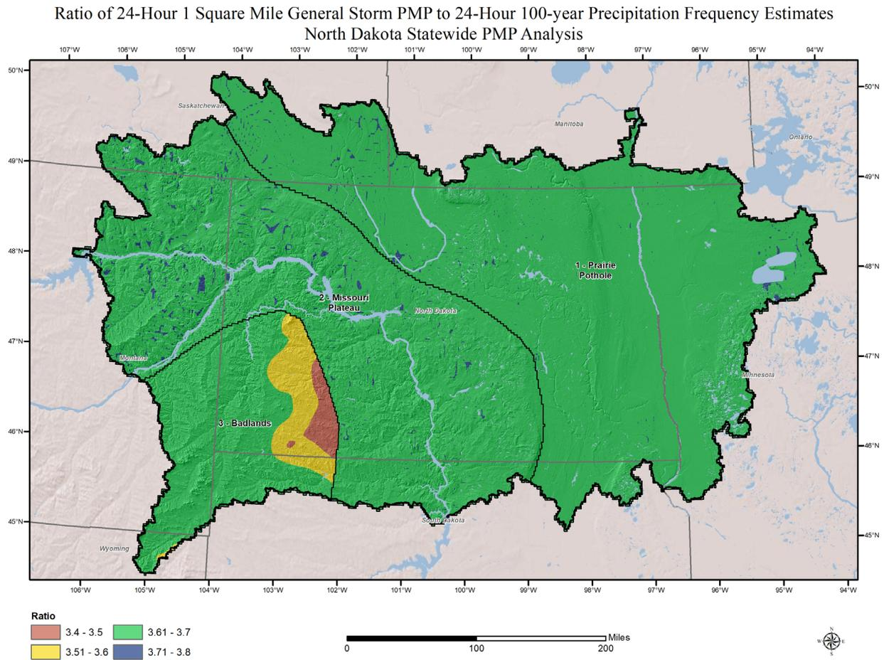
**Figure 14.13: Ratio of 24-hour 1-square mile General storm PMP to 100-year precipitation**
