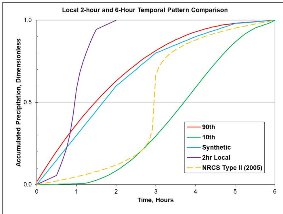
Figure 13.20: Comparison of final Local storm patterns to NRCS Type II temporal pattern
