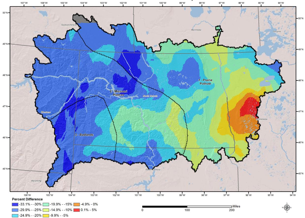
Figure 14.8: Local Storm 200 mi<sup>2</sup> Percent Difference from HMR 51 – 24 hour
