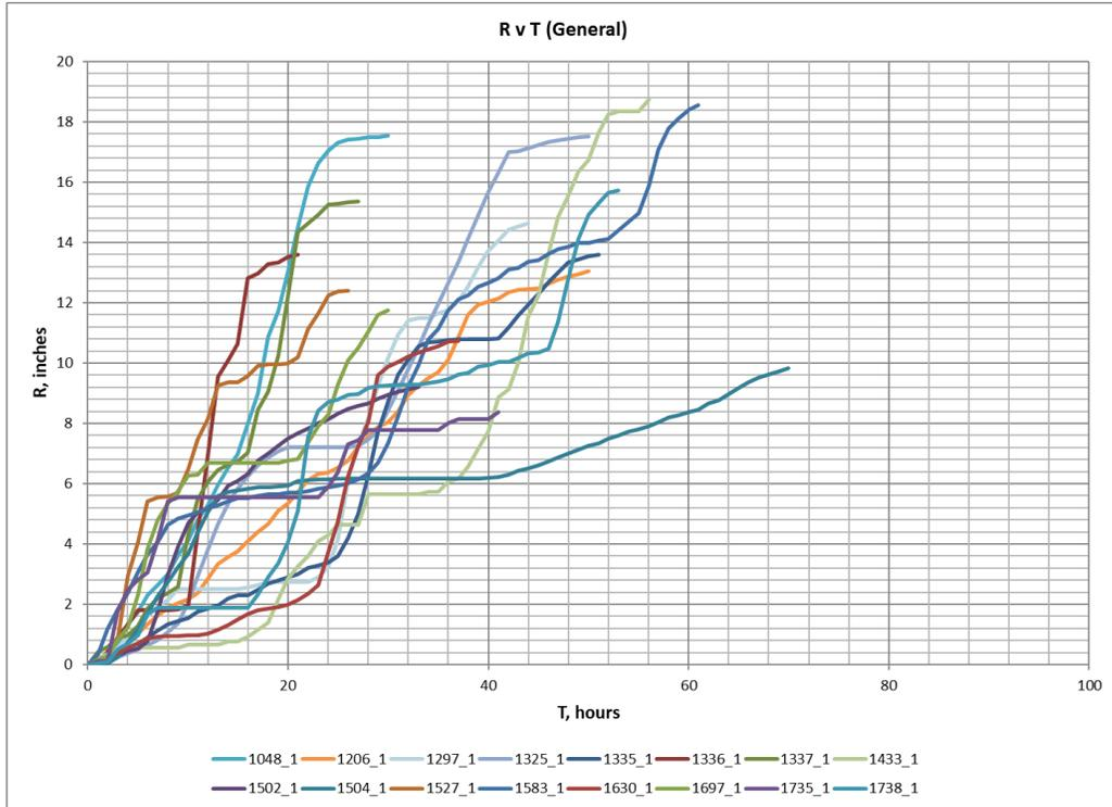
Figure 13.4: SPAS Rainfall (R) versus time (T) for General Type Storm
