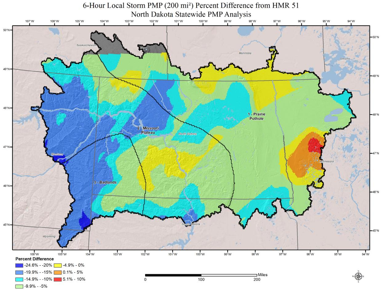
Figure 14.4: Local Storm 200 mi<sup>2</sup> Percent Difference from HMR 51 – 6 hour
