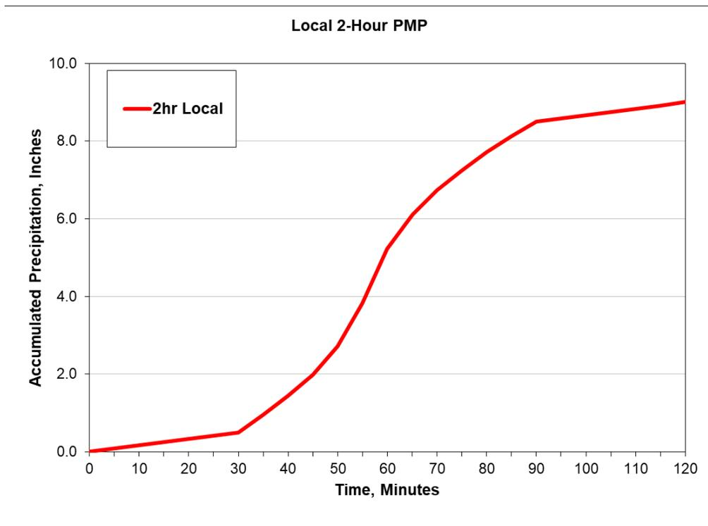
Figure 13.16: Hypothetical 2-hour local storm pattern at 5-minute time step
