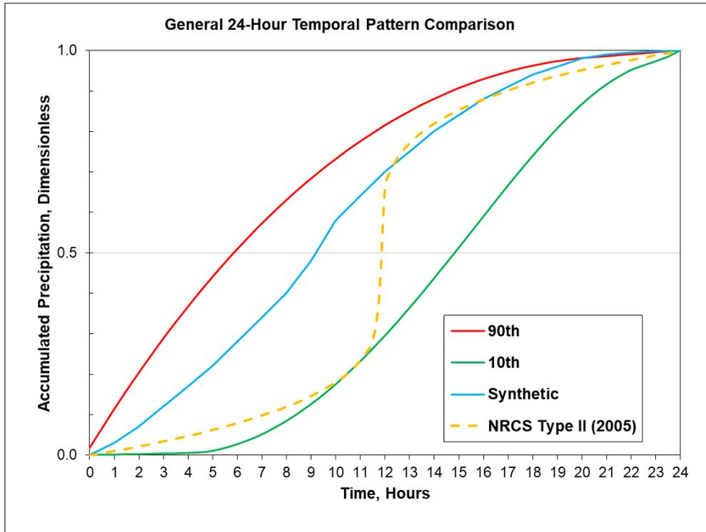
Figure 13.21: Comparison of final General storm patterns to NRCS Type II temporal pattern
