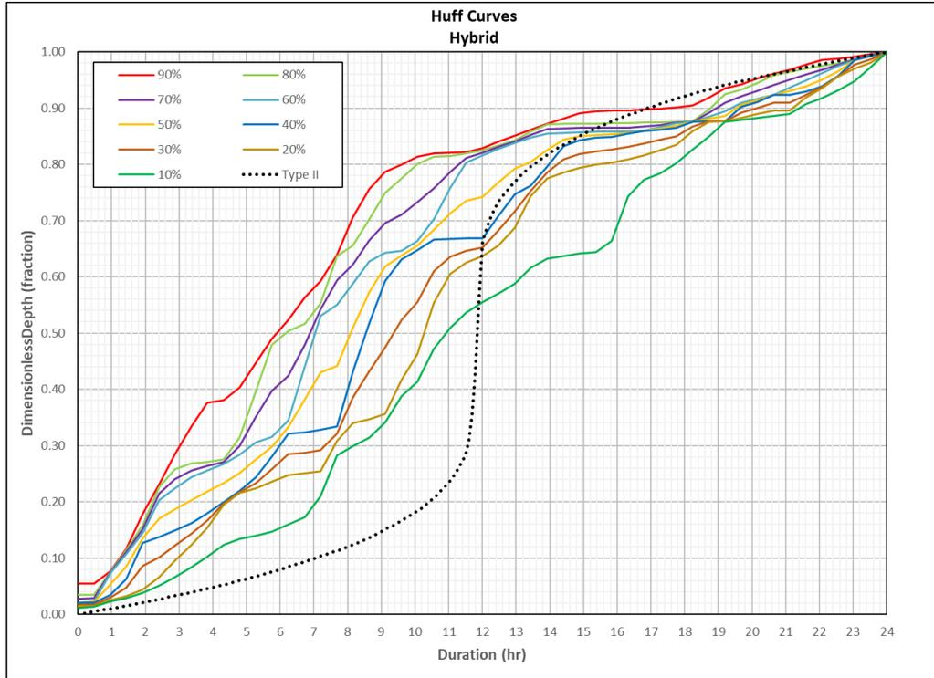
Figure 13.12: Raw Huff temporal curves for 24-hour Hybrid storms
