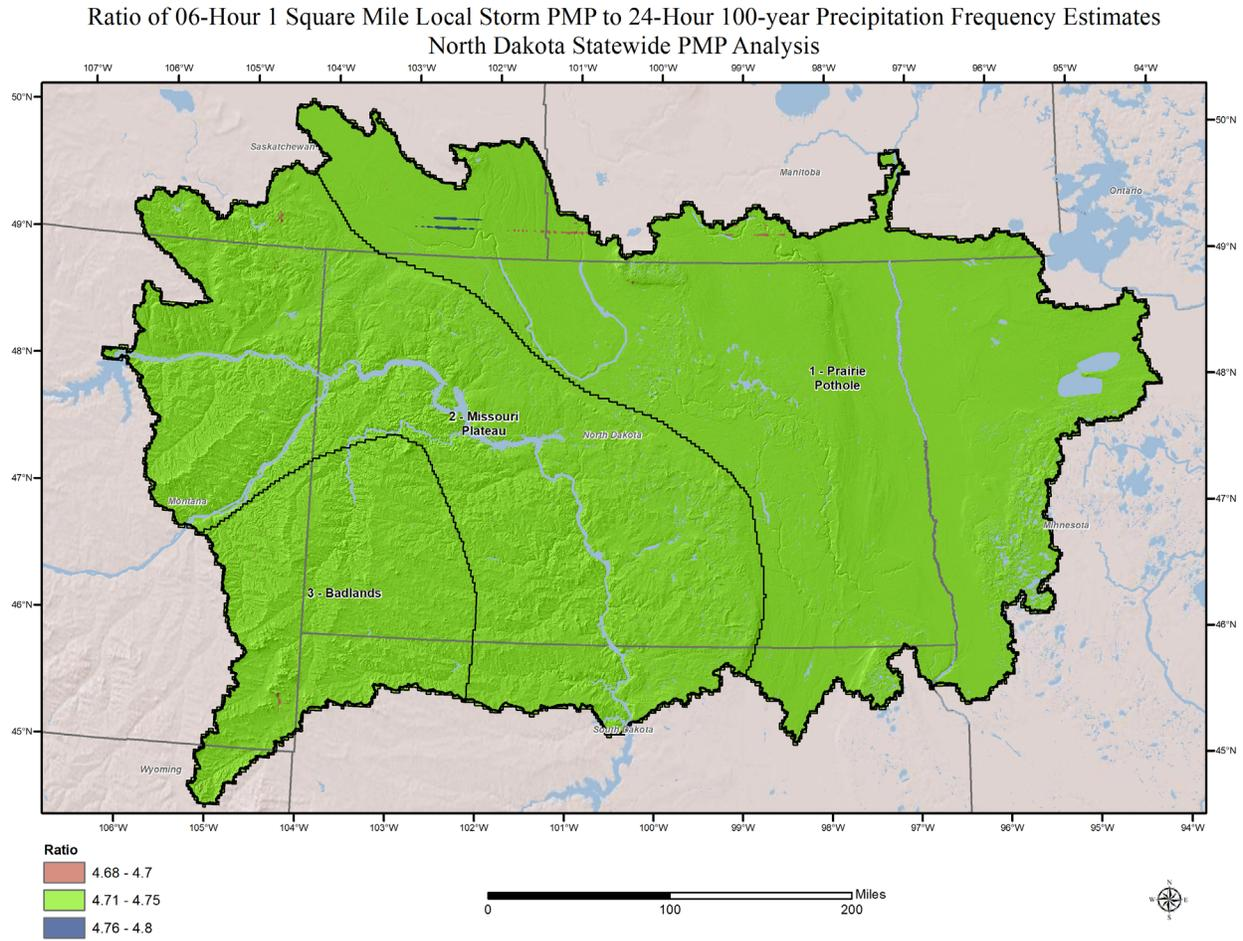
Figure 14.12: Ratio of 6-hour 1-square mile Local storm PMP to 100-year precipitation
