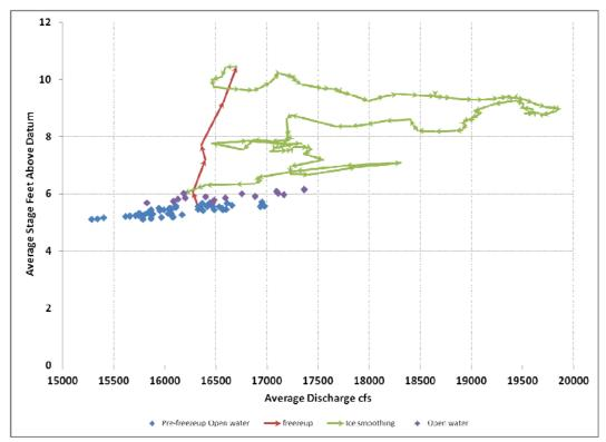
Figure 8 Rating curve for average stage and discharge during freezeup
