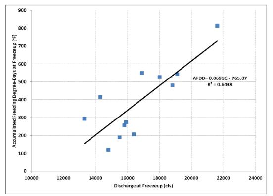
Figure 9 Accumulated Freezing Degree-Days (AFDD) at freezeup as a function of discharge
