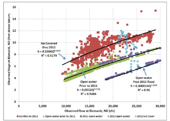
Figure 11 Open water and ice covered rating curves for period before 2011 flood and after
