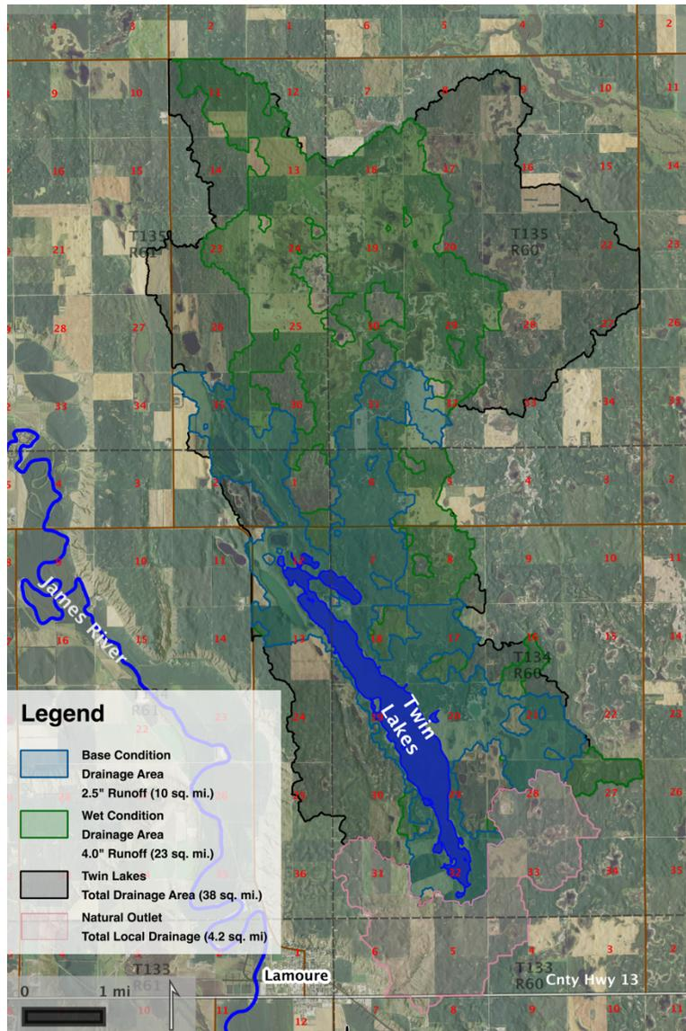
**Figure C2:** Twin Lakes contributing drainage area for the 2.5” (light blue area) and 4.0” (green) runoff events.
