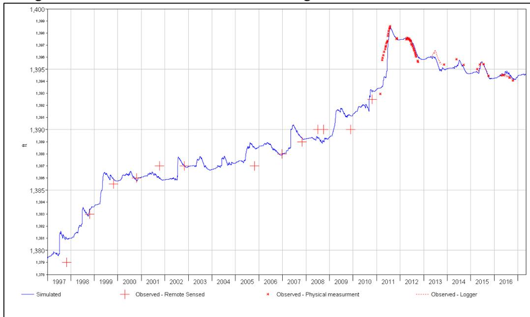
**Figure 8:** Simulated (blue line) and observed (red symbols) lake elevations from 1997 through early 2017.
