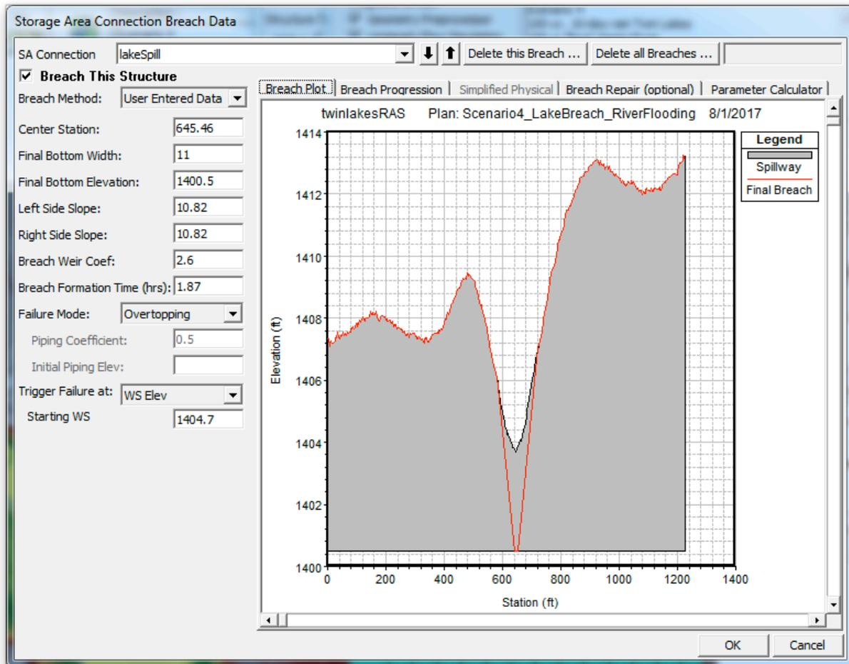
**Figure D6:** Lake spill point breaching parameters
