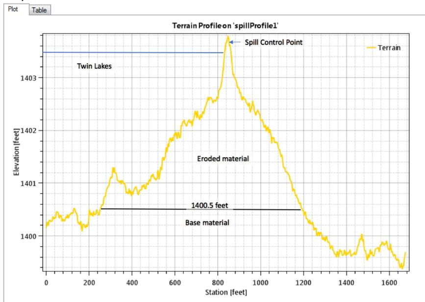
**Figure D5:** Cross section of outlet control topography and breach elevation (Note: Vertical scale is greatly exaggerated).
