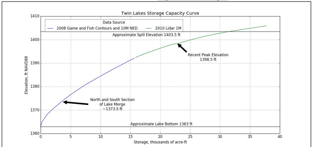
**Figure 5:** Twin Lakes storage capacity curve.
