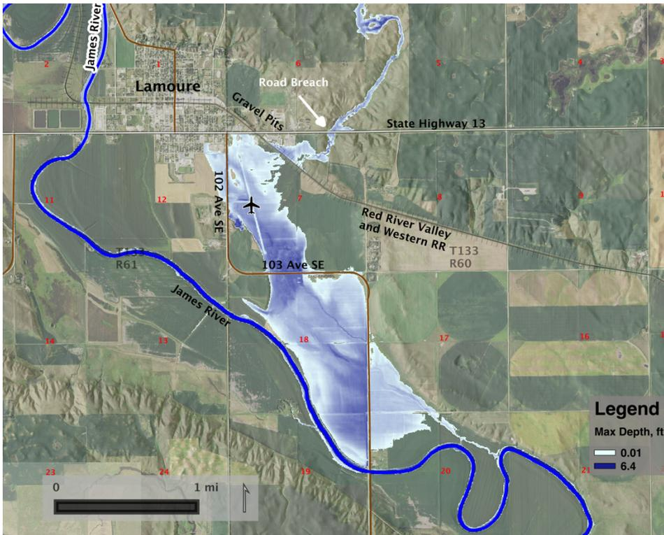
**Figure 12:** Scenario 3 inundation caused by a 100-year, 10-day rainfall event over Twin Lakes with the starting elevation of the lake at its spill point and assuming the lake outlet and State Highway 13 have breached.
