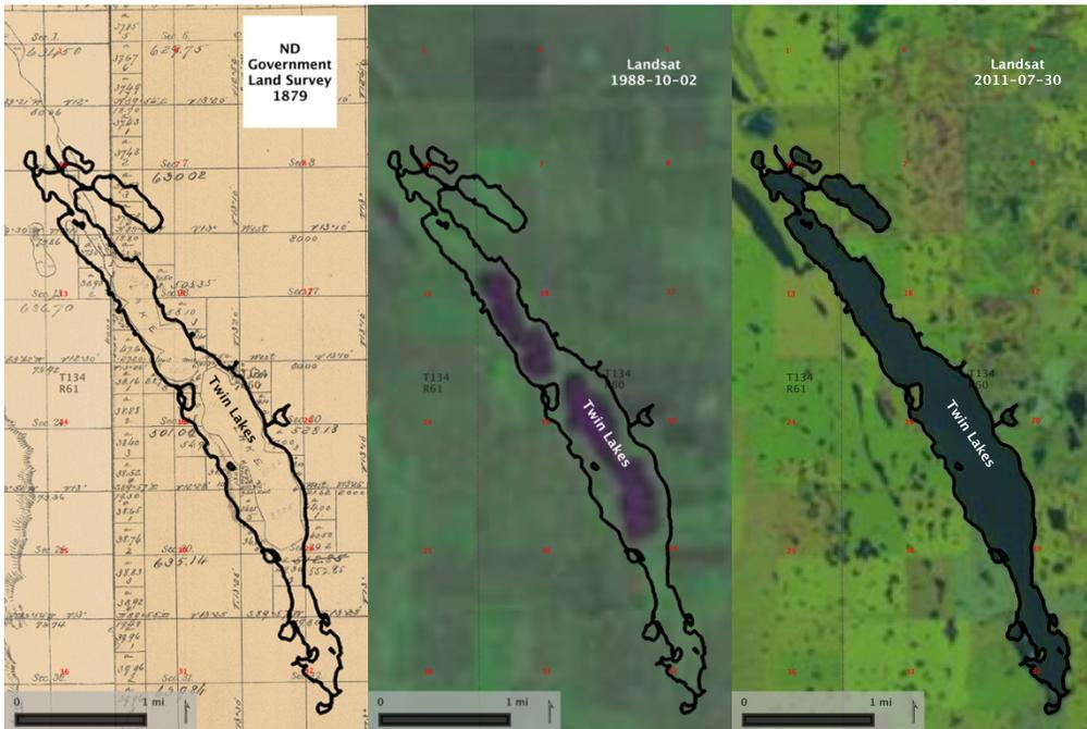
**Figure 6:** Outline of Twin Lakes footprint at elevation 1395 ft NAVD88 overlying 1879 General Land Office survey plat outline, 1988 Landsat image, and a 2011 Landsat image.
