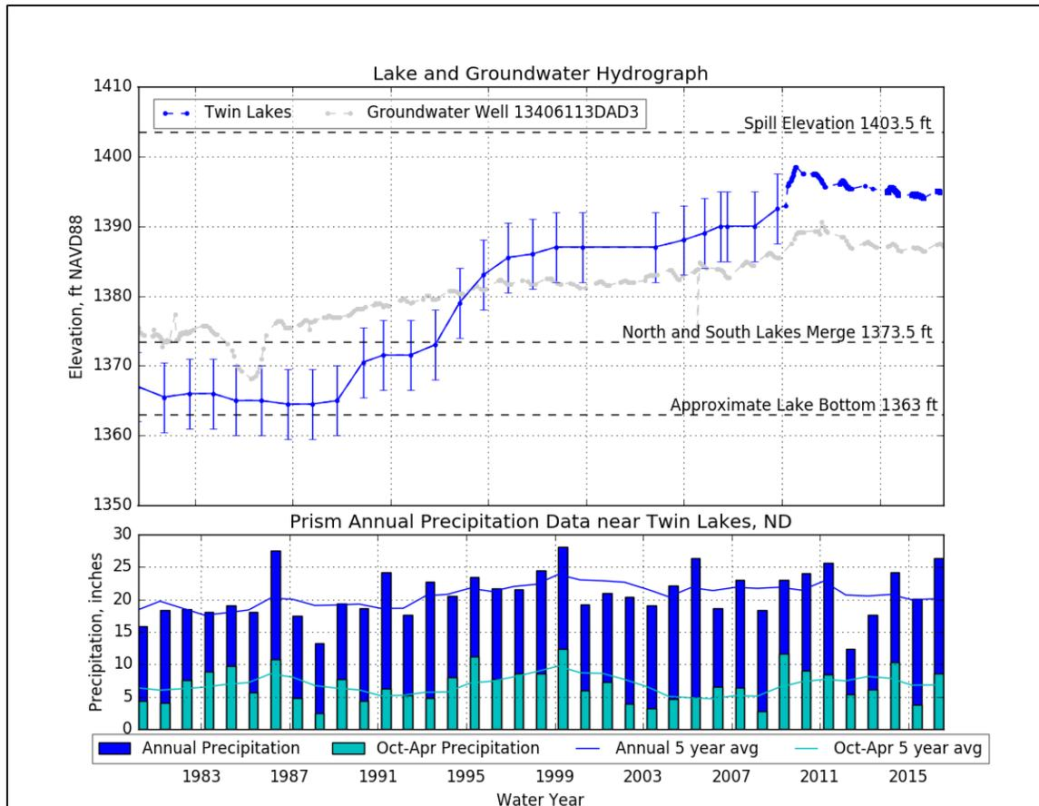
**Figure 7:** Twin Lakes hydrograph and annual precipitation data.
