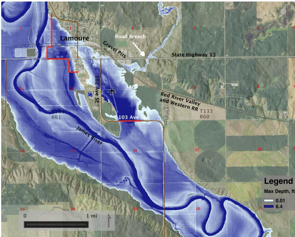
**Figure 13:** Scenario 4 inundation caused by Scenario 3 along with a 100-year flood event on the James River. Inundation within the town and airport is from the lake.
