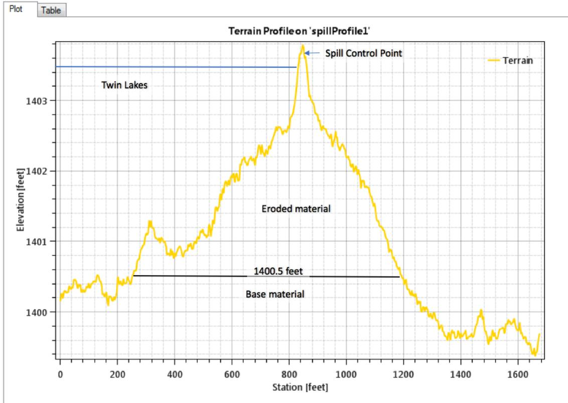
**Figure 11:** Cross section of outlet control topography and breach elevation (Note: Vertical scale is greatly exaggerated).
