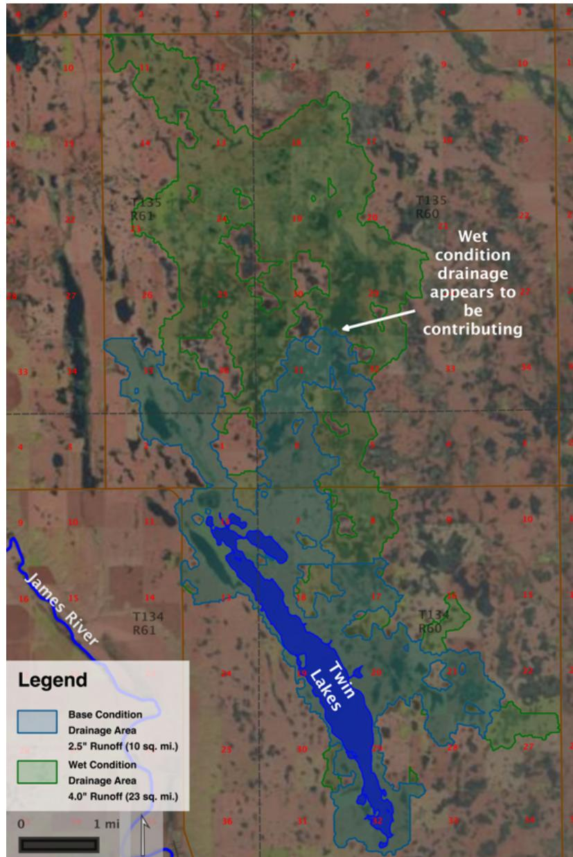
**Figure C6:** Landsat image collected on May 2, 2011 showing the wet condition drainage area connected to the base condition area.
