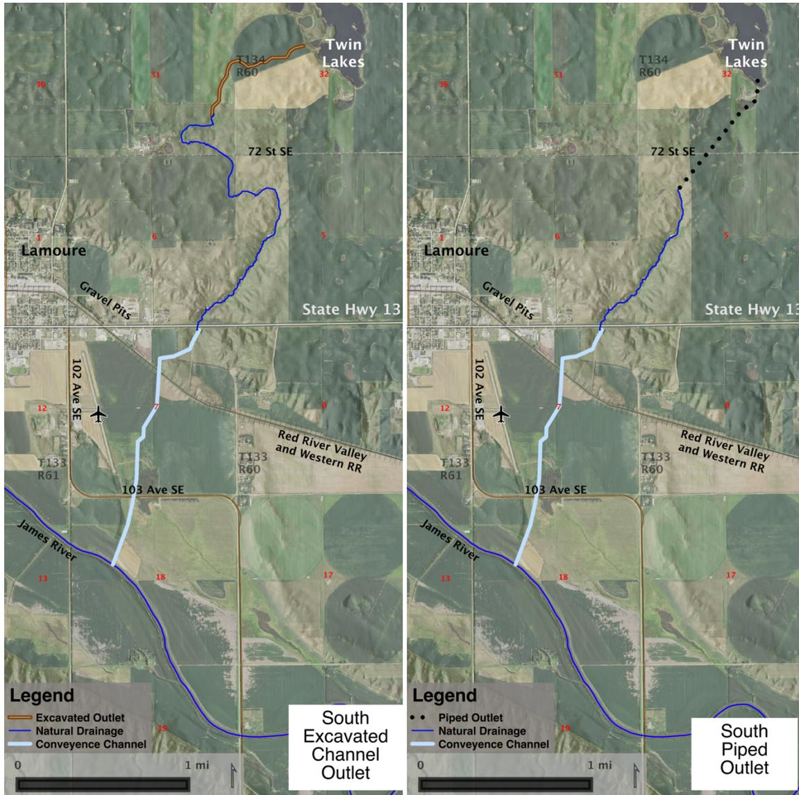
**Figure E1 (left):** South Excavated Channel Outlet Option.
