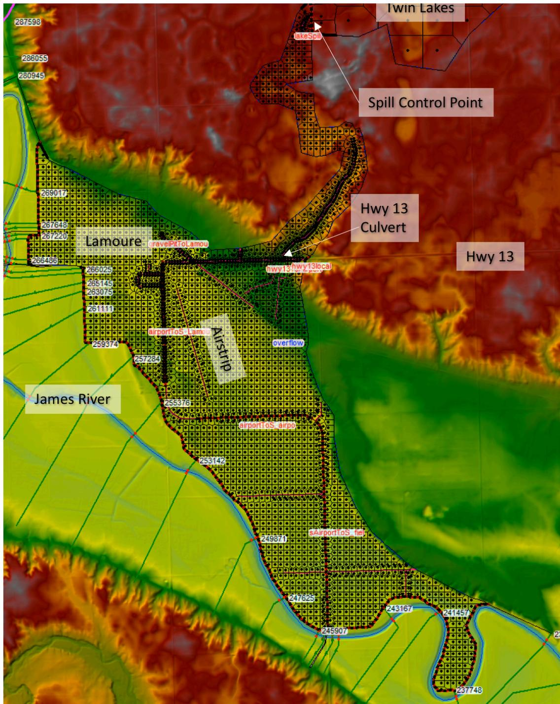
**Figure D2:** Overflow 2D area, Hwy 13 culvert, and lake overflow control point with LiDAR terrain as a background.
