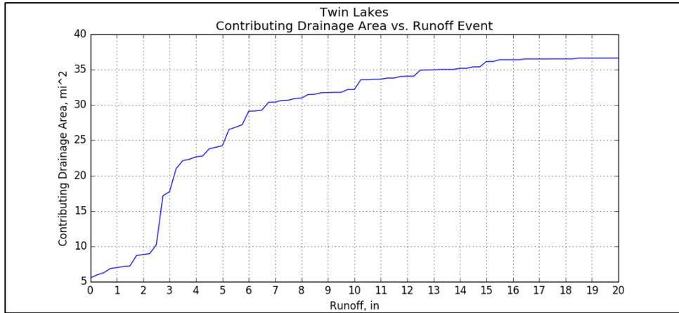
**Figure 3:** Twin Lakes contributing drainage area vs. runoff event.
