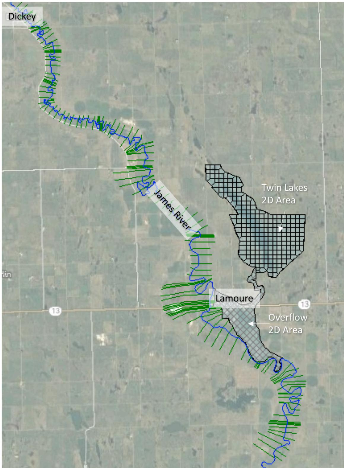
Figure D1: Hydraulic model domain.
