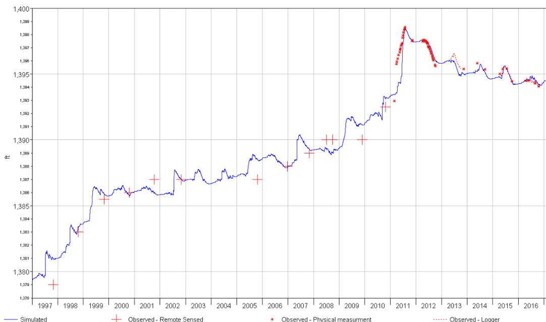
**Figure C4:** Simulated (blue line) and observed (red symbols) lake elevations from 1997 through early 2017.
