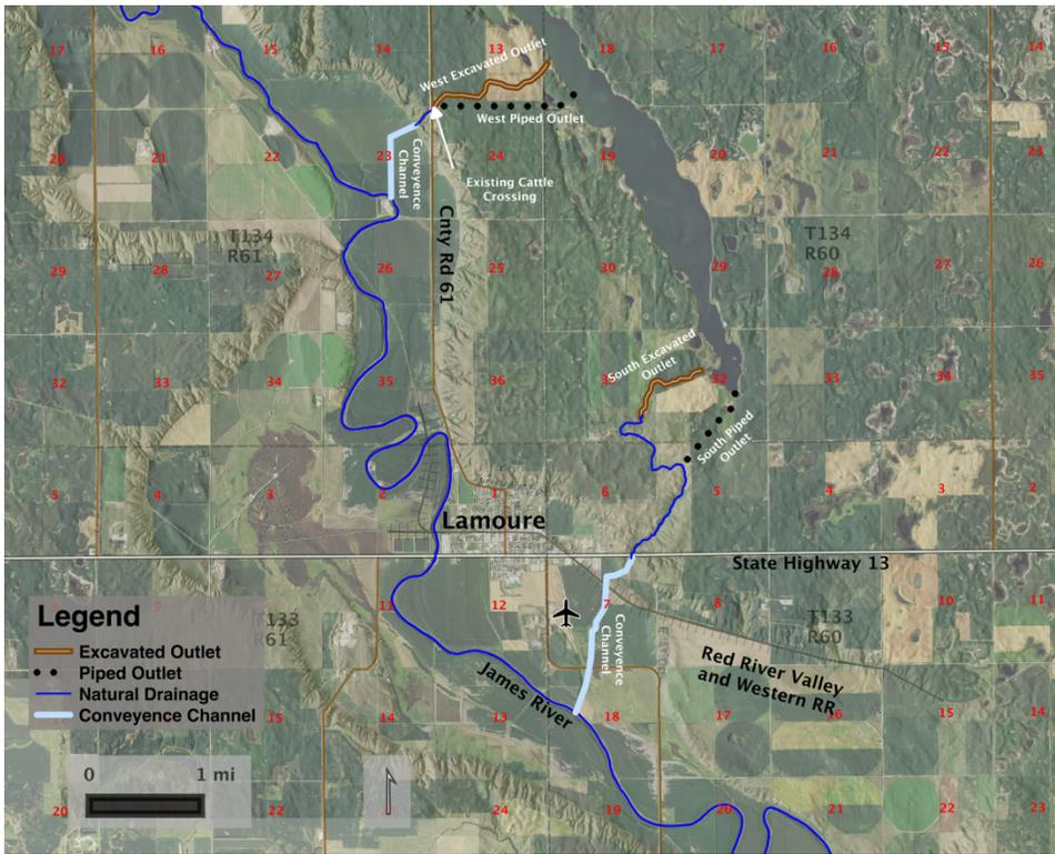
**Figure 14:** Evaluated gravity drain options.
