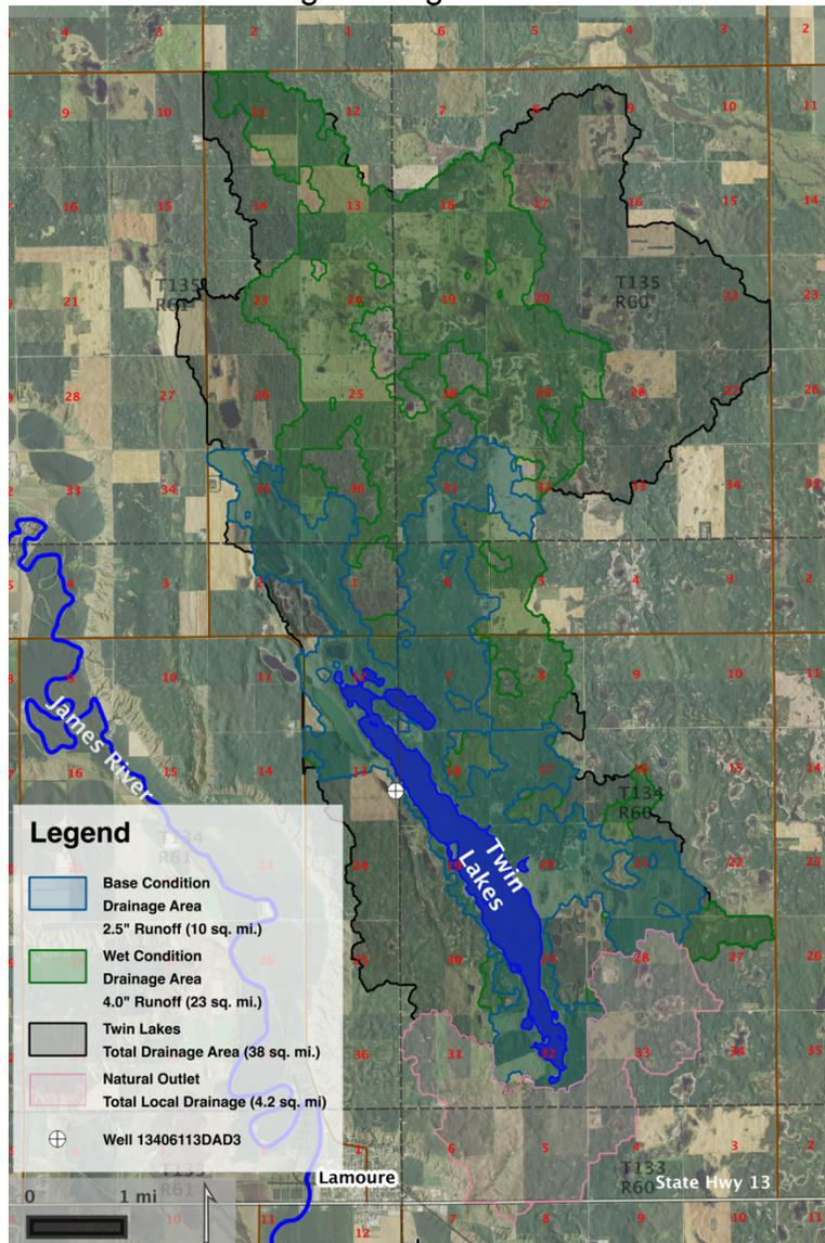
**Figure 4:** Twin Lakes contributing drainage area for the 2.5" (light blue area) and 4.0" (green) runoff events.
