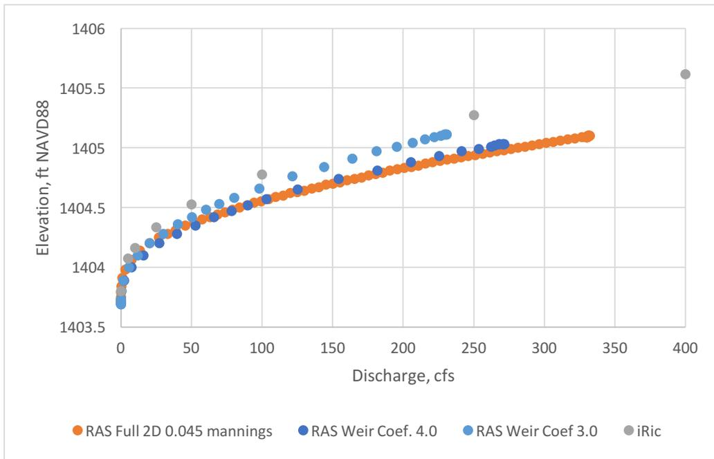
**Figure D4:** Evaluated spill point rating curves.
