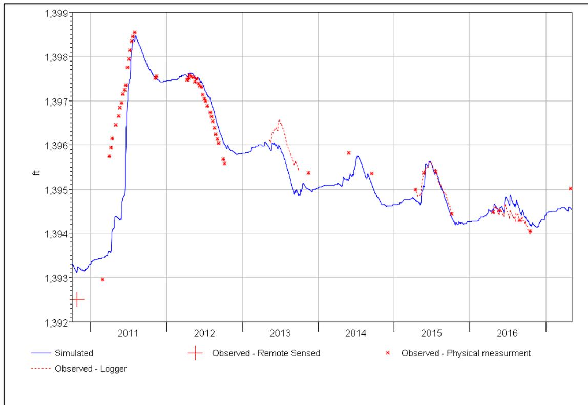
**Figure 9:** Simulated (blue line) and observed (red symbols) lake elevations during the period of physical observations, late 2010 through early 2017.
