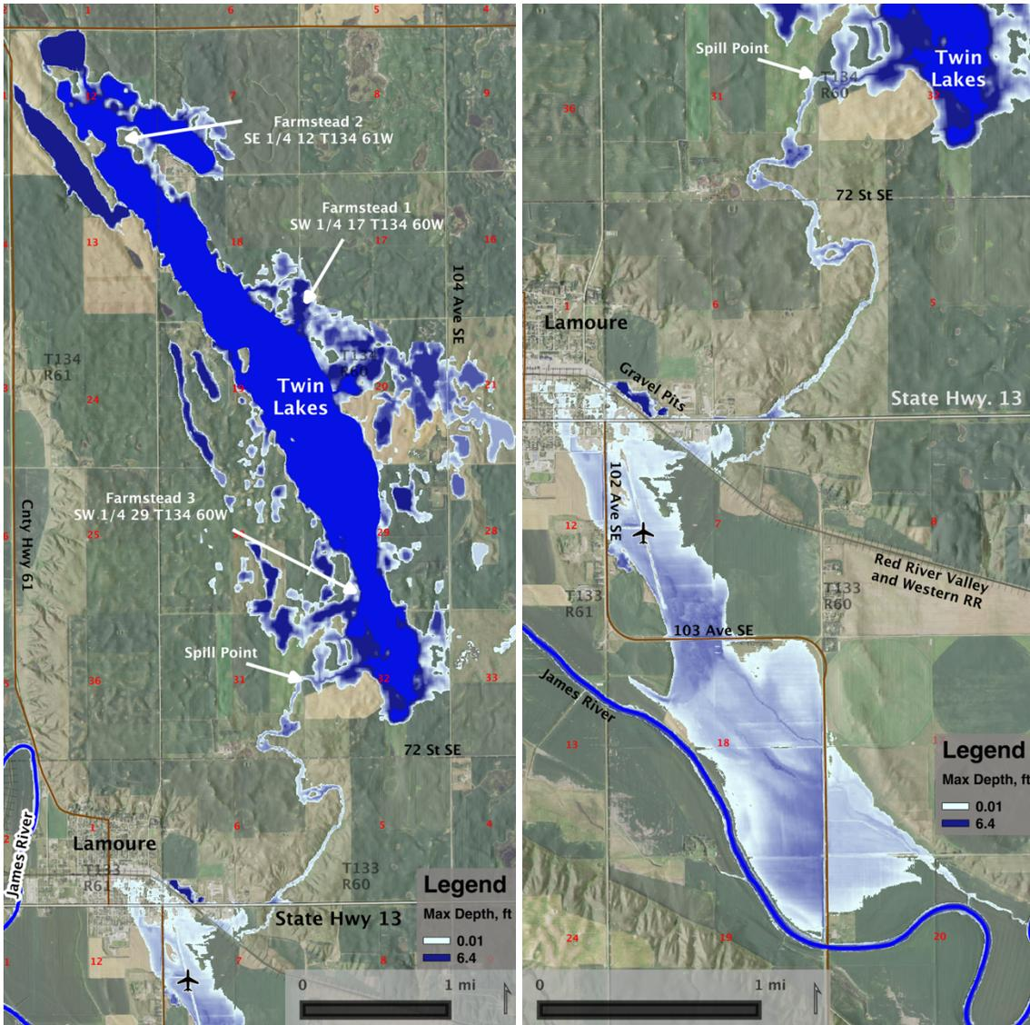
**Figure 10:** Scenario 2 inundation caused by a 100-year, 10-day rainfall event over Twin Lakes with the starting elevation of the lake at its spill point.
