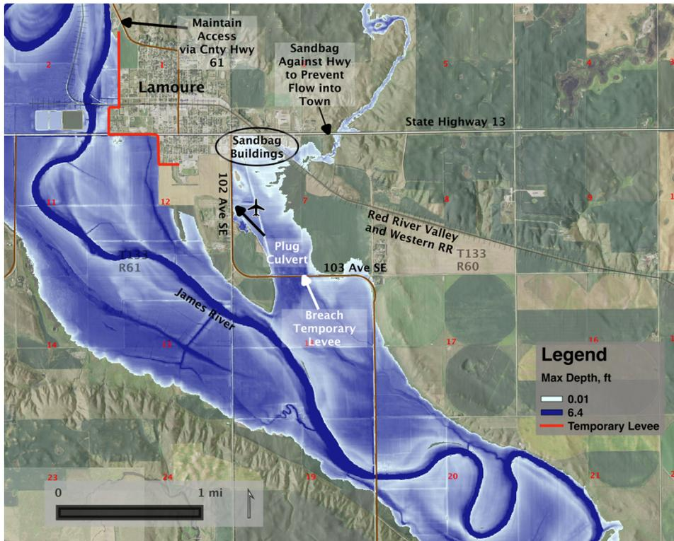
**Figure 15:** Simulated inundation for Scenario 4 with Emergency Protection Measures in place.
