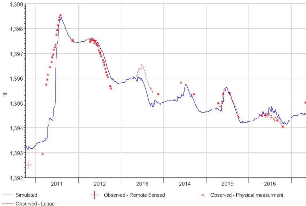
**Figure C5:** Simulated (blue line) and observed (red symbols) lake elevations during the period of physical observations, late 2010 through early 2017.
