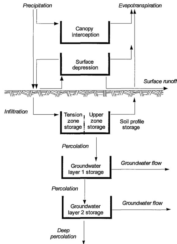
**Figure C3:** Soil Moisture Accounting Method (SMA) diagram (Hydrologic Engineering Center, 2000).
