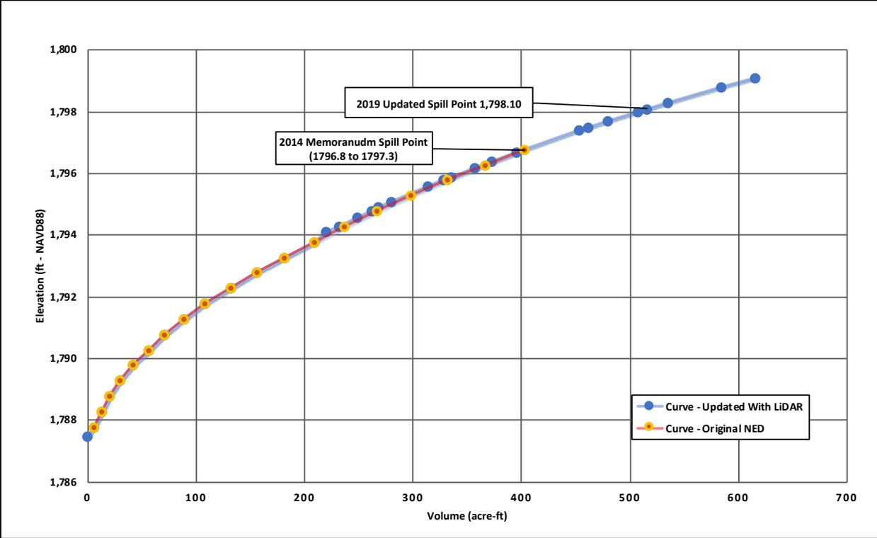
Figure 7. Strasburg Slough elevation-capacity curve
