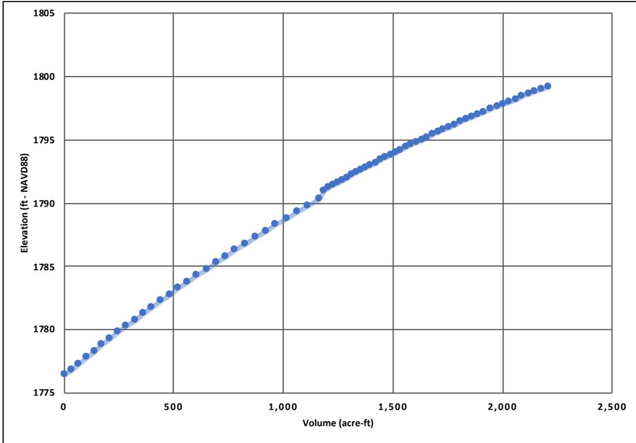
**Figure 8.** City lagoon elevation-capacity curve
