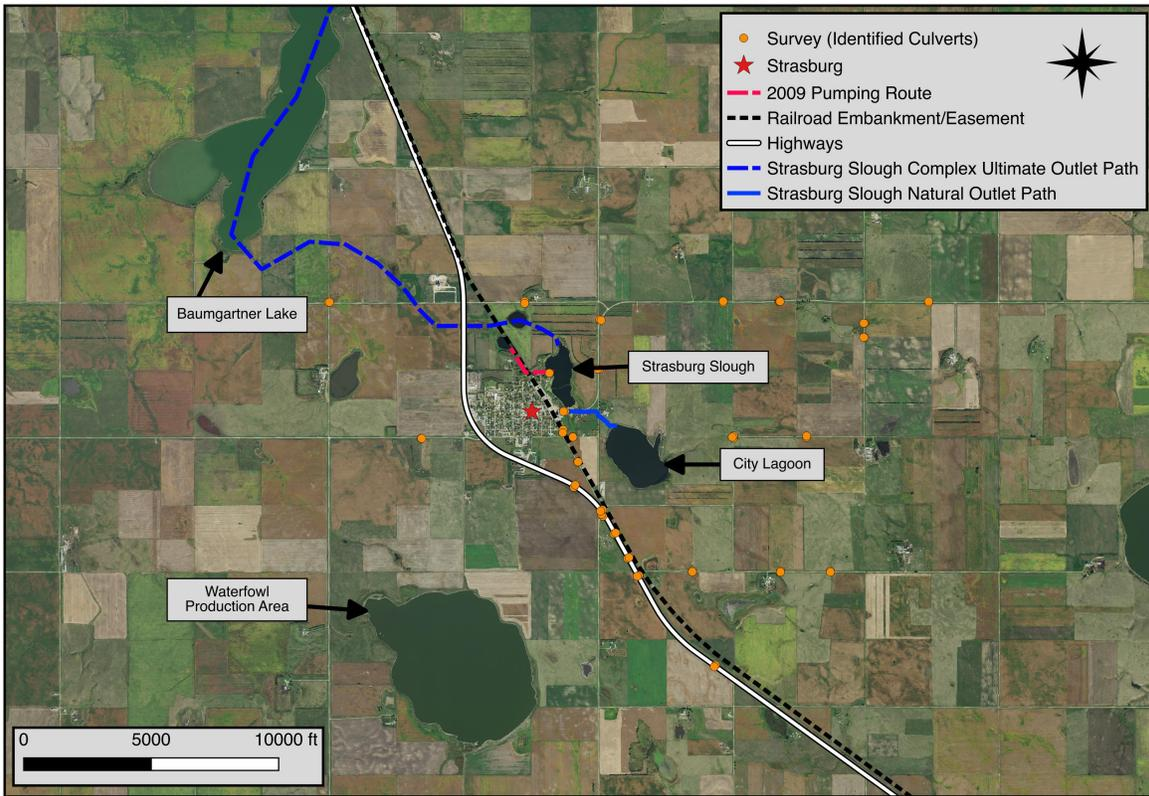
**Figure 4.** Culvert survey conducted for Strasburg Slough analysis
