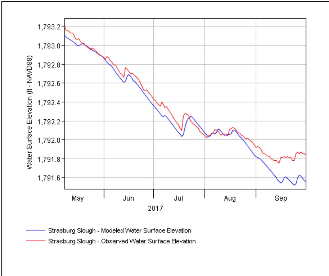
**Figure 18.** 2017 Strasburg Slough water surface comparison
