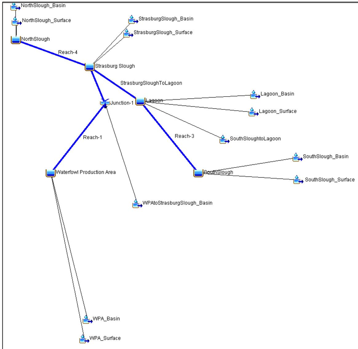
**Figure 15.** Screenshot of the hydrologic model's conceptual layout
