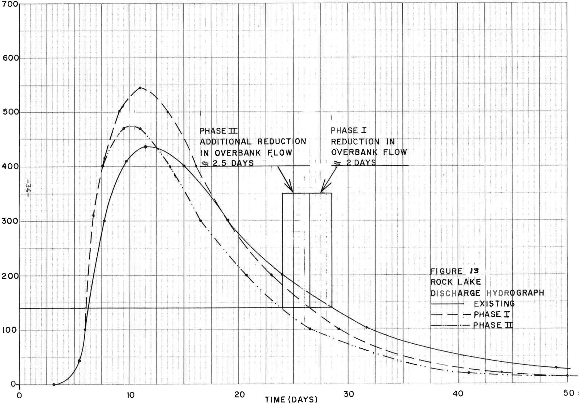
The Phase I project is a proposed cleanout to return Badger Creek to its condition prior to the siltation and growth of vegetation that has occurred over many years. The completion of the project will re-establish what would have been existing conditions had the creek been maintained. Therefore, any impacts from such a project would be those that would have occurred naturally with proper maintenance.
