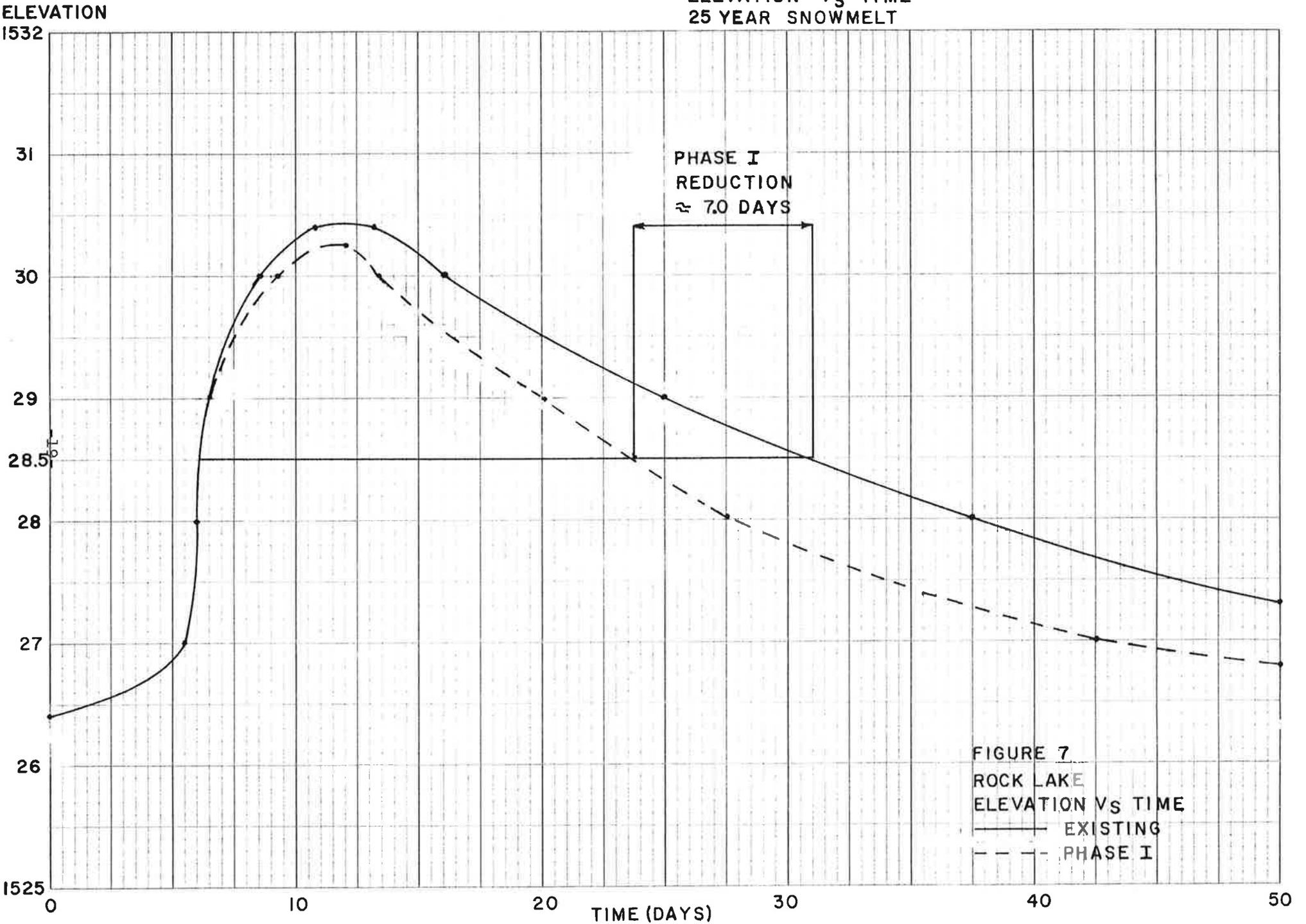
Badger Creek was evaluated for various flows under both existing and improved (Phase I) conditions, to determine the elevations that occur on Rock Lake for a given discharge into Badger Creek. The starting elevation for Rock Lake was set at 1526.4 msl, based on preliminary surveys. The elevation-discharge curves for existing and Phase I conditions shown in Figure 8 illustrates the improved removal efficiency of Badger Creek.
