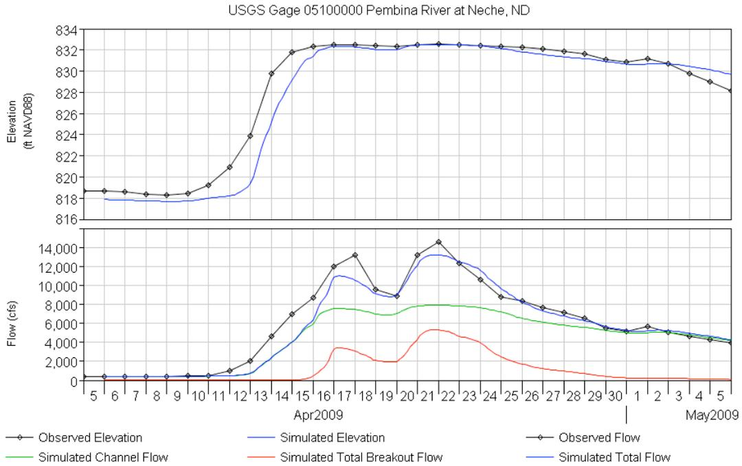
**Figure 9:** 2009 flood event simulated and observed stage and flow at USGS gage 05100000 Pembina River at Neche, ND.
