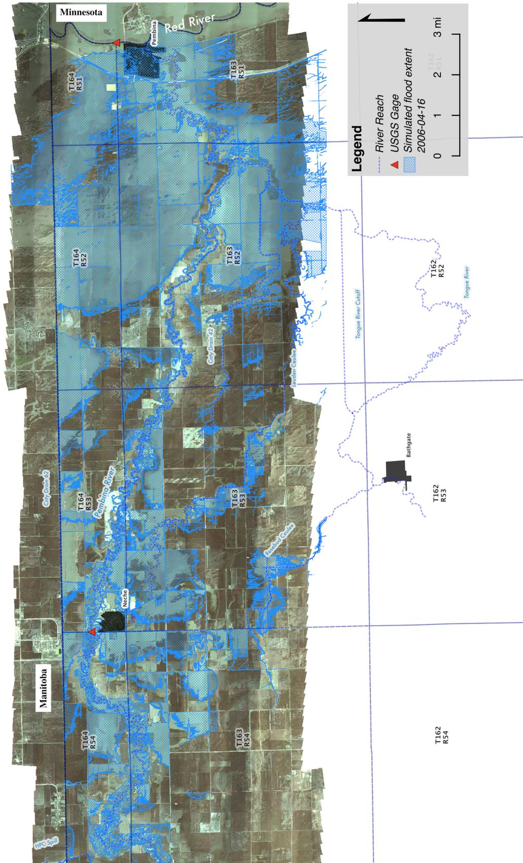
**Figure 6:** 2006 flood event simulated and observed flood extents. The aerial image was collected near the peak of the flood and the simulated flood extent of April 16, 2006 is shown.
