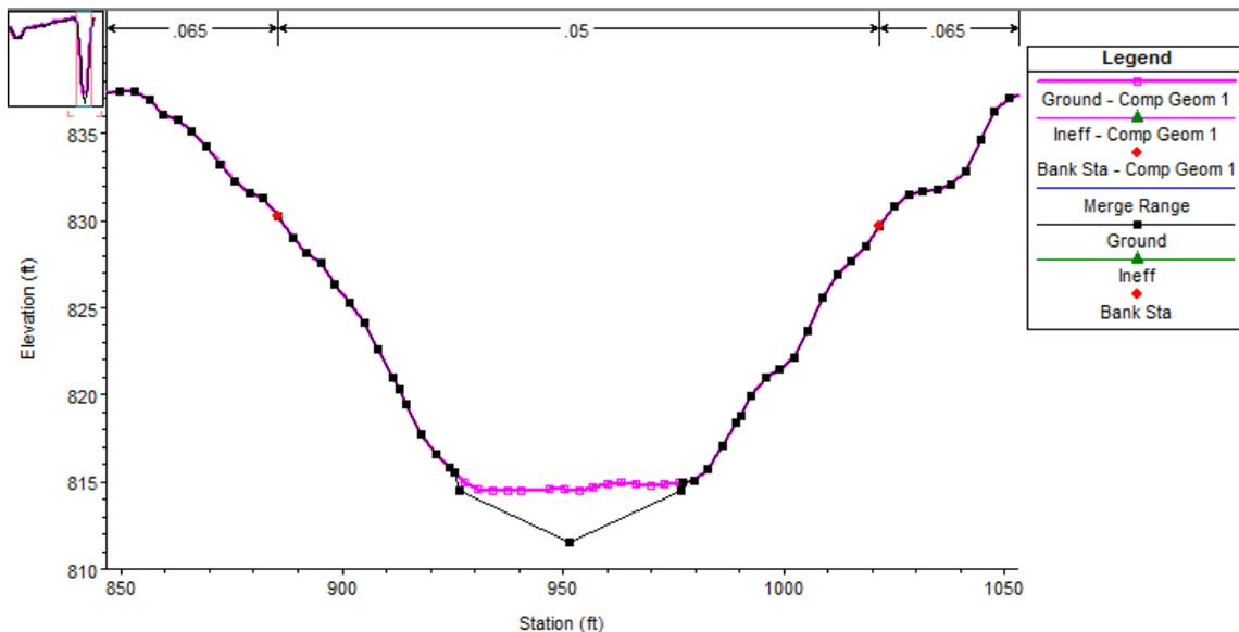
**Figure 4:** Cross-section terrain showing synthetic bathymetry (black line) and raw LiDAR elevations (pink line) for Pembina River cross-section 52.2471 (USGS gage 05100000).
