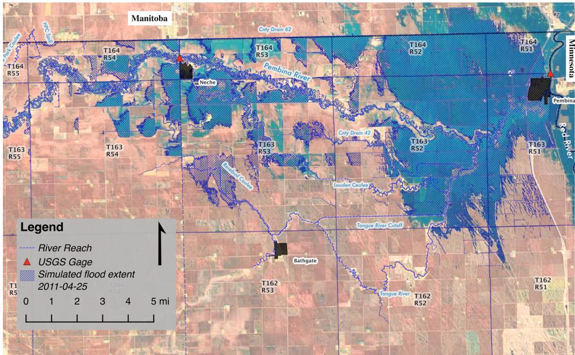
**Figure 12:** Simulated flood extents overlying an April 25, 2011 Landsat image. Landsat image courtesy of the USGS.
