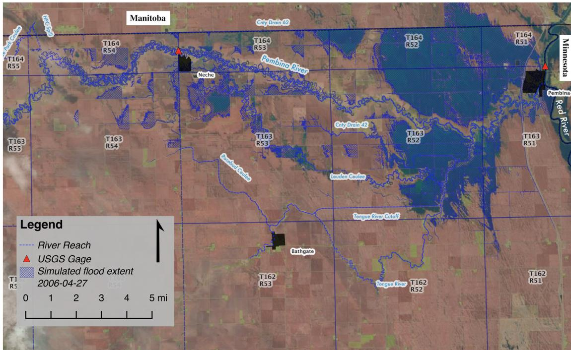
**Figure 8:** Simulated flood extents overlying an April 27, 2006 Landsat image. Landsat image courtesy of the USGS.
