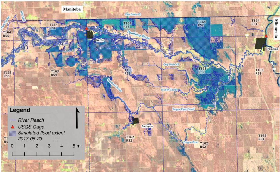
**Figure 14:** Simulated flood extents overlying a May 23, 2013 Landsat image. Landsat image courtesy of the USGS.
