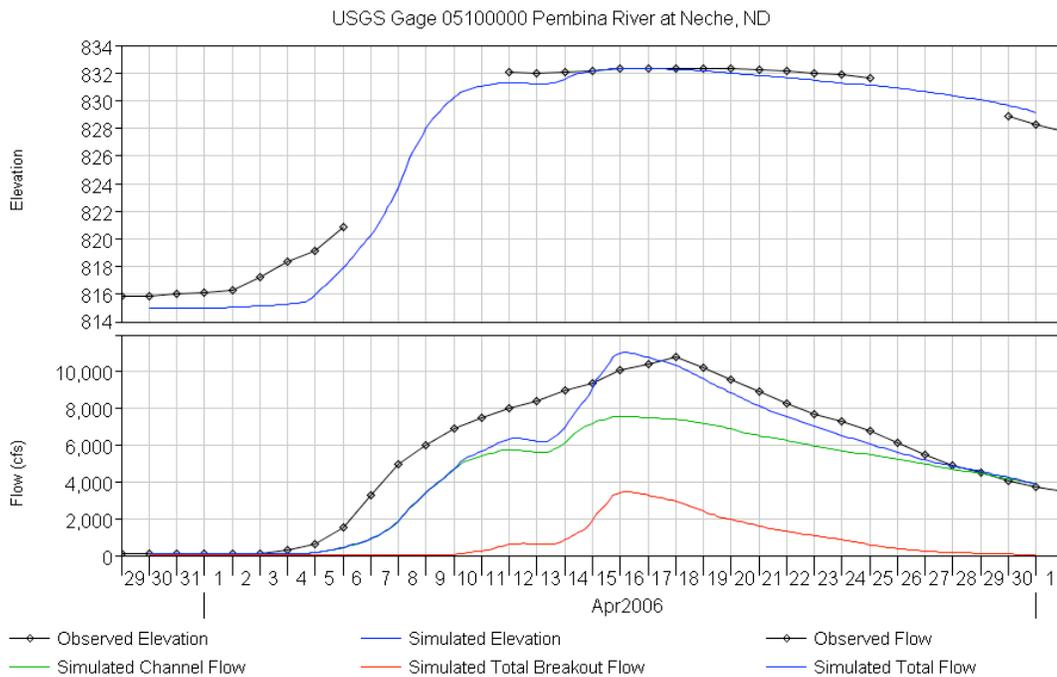
**Figure 5:** 2006 flood event simulated and observed stage and flow at USGS gage 05100000 Pembina River at Neche, ND.
