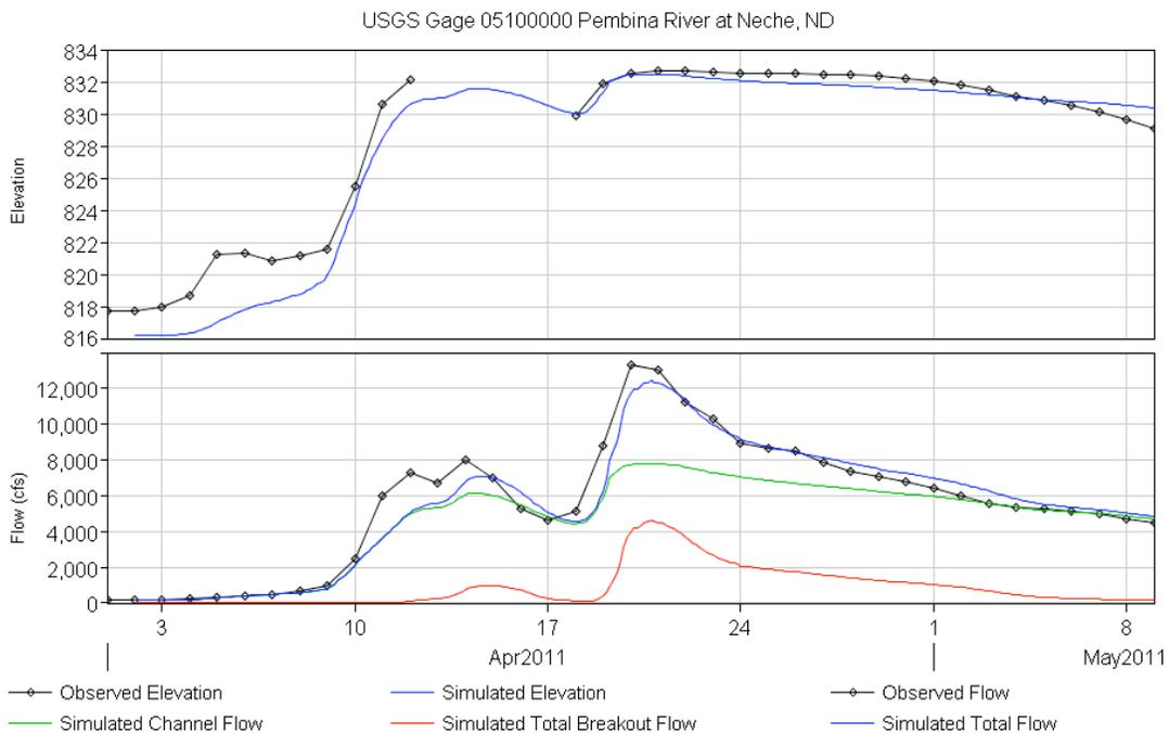
**Figure 11:** 2011 flood event simulated and observed stage and flow at USGS gage 05100000 Pembina River at Neche, ND.
