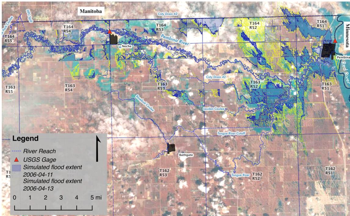
**Figure 7:** Simulated April 11, 2006 (blue) and April 13, 2006 (yellow) flood extents overlying an April 11, 2006 Landsat image. Landsat image courtesy of the USGS.
