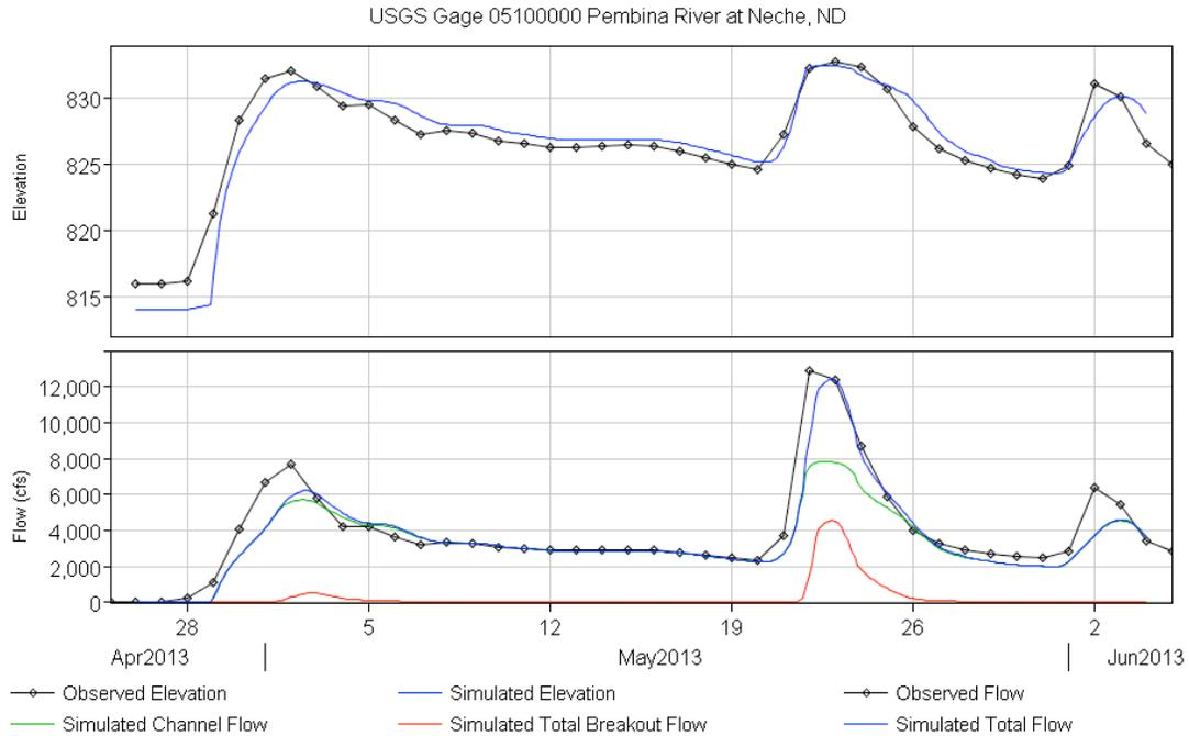
**Figure 13:** 2013 flood event simulated and observed stage and flow at USGS gage 05100000 Pembina River at Neche, ND.
