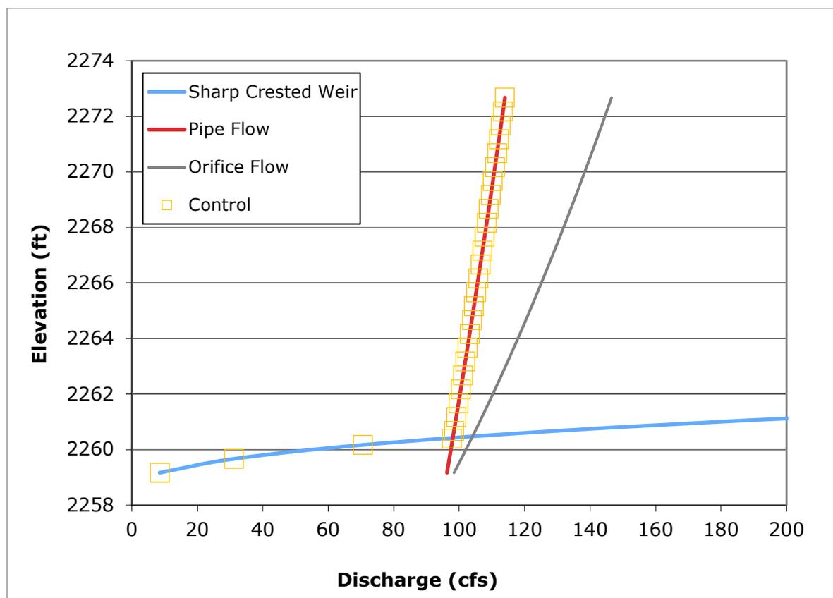
Figure 5. Principal Spillway Rating Curve
