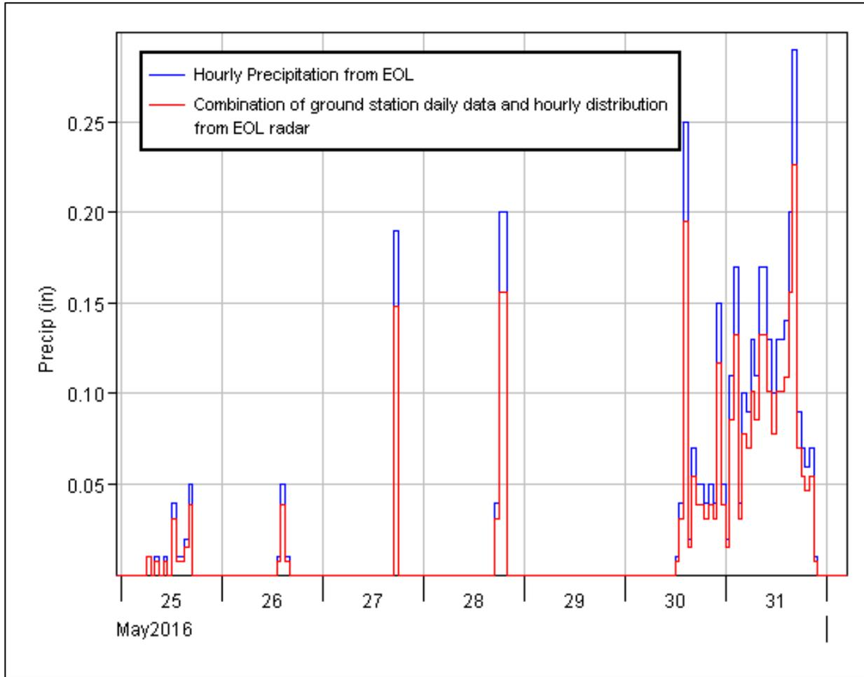
**Figure 3.** Hourly precipitation generated from the combination of ground station daily data and hourly distribution from radar (red line), and hourly precipitation from EOL (blue line).
