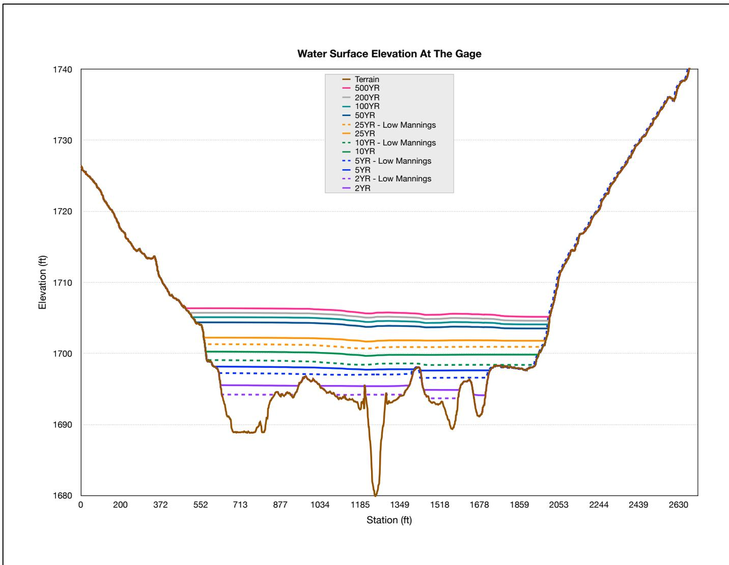
**Figure 17.** Frequency Events Maximum Water Surface Elevation at The USGS Stream Gage.
