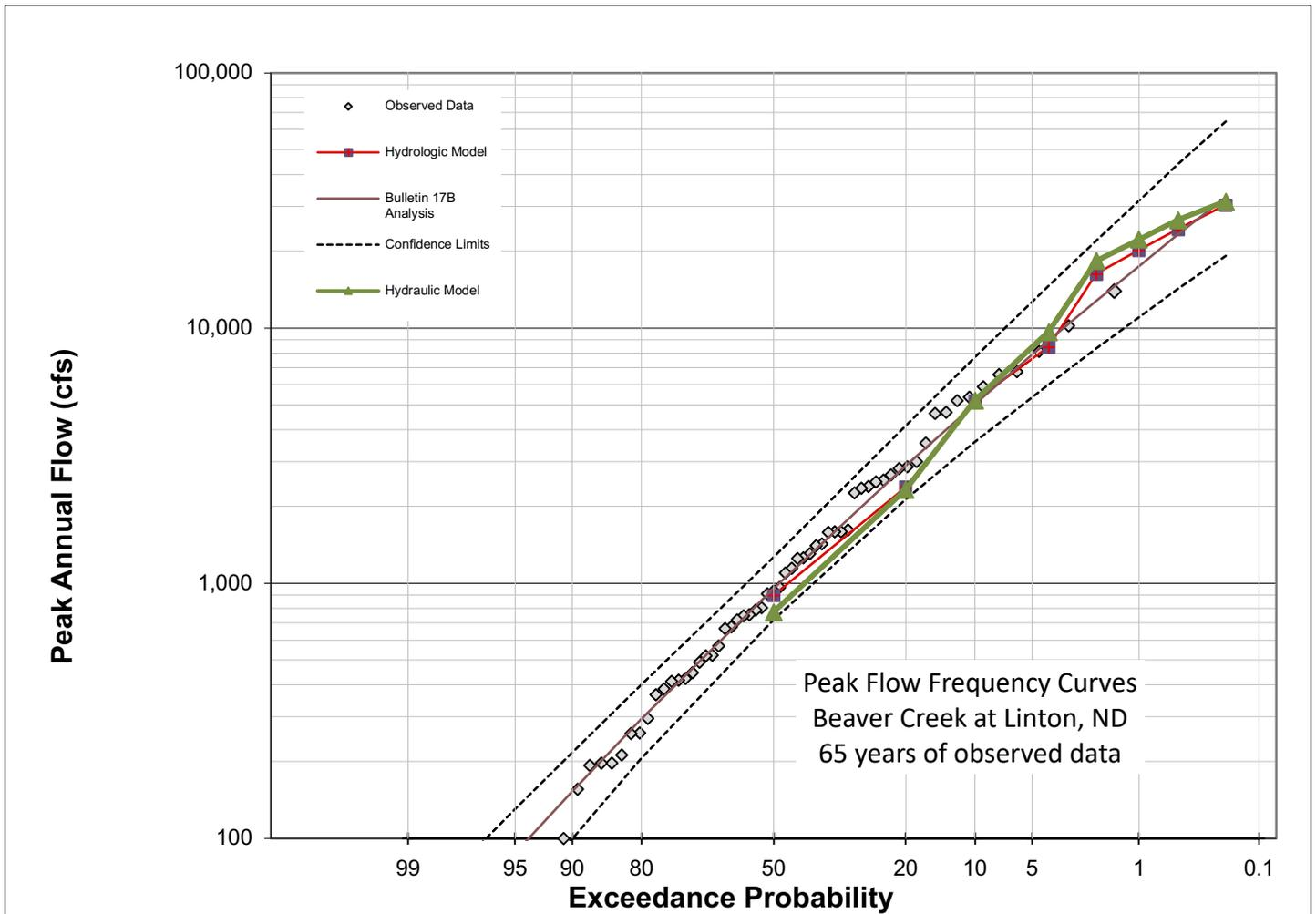
**Figure 16.** Frequency Event Peak Flow Comparison at USGS Stream Gage.
