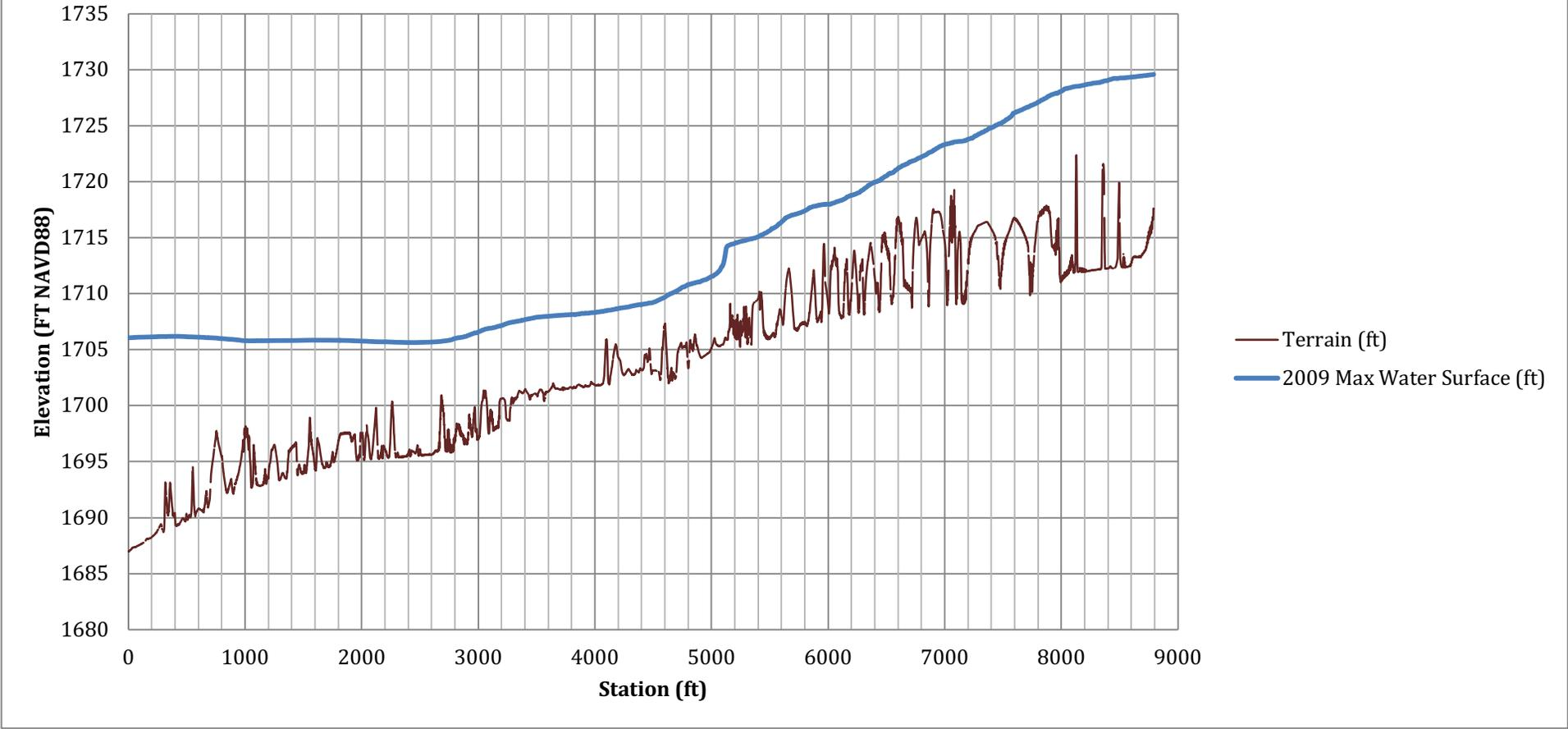
Figure 10. 2009 Max Water Surface Profile - Spring Creek.
