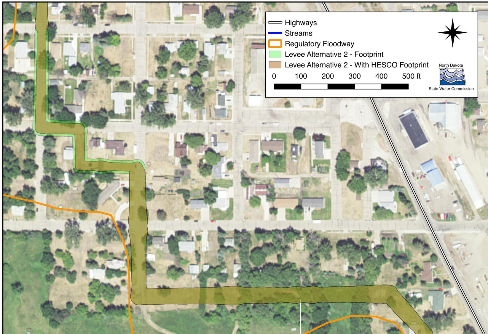
Figure 23. Temporary Emergency Levee Alternative 2 footprint - Map 2
