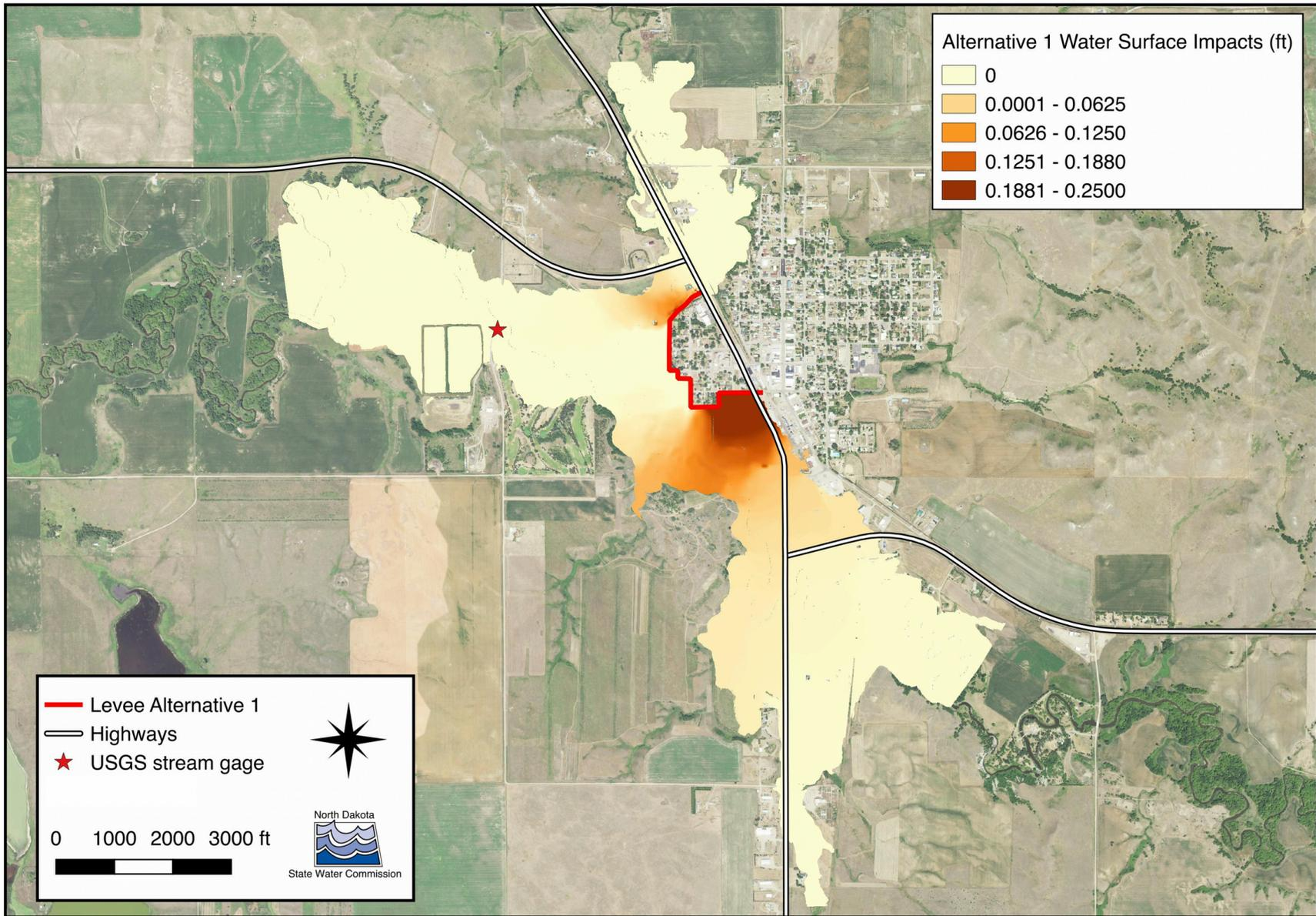
**Figure 19.** Temporary Emergency Levee Alternative 1 Water Surface Impacts
