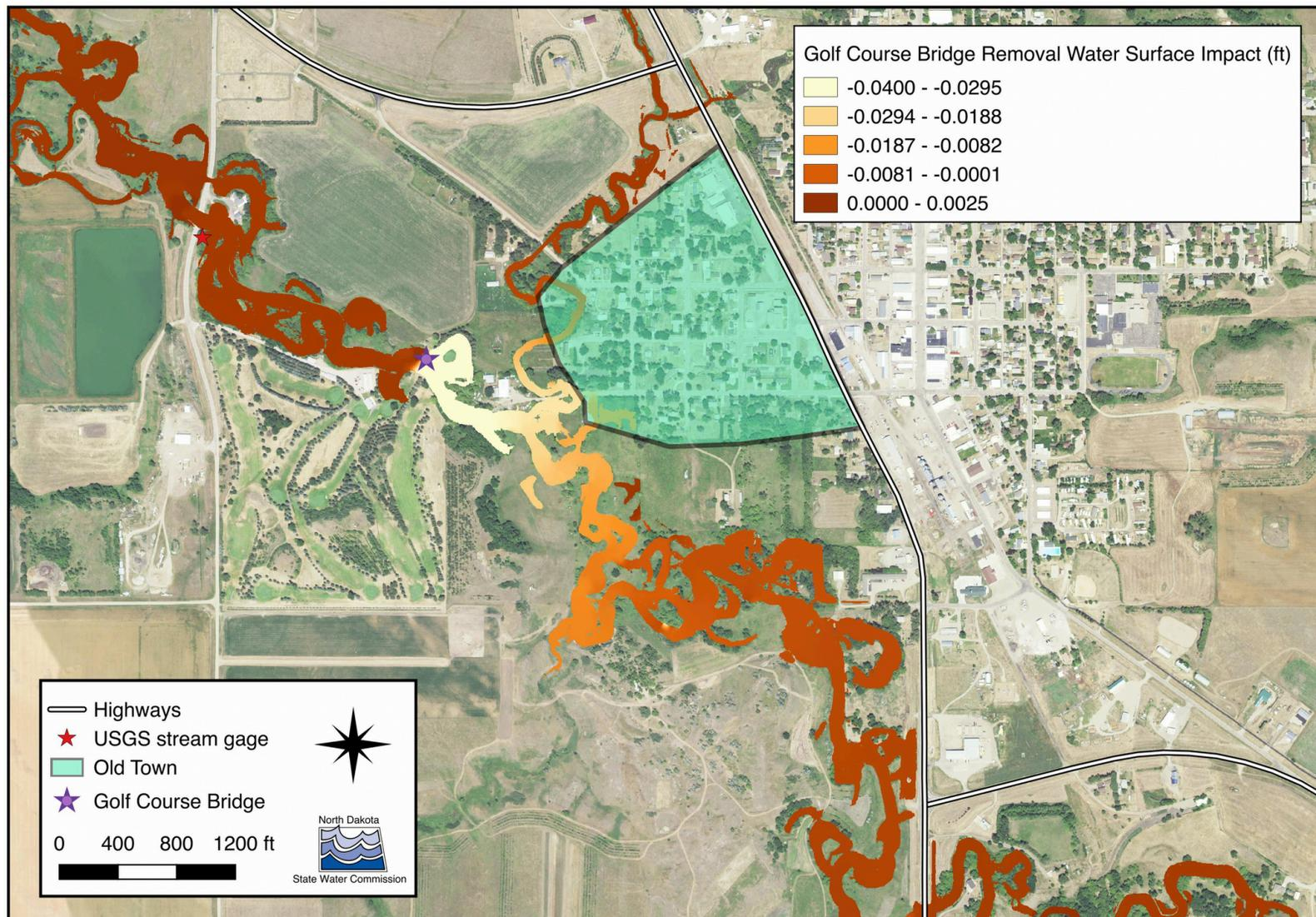
**Figure 9.** Maximum water surface difference for the 2-year frequency event between the Golf Course Bridge removal and existing conditions.
