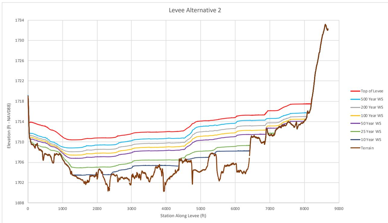
**Figure 28.** Water surface profiles along Temporary Emergency Levee Alternative 2
