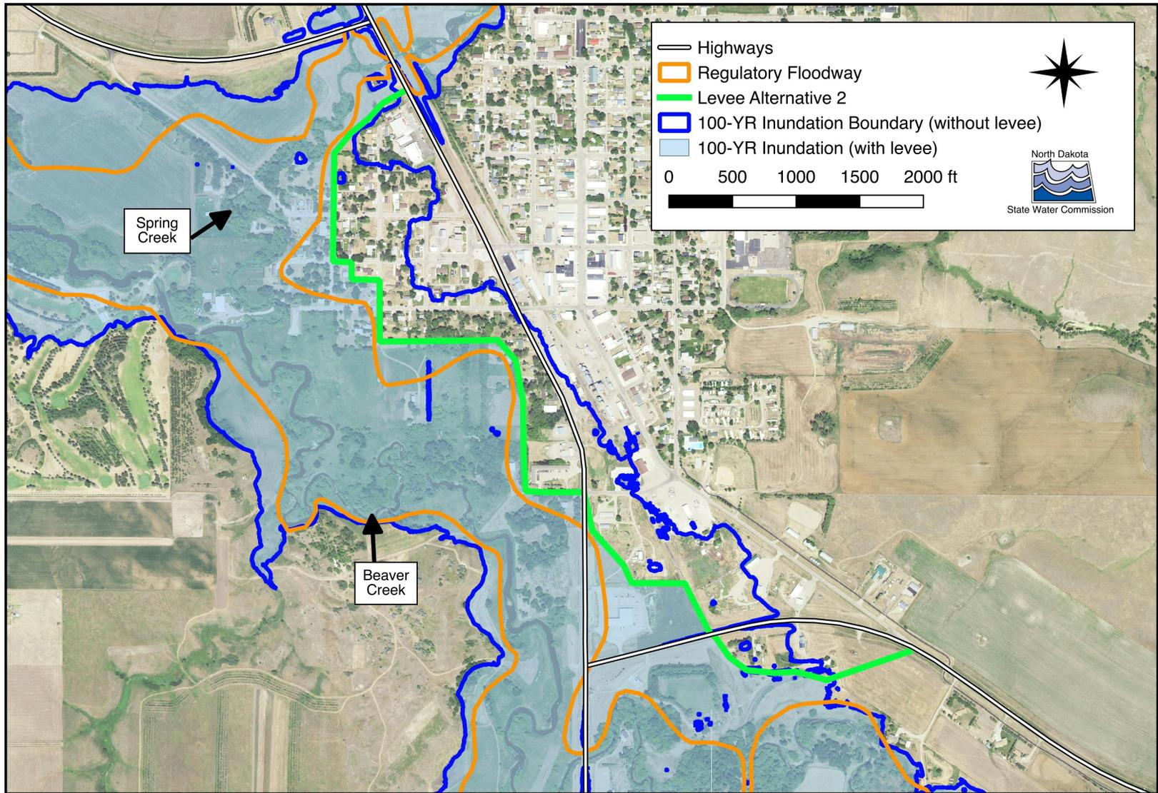
**Figure 21.** 100-year inundation area for Temporary Emergency Levee Alternative 2
