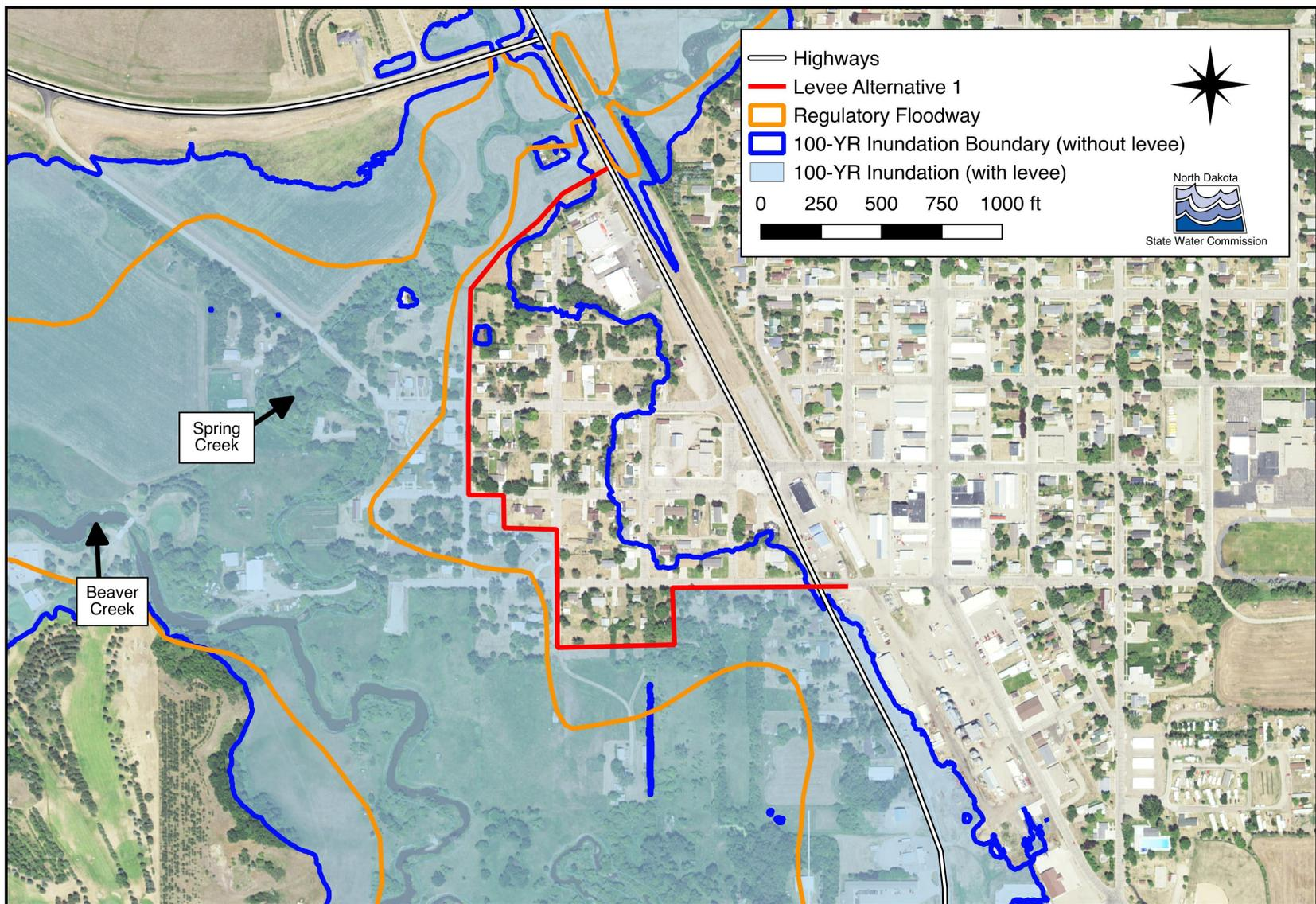
Figure 16. 100-year inundation area for Temporary Emergency Levee Alternative 1
