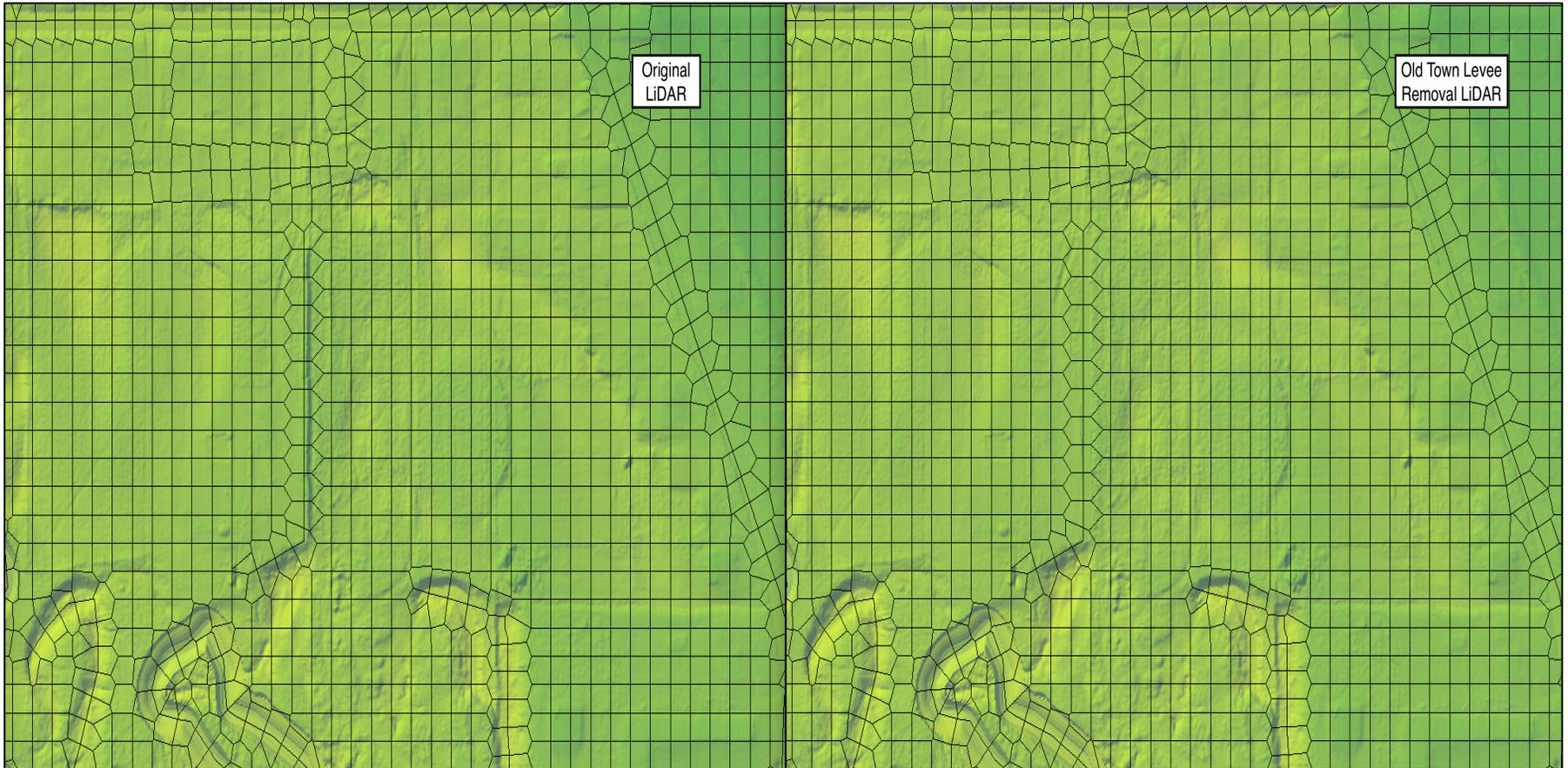
**Figure 12.** LiDAR comparison for Old Town Levee removal
