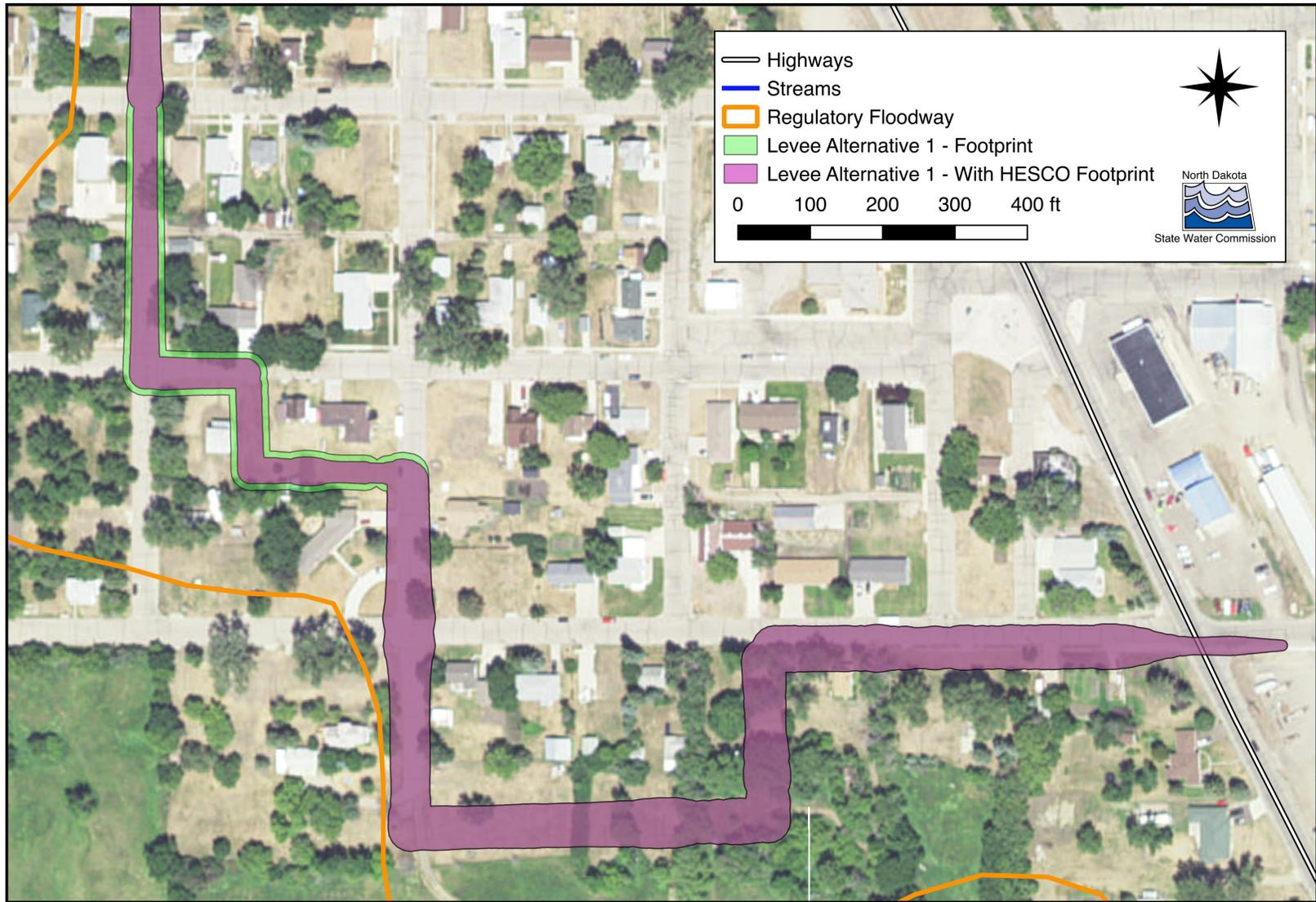
Figure 18. Temporary Emergency Levee Alternative 1 footprint - Map 2
