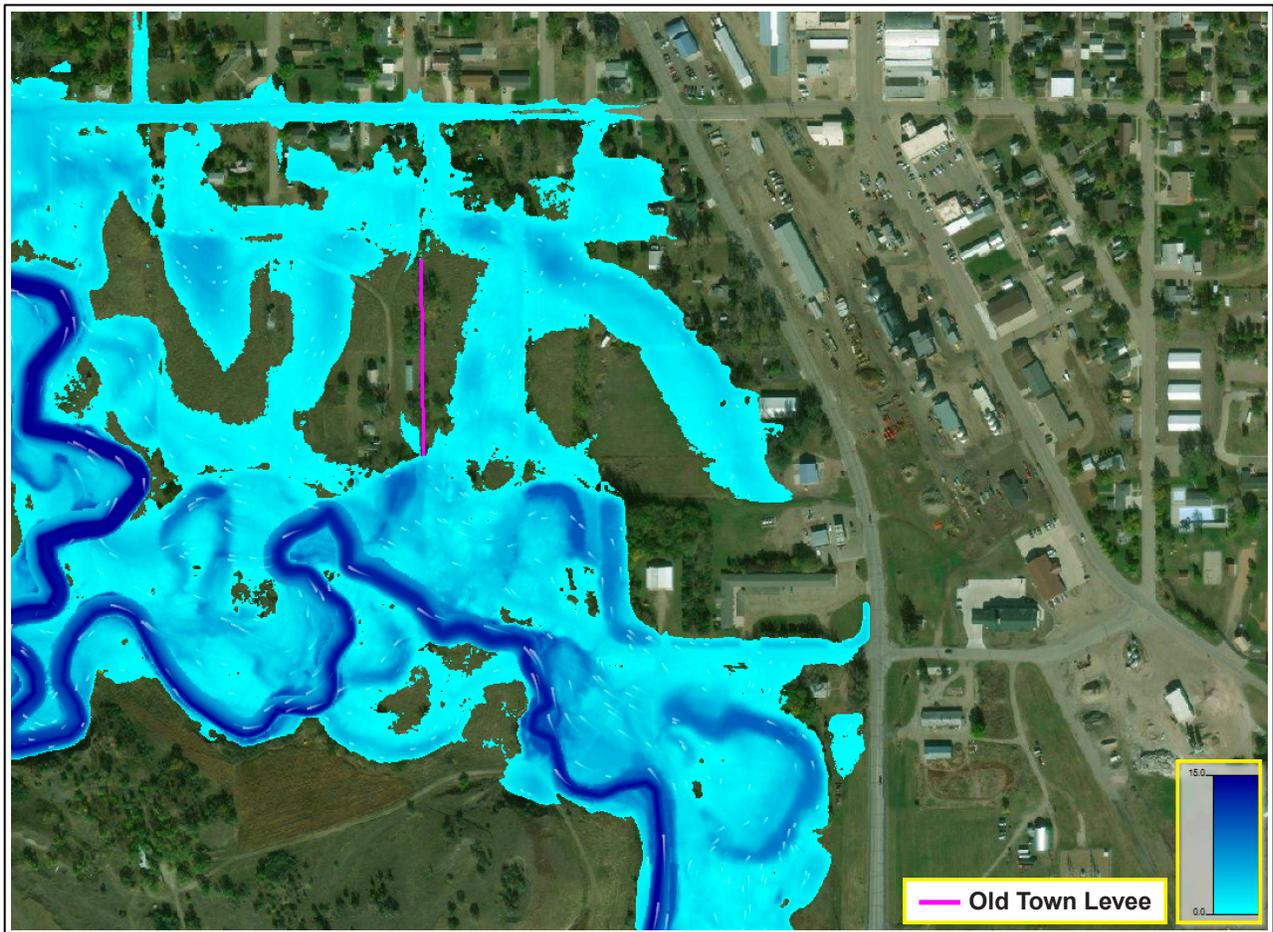
**Figure 13.** Old Town Levee lower flow path
