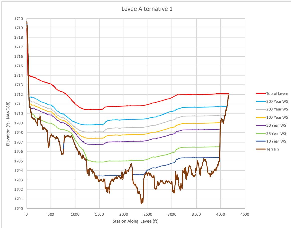
**Figure 20.** Water surface profiles along Temporary Emergency Levee Alternative 1
