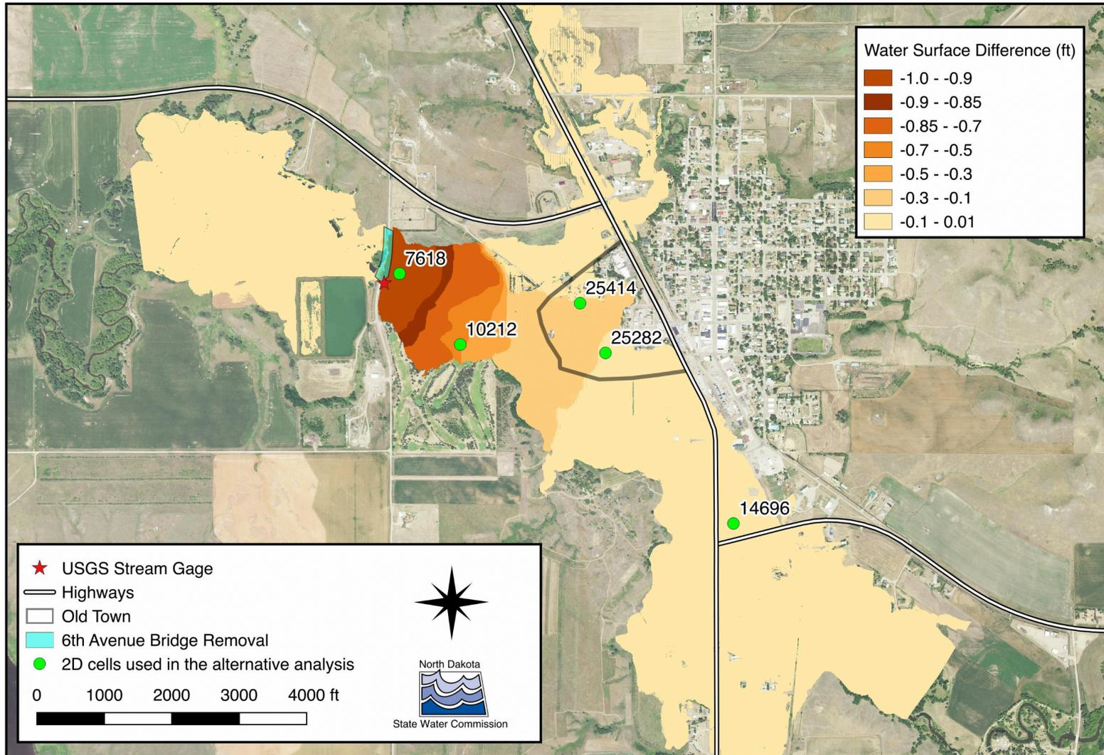
**Figure 6.** Maximum water surface difference at peak flow for the 2009 snowmelt event between existing conditions and removal of the 6th Avenue SE Bridge
