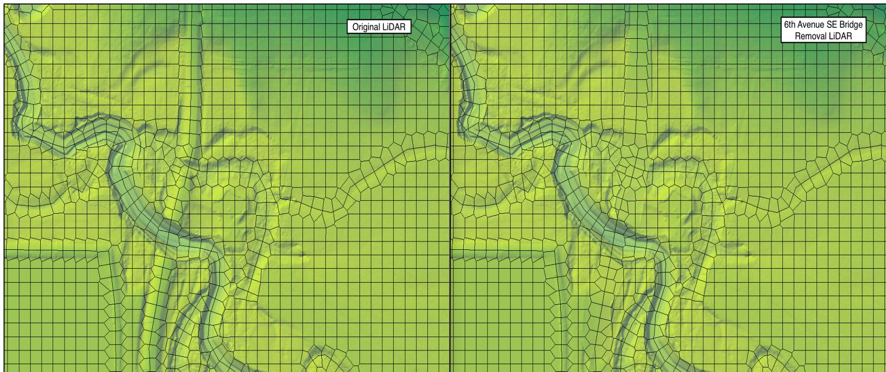
**Figure 5.** LiDAR comparison for the 6<sup>th</sup> Avenue SE Bridge removal
