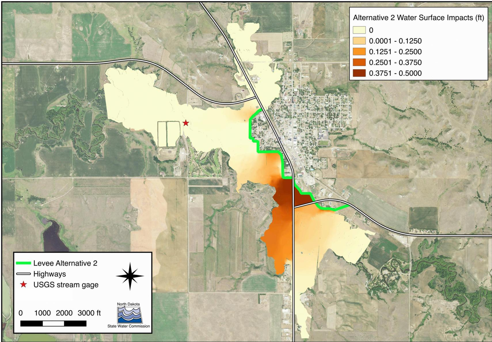
**Figure 27.** Temporary Emergency Levee Alternative 2 Water Surface Impacts
