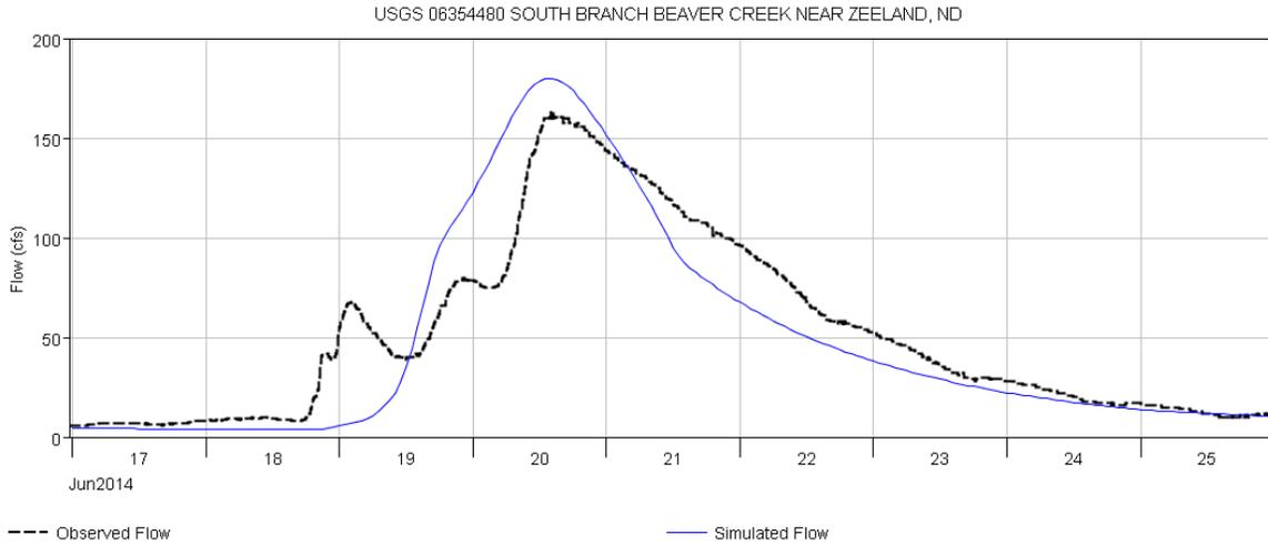
**Figure 13:** Observed and modeled discharges at USGS gage 06354480 near Zeeland for the 2014 rainfall event.
