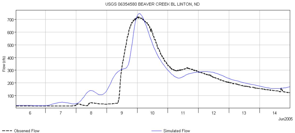
**Figure 6:** Observed and modeled discharges at USGS gage 06354580 below Linton for the 2005 rainfall event.
