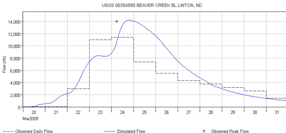
**Figure 16:** Observed and modeled discharges at USGS gage 06354580 below Linton for the 2009 snowmelt event.
