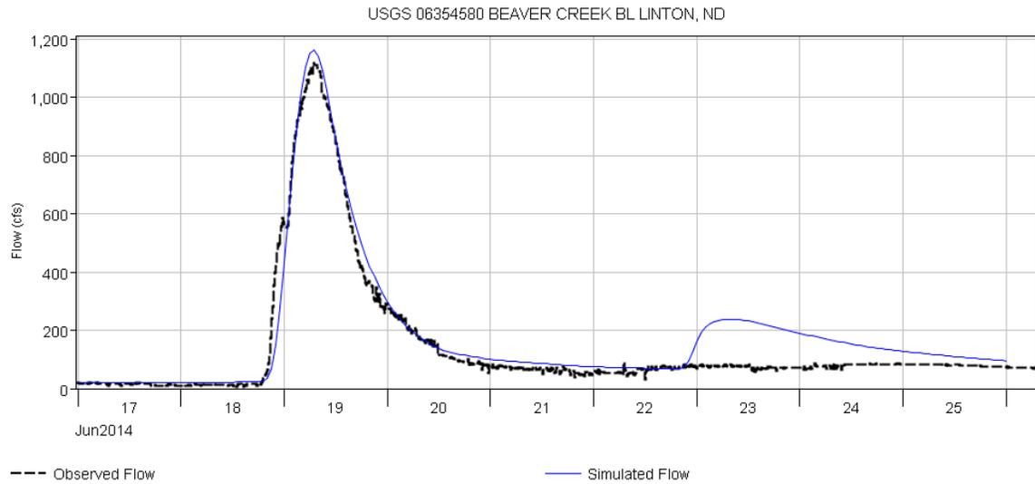
**Figure 14:** Observed and modeled discharges at USGS gage 06354580 below Linton for the 2014 rainfall event.
