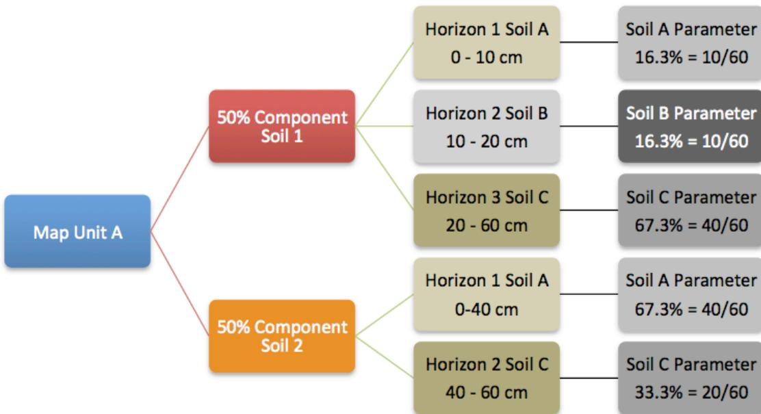
**Figure 2:** Example soil type distribution to a depth of 60 cm within a map unit.
