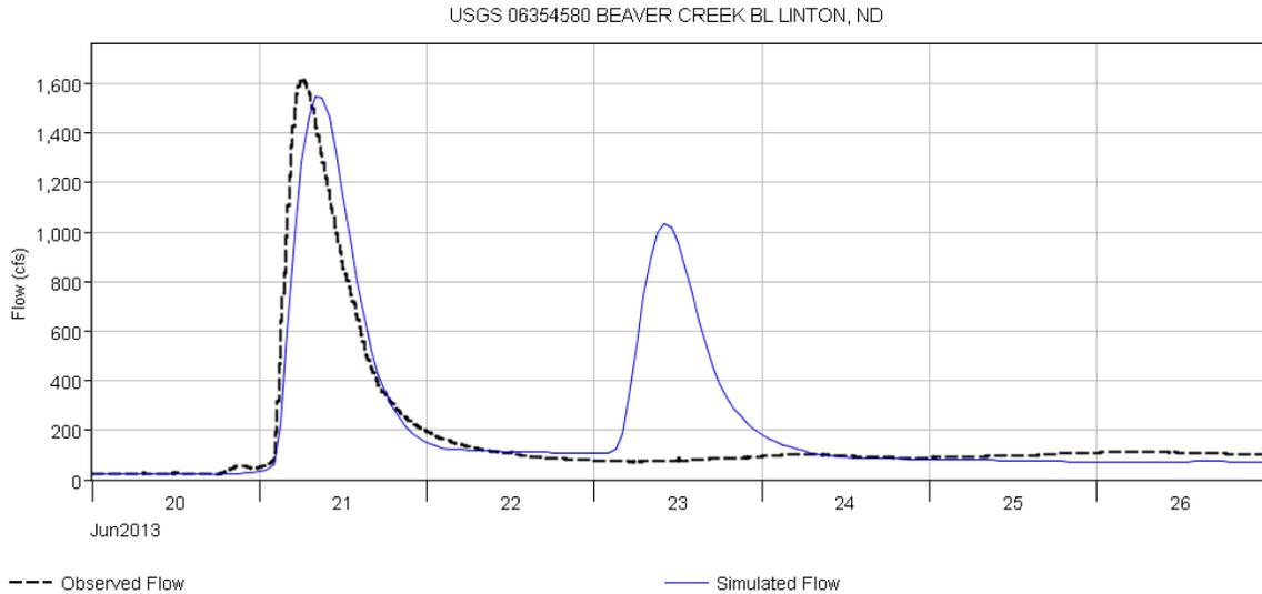
**Figure 11:** Observed and modeled discharges at USGS gage 06354580 below Linton for the 2013 rainfall event.
