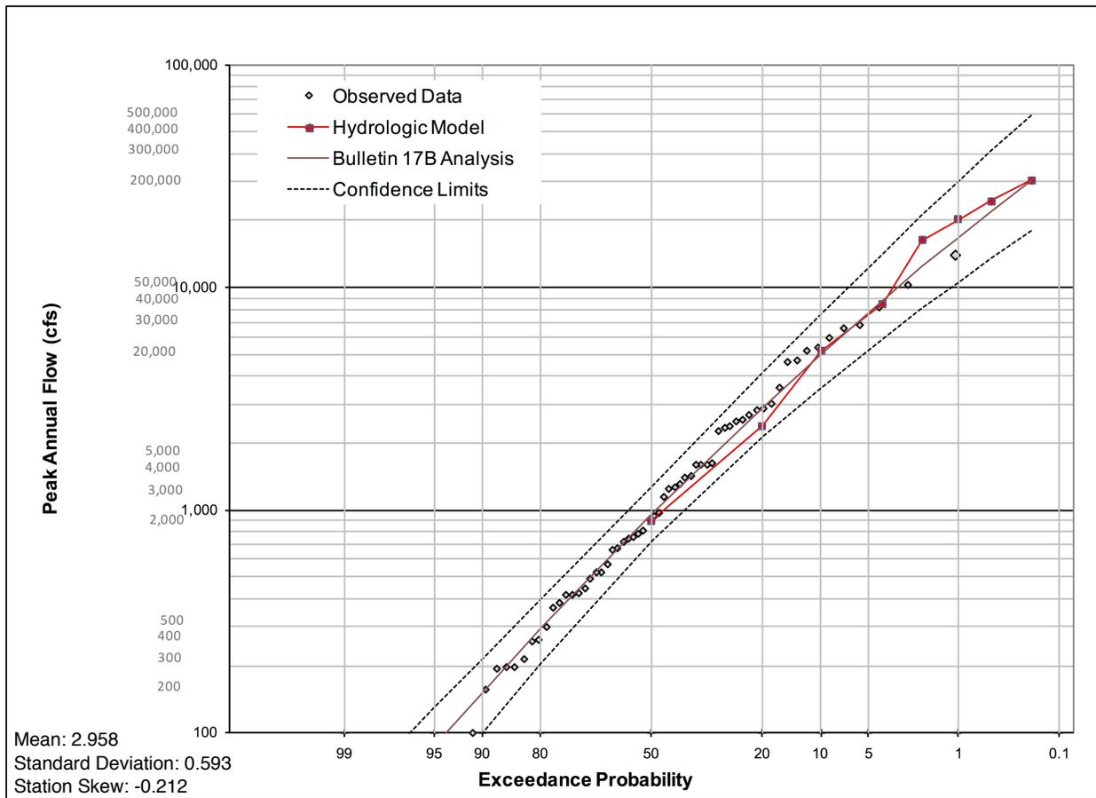
**Figure 17:** Annual peak flow frequency curve for USGS Gages 06354500 at Linton and 06354580 below Linton (1950 – 2013).
