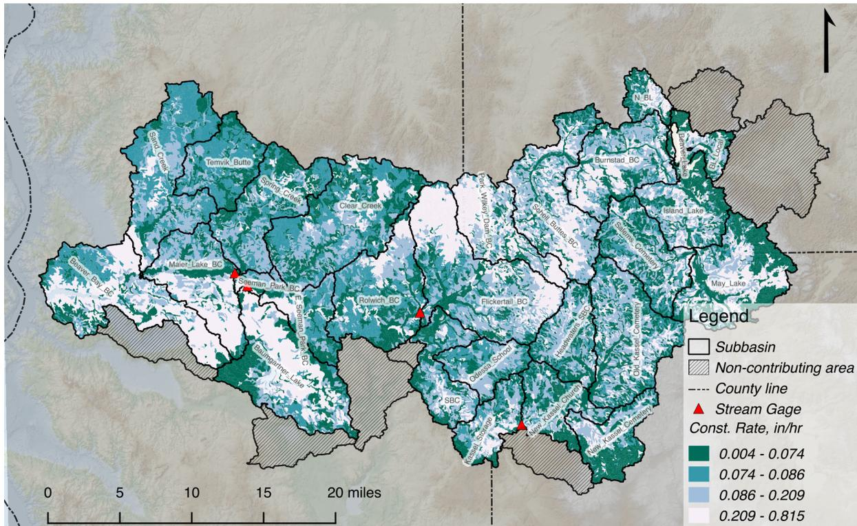
**Figure 3:** Constant infiltration rate distribution.
