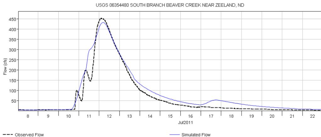
**Figure 8:** Observed and modeled discharges at USGS gage 06354480 near Zeeland for the 2011 rainfall event.
