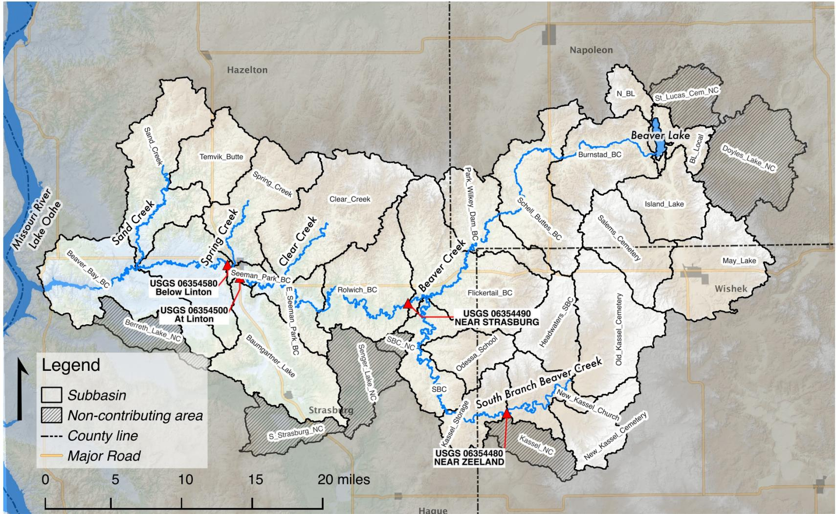
Figure 2: Beaver Creek subbasins and stream gages.
