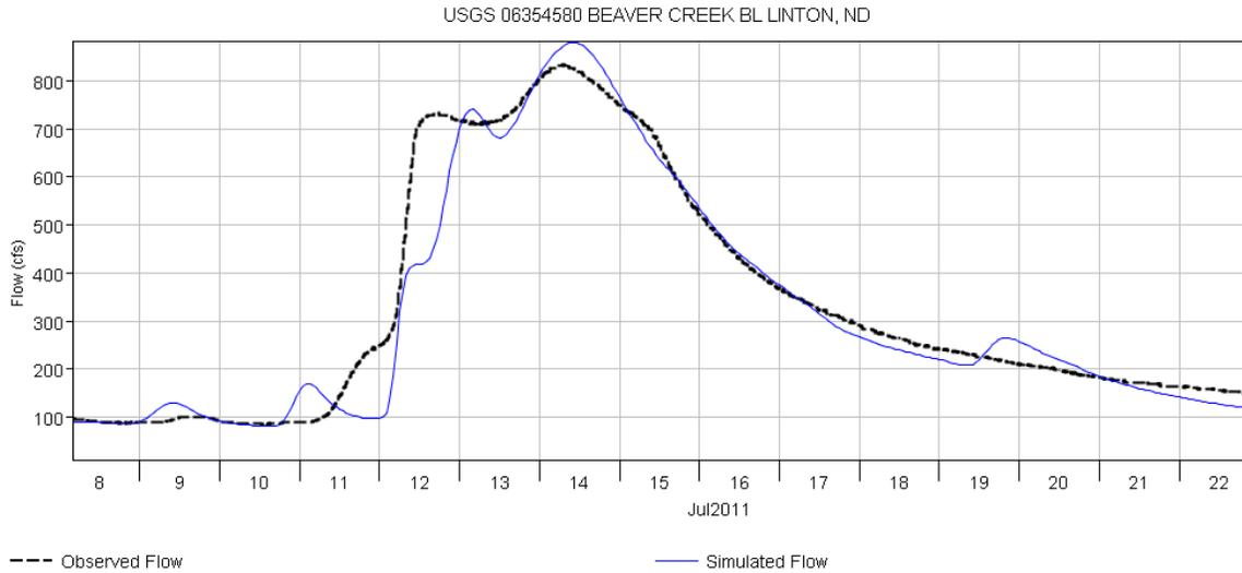
**Figure 9:** Observed and modeled discharges at USGS gage 06354580 below Linton for the 2011 rainfall event.
