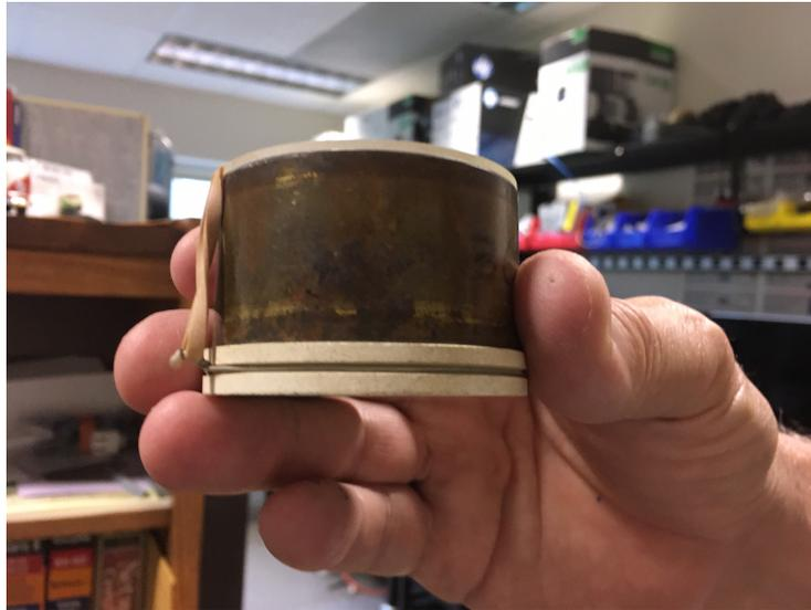
Figure. 4. Sample-plate assembly used for measurement of soil water-retention curves.
