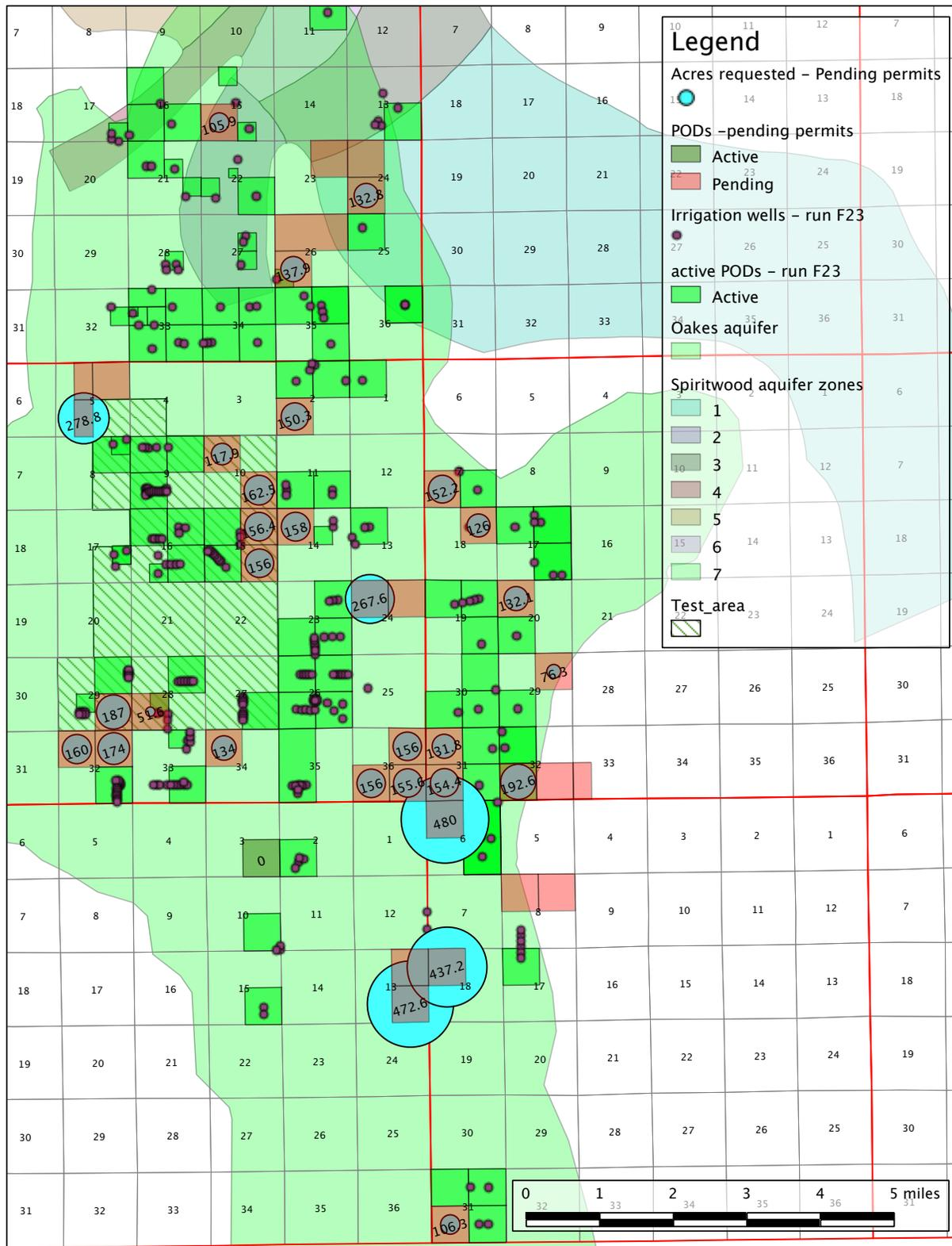
**Figure 11.** Location of active and pending PODs for Oakes and underlying Spiritwood aquifers. The diameter of the circles show acres requested in pending water permit applications and are labeled with the pending acres. The size of the circle is proportional to the acres requested.
