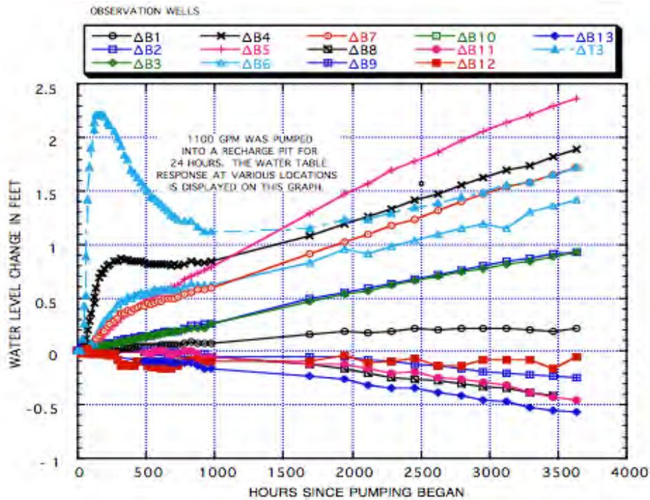
Figure 15. Changes in water levels in monitoring wells following the 24-hour pilot test on the south (triangular) basin in the fall of 1992.
