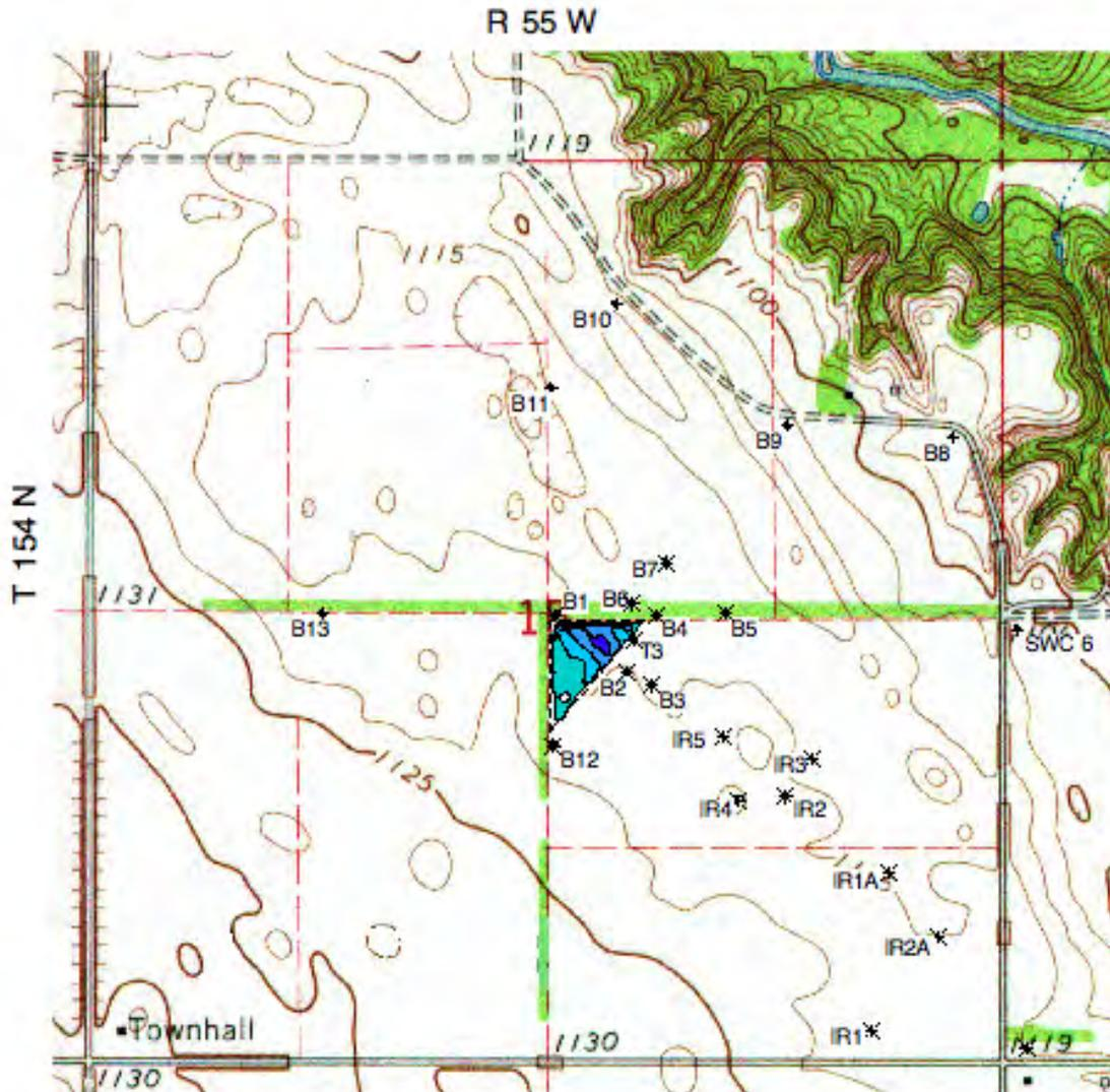
Figure 6. Pilot basin site in the center of Section 154-055-15. Wells labeled “IR” are the locations of irrigation wells before basin construction. Sites labeled “B” are observation wells placed to monitor water levels affected by ARR.
