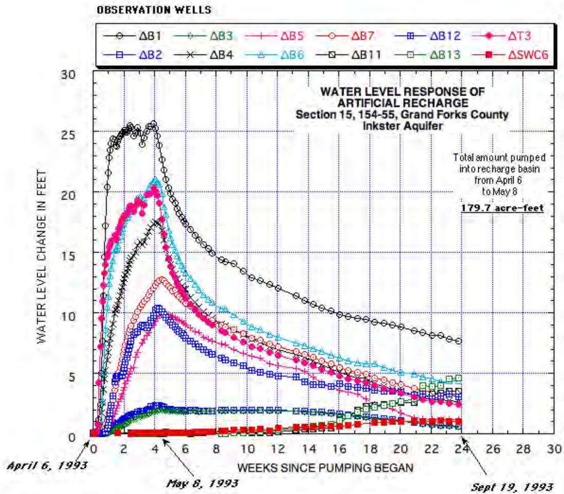
Figure 16. Changes in water levels in monitoring wells following the 24-hour pilot test on the south (triangular) basin in the spring of 1993. Basin operation was initiated on April 6, and terminated on May 8.
