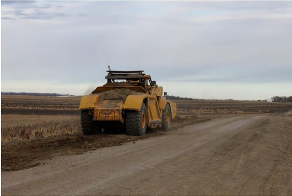
Figure B-3. John Deere JP686™ self-loading scraper depositing the filter-cake residue collected from the basin floor on the outside of the basin berm.
