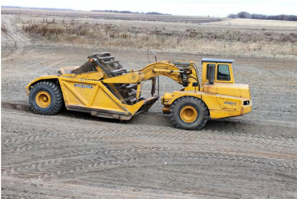
Figure B-2. John Deere JP686<sup>TM</sup> self-loading scraper, used to collect the filter-cake pile deposited by the grader.
