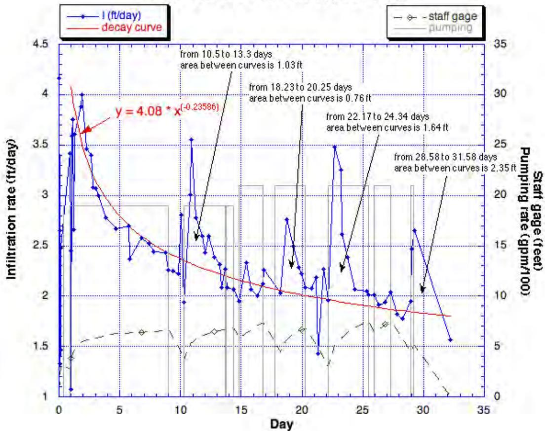
Figure 12. Infiltration during the spring 1993 pilot operation on ARR Basin 1 (the triangular south basin).
