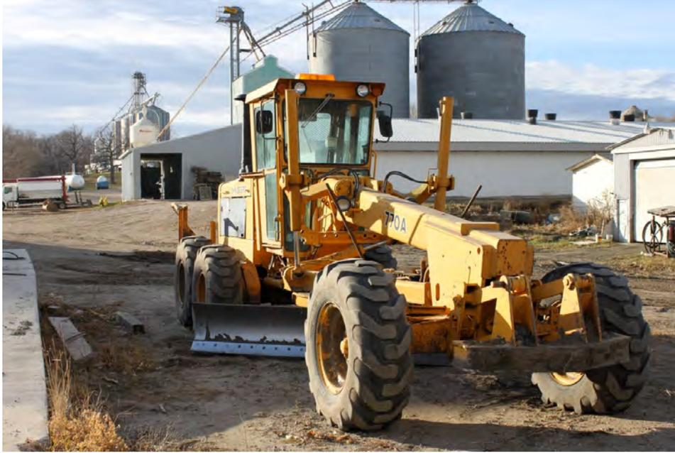
Figure B-1. John Deere 770<sup>TM</sup> grader used to “peel” filter cake. The grading operation begins on two edges of the basin, and the filter cake is scraped toward the center, where a single pile is collected for removal.
