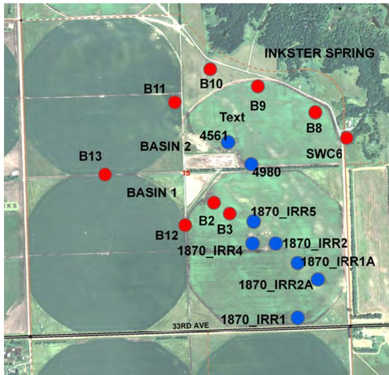
Figure 17. Location of the Forest-River Community ARR basin(s) in the center of 154-055-15, with irrigation wells (blue) and monitoring wells (red).
