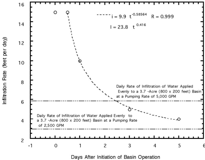
Figure 8. Infiltration rates at which the recharge mound underlying the recharge basin will intersect the basin surface (at 30 feet above the water table) after a specified number of days of operation during the fall 1992 pilot test.
