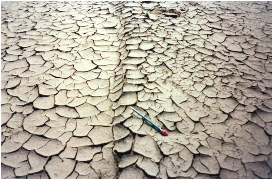
Figure 14. Surface sediment filter cake: (A) immediately after operation of the rectangular (2nd) basin, and (B) after desiccation of the basin floor.
