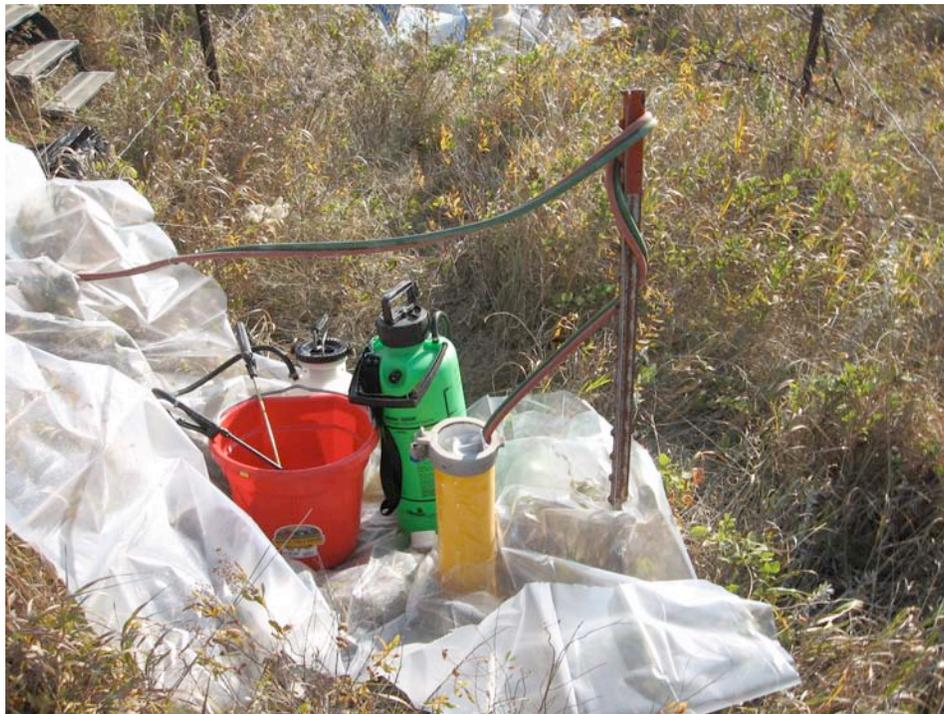
Photo 4. Purging a well using a gas squeeze pump.
