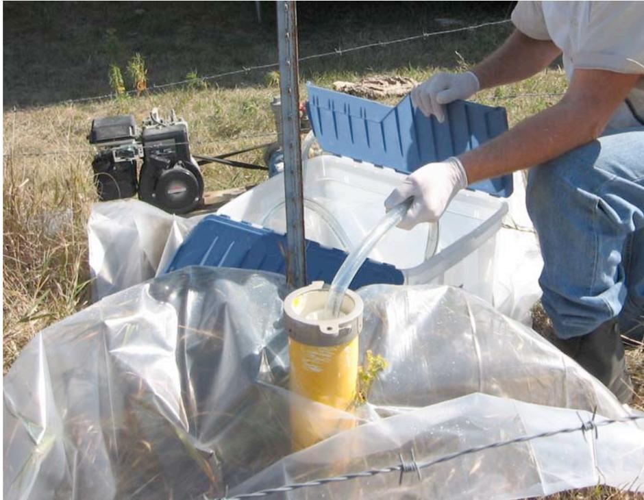
Photo 3. Purging a well by suction lift using a screw pump.
