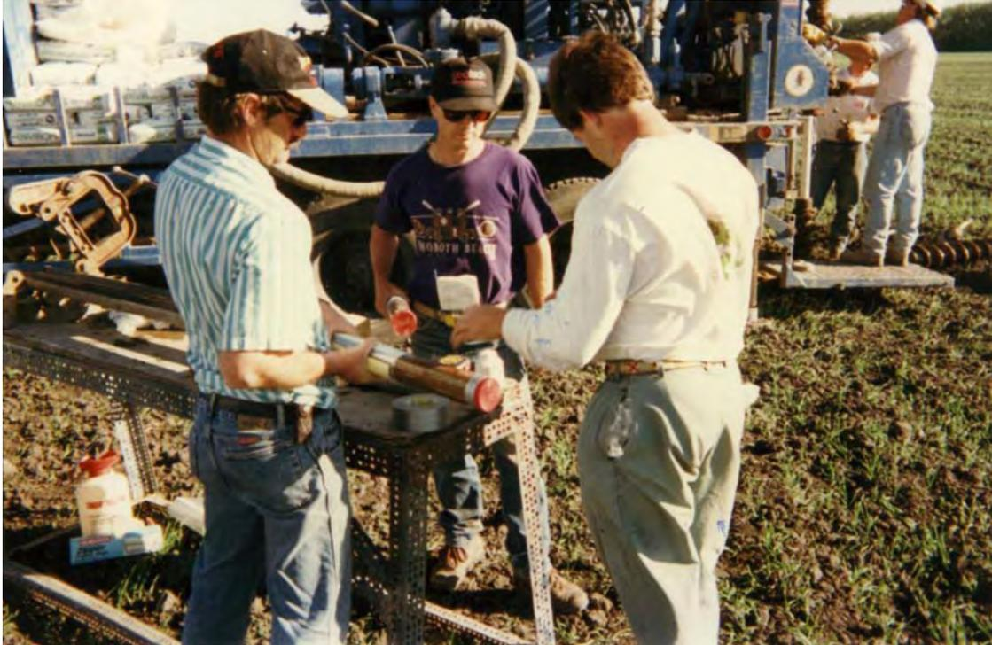
Field processing of acetate-lined sediment samples from “split-spoon” cores, obtained with a hollow-core auger from the shallow, middle, and deep Elk Valley aquifer on Sites 1 through 6 (June 1997).
