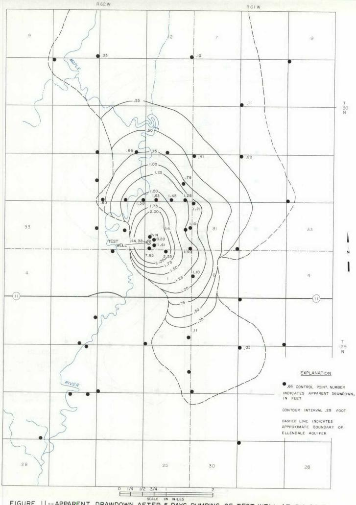
FIGURE 11 -- APPARENT DRAWDOWN AFTER 5 DAYS PUMPING OF TEST WELL AT 310 G.P.M.
