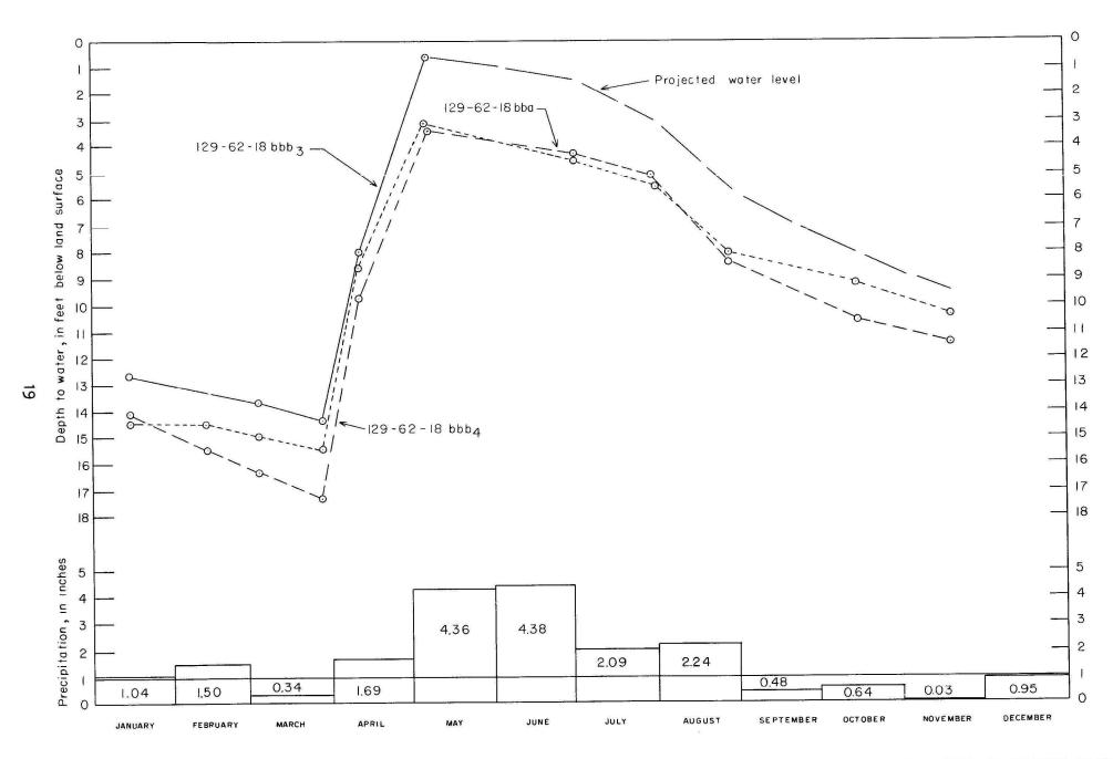
FIGURE 8 -- WATER - LEVEL FLUCTUATIONS IN DRY BRANCH OUTWASH DEPOSIT AND PRECIPITATION AT ELLENDALE DURING 1969
