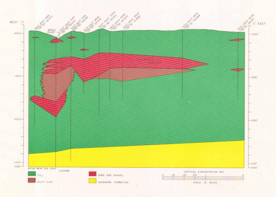
FIGURE 5 -- GEOLOGIC CROSS SECTION C-C'
