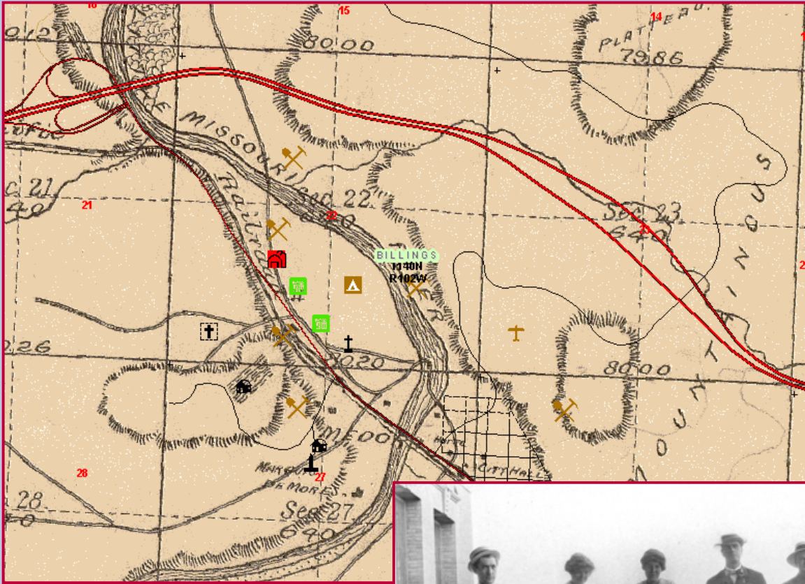
At Left: The General Land Office (GLO) plats were scanned and then geo-registered for use in the SWC enterprise GIS, so they can be overlaid with contemporary map data. This allows comparison of map features from 100 years ago, with those that we see around us today.
