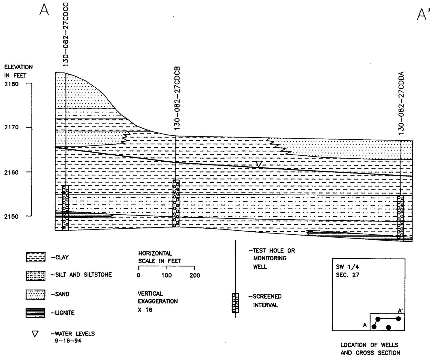
Figure 6. Geohydrologic section A-A' in the Selfridge landfill.
