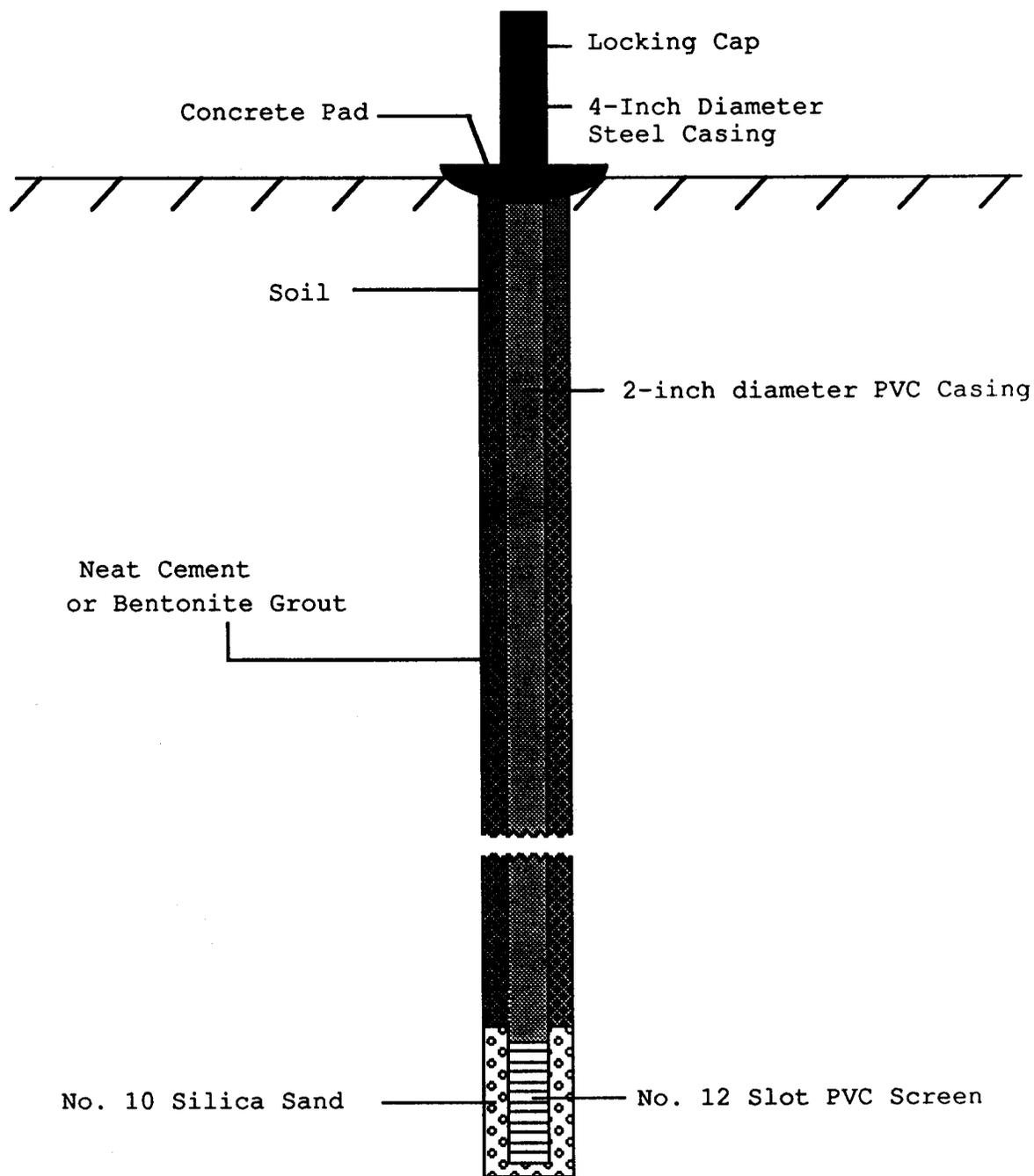
Figure 2. Construction design used for monitoring wells installed at the New Salem landfill.
