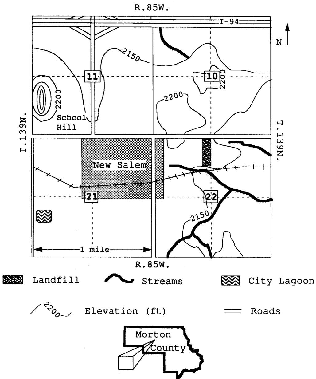
Figure 1. Location of the New Salem landfill in the NW 1/4 of section 22 T139 N. R85 W.
