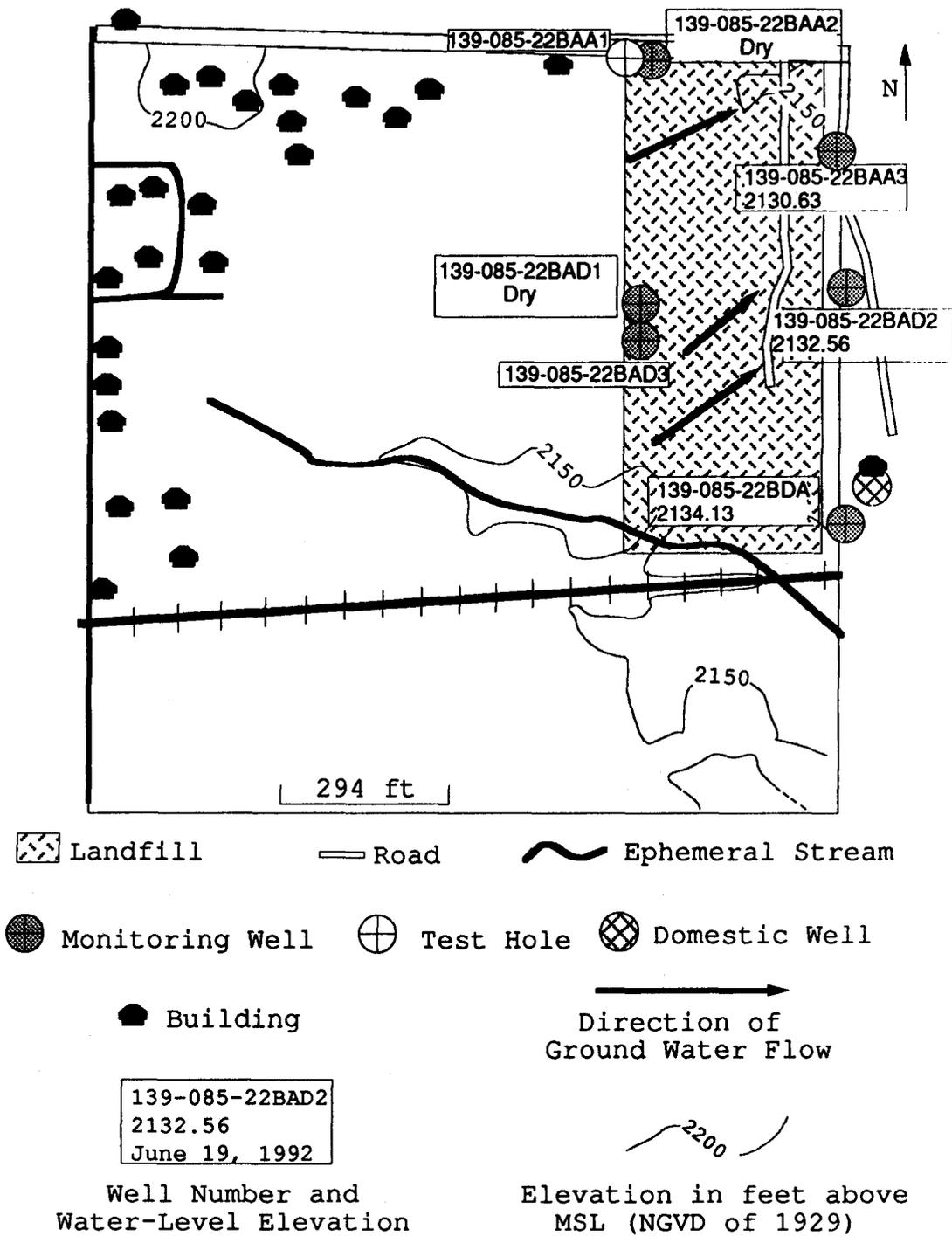
Figure 5. Location of monitoring wells and test holes at the New Salem landfill and direction of ground-water flow in the uppermost aquifer beneath the landfill.
