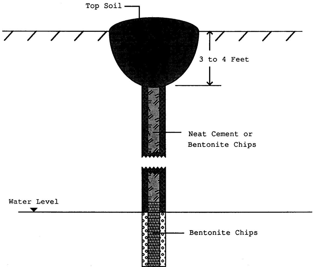
Figure 3. Monitoring well abandonment procedure.
