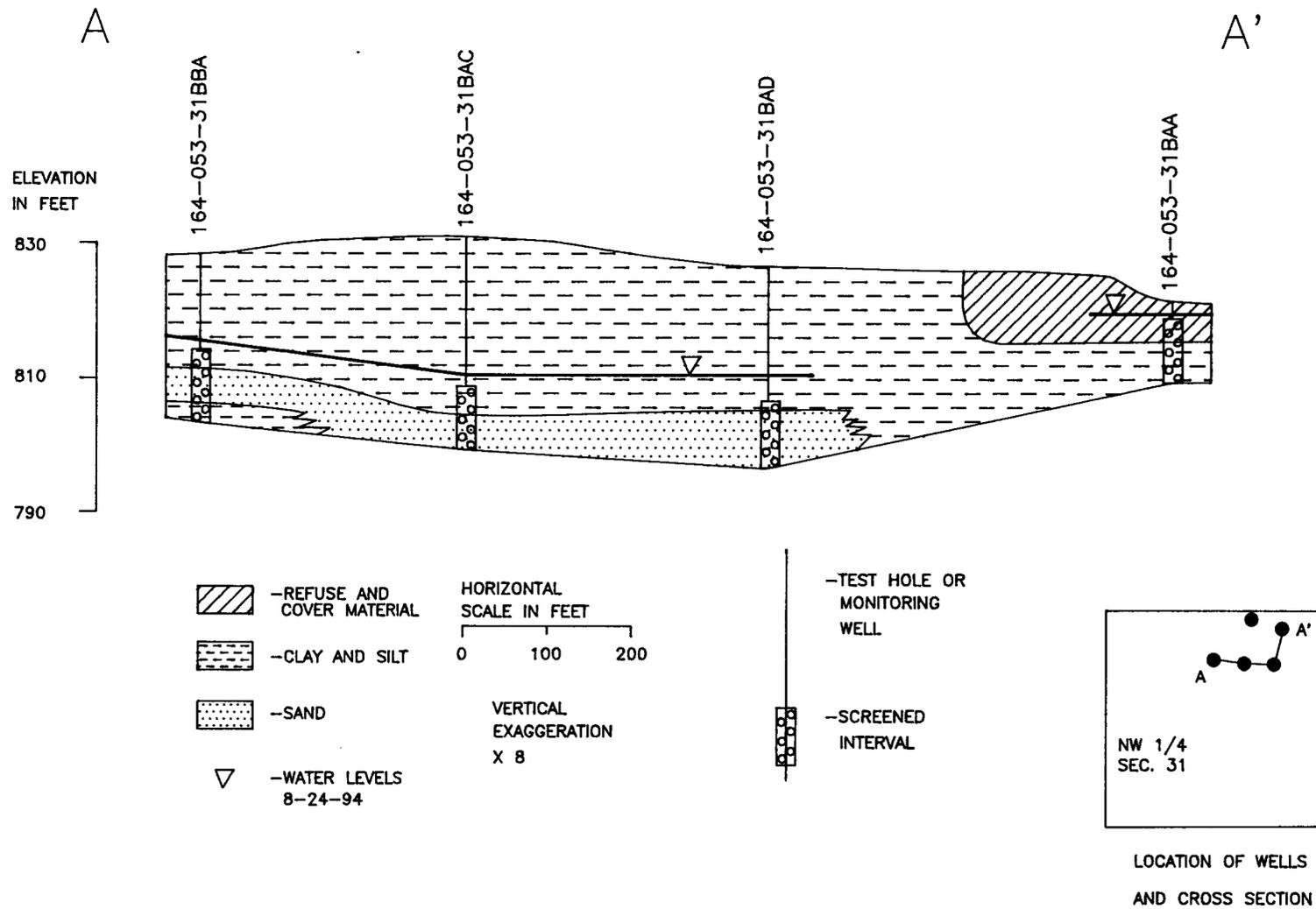
Figure 5. Geohydrologic section A-A' in the Jensen landfill.
