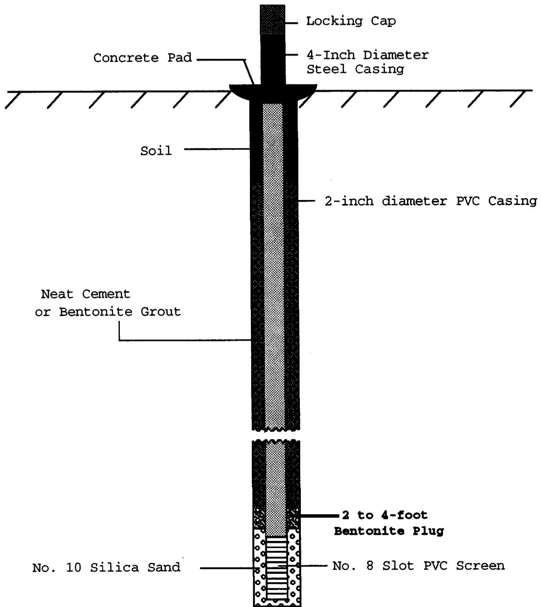
Figure 2. Construction design used for monitoring wells installed at the Jensen landfill.
