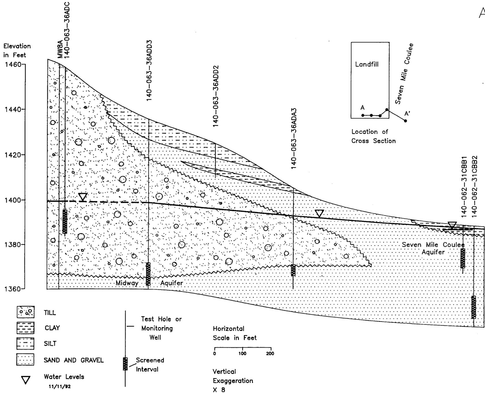
Figure 5. Geohydrologic cross section A-A' in the Jamestown landfill.
