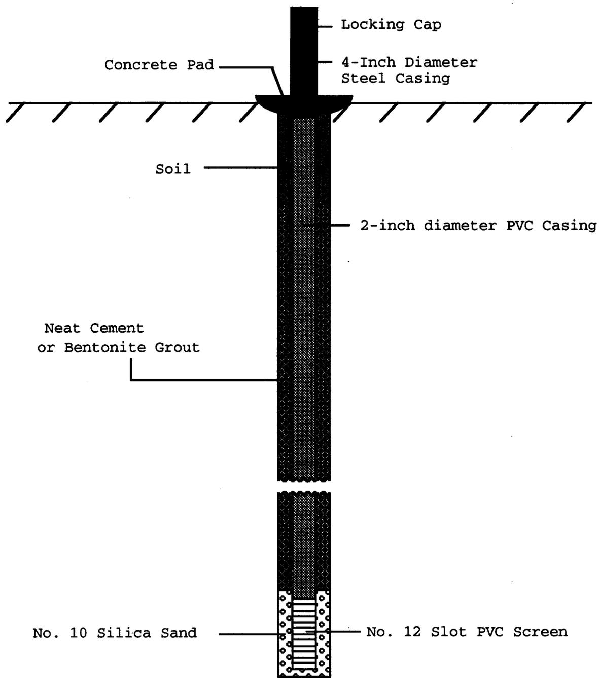
Figure 2. Construction design used for monitoring wells installed at the Jamestown landfill.
