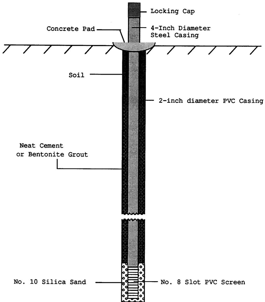
Figure 2. Construction design used for monitoring wells installed at the Geving landfill.
