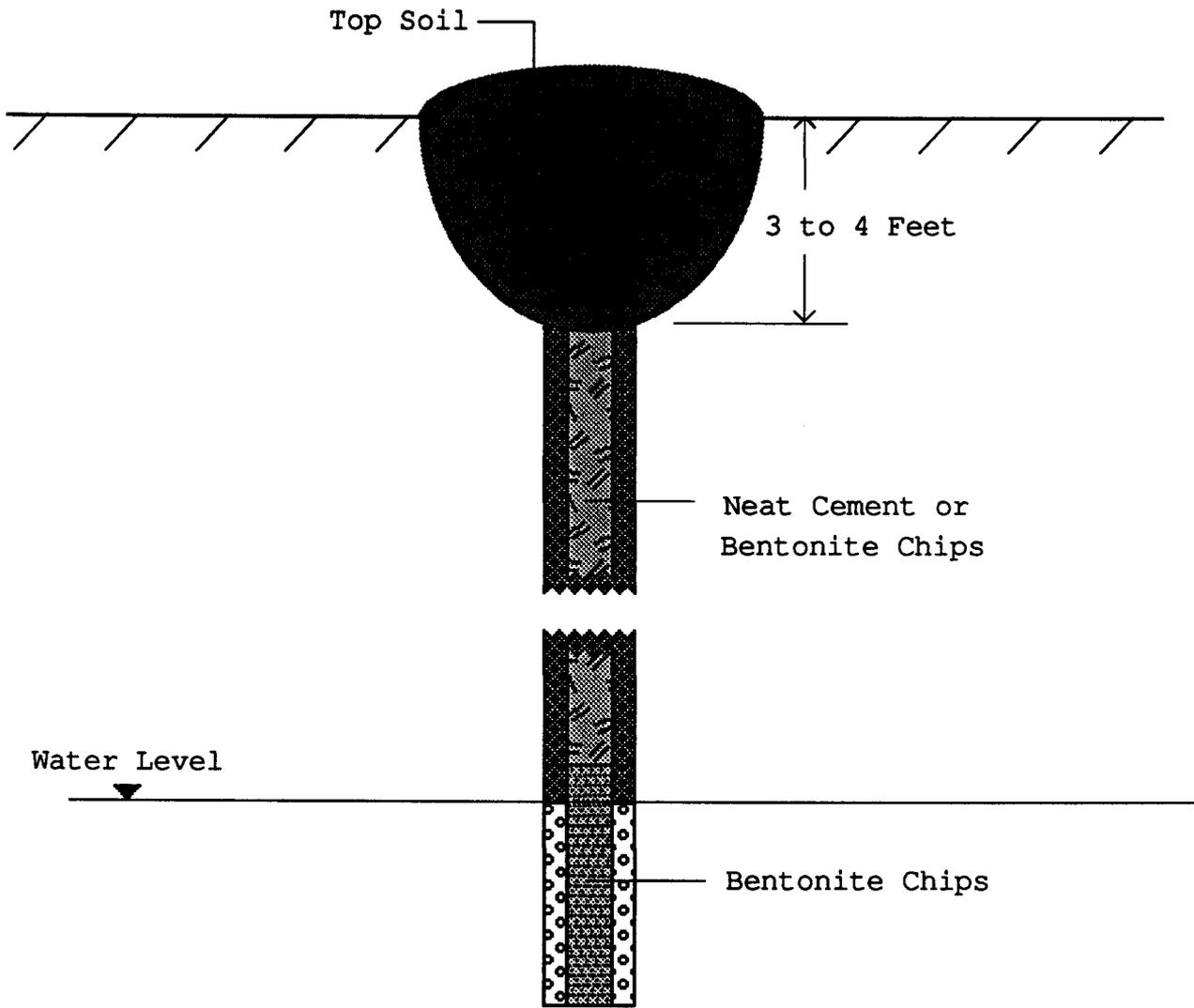
Figure 3. Monitoring well abandonment procedures.
