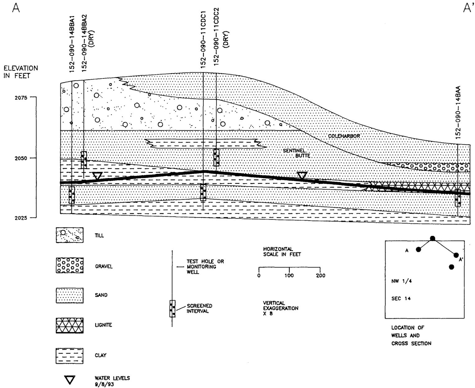
Figure 6. Geohydrologic section A-A' in the Geving landfill.
