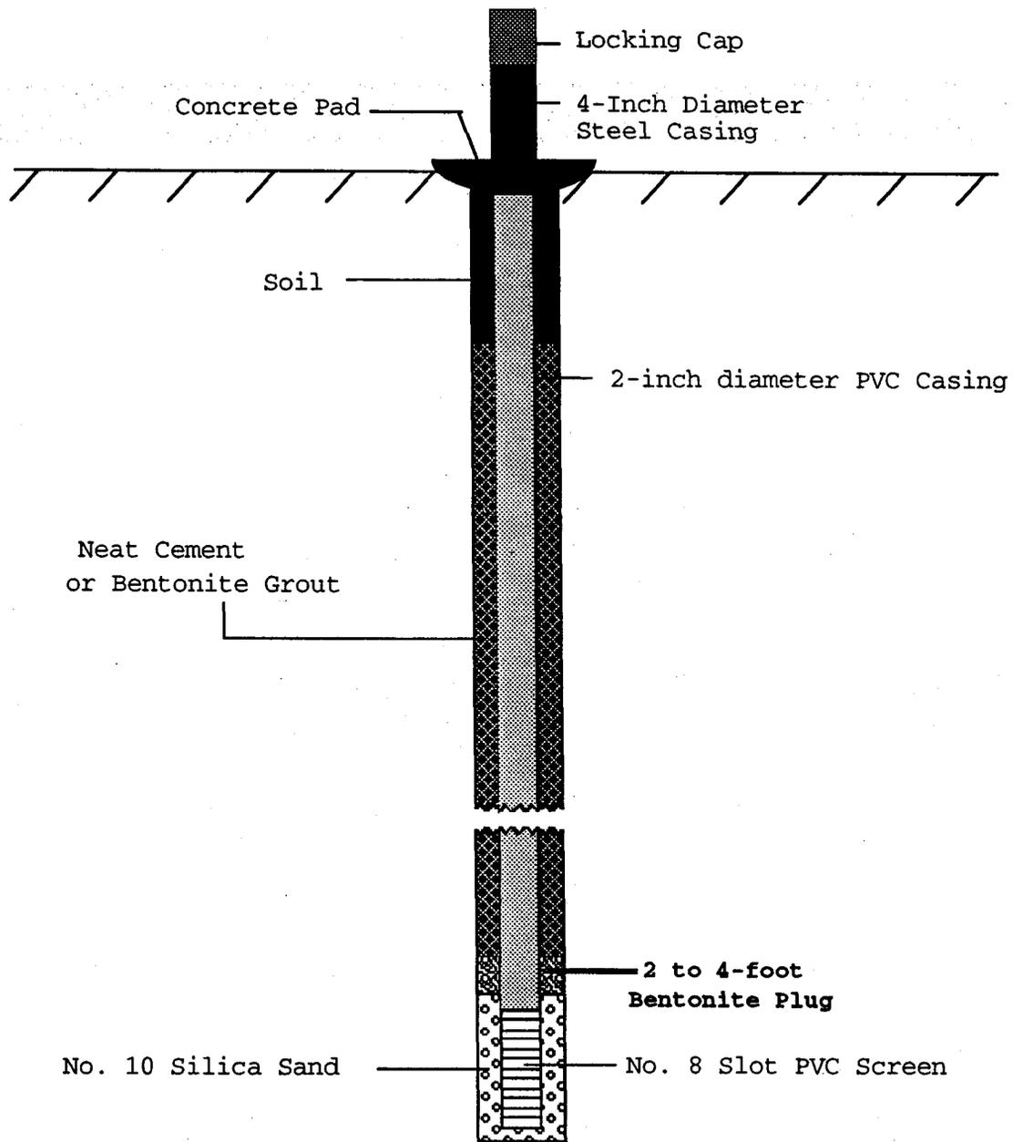
Figure 2. Construction design used for monitoring wells installed at the Fargo landfill.
