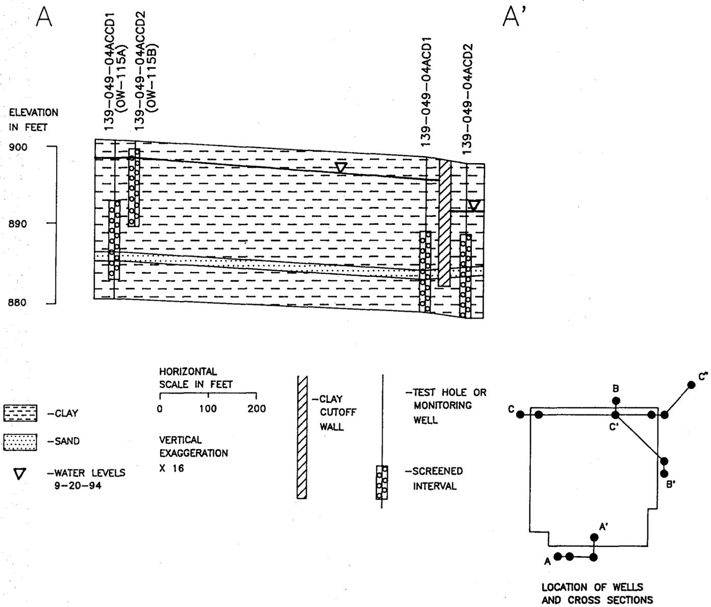
Figure 5. Geohydrologic section A-A' in the Fargo landfill.
