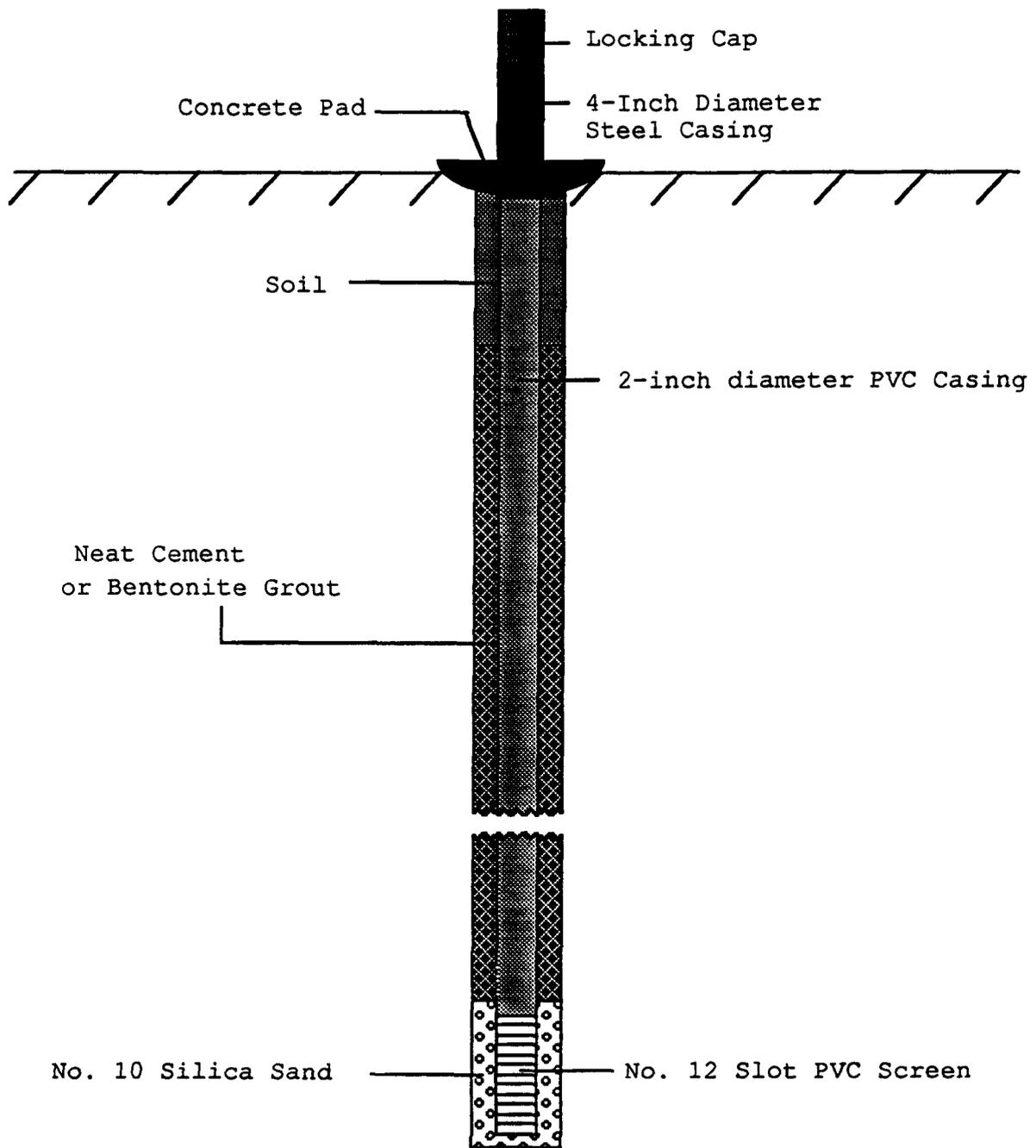
Figure 2. Construction design used for monitoring wells installed at the Casselton landfill.
