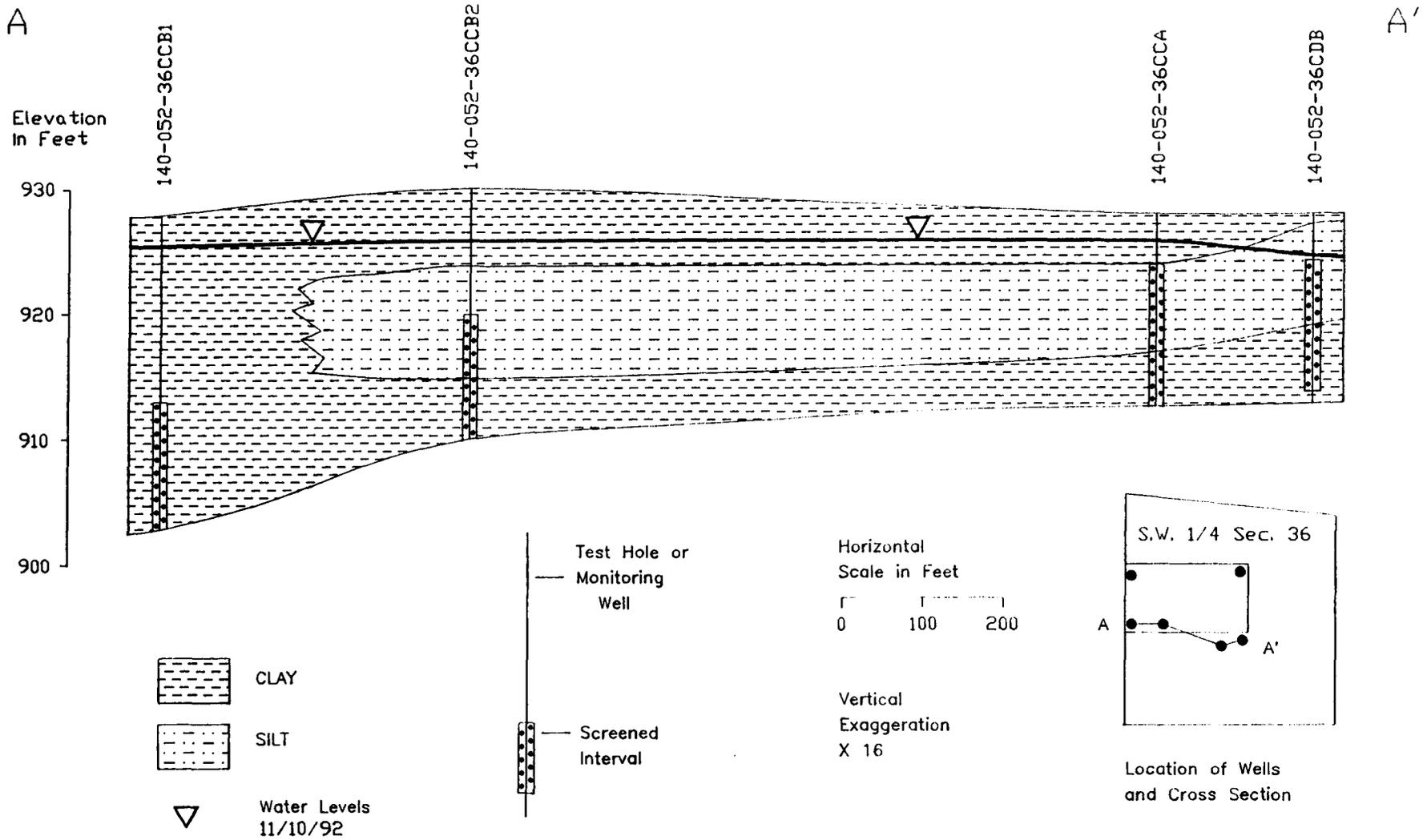
Figure 5. Geohydrologic section A-A' in the Casselton landfill.
