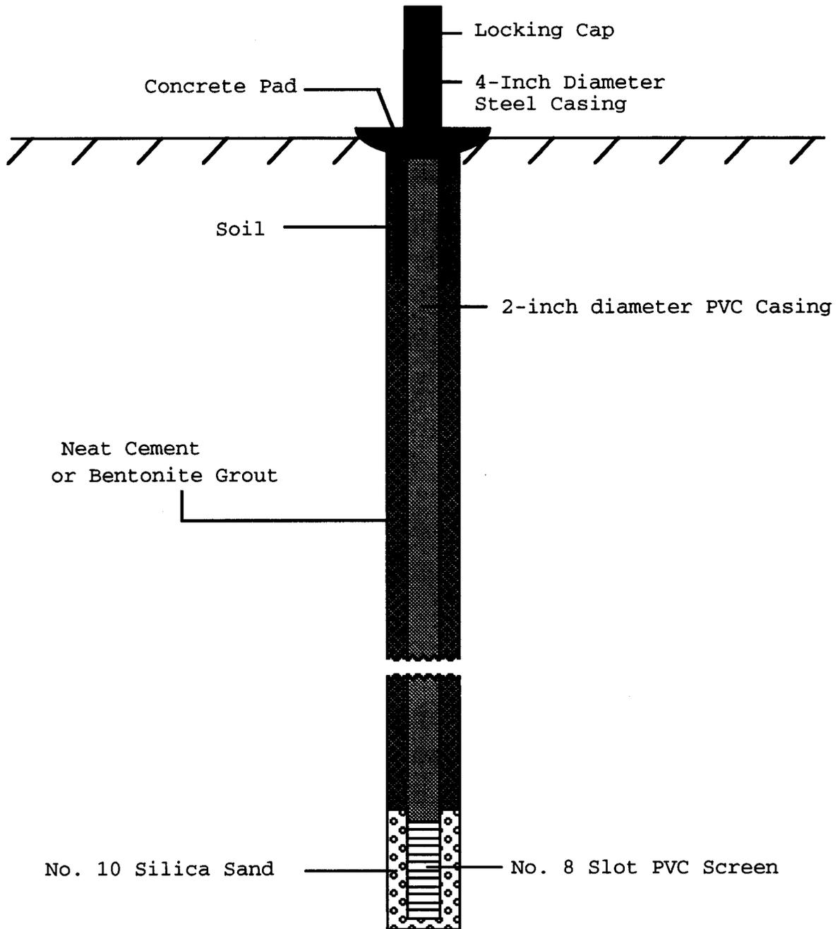
Figure 2. Construction design used for monitoring wells installed at the Beach landfill.
