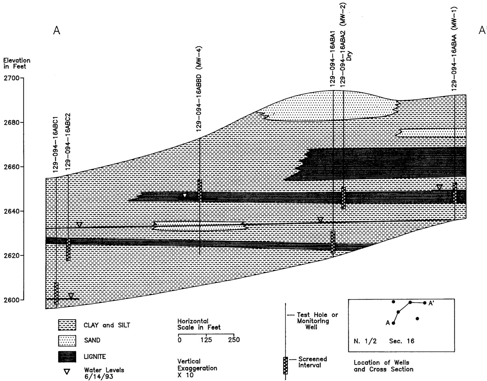
Figure 5. Geohydrologic section A-A' in the Adams County landfill.
