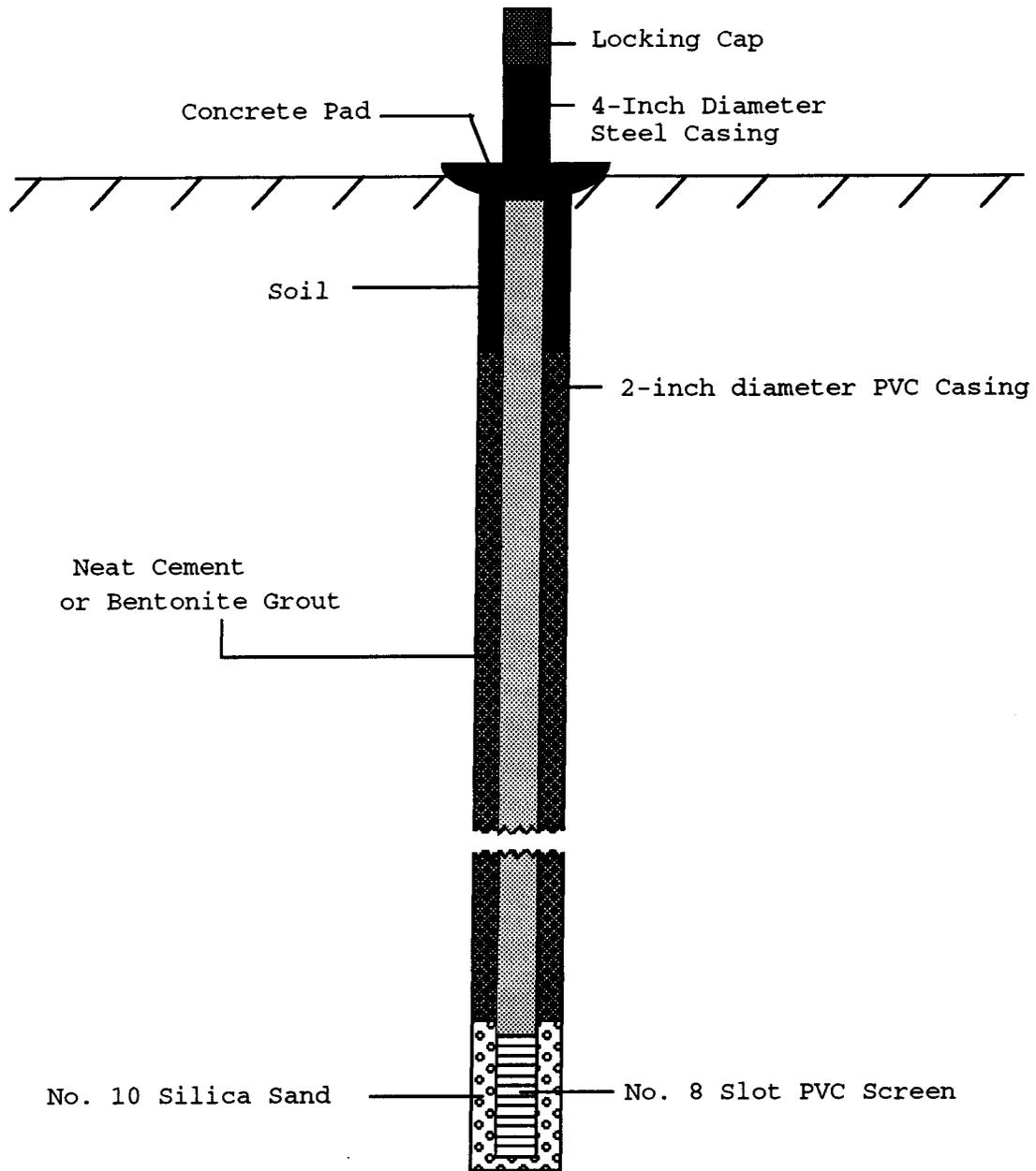
Figure 2. Construction design used for monitoring wells installed at the Adams County landfill.
