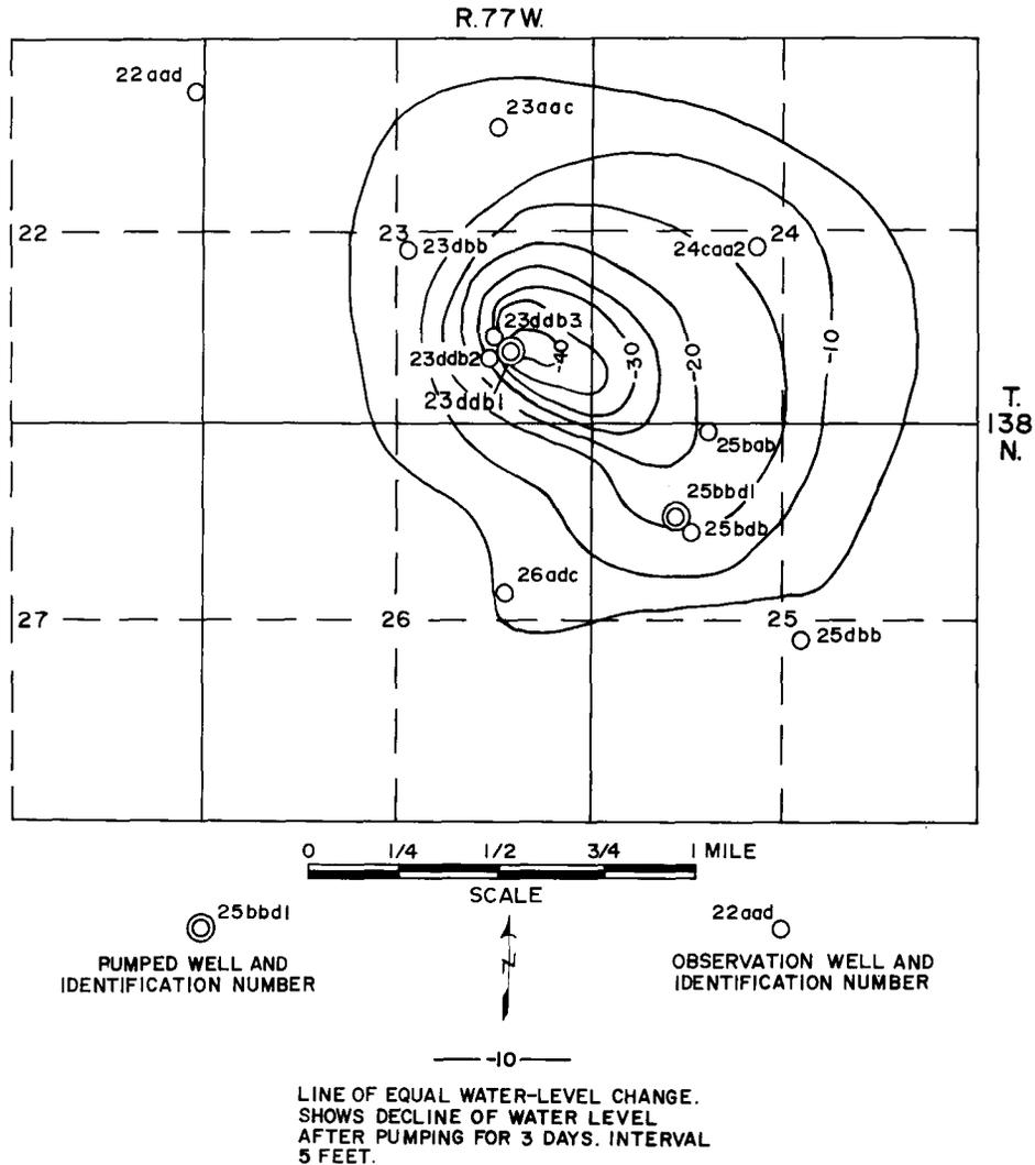
**Figure 11.**—Location of wells used during McKenzie aquifer tests 1 and 2, and area of influence resulting from test 1.
