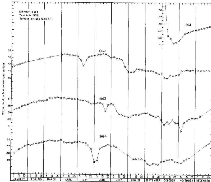
Figure 25.—Water-level fluctuations in wells in the Bismarck aquifer.
