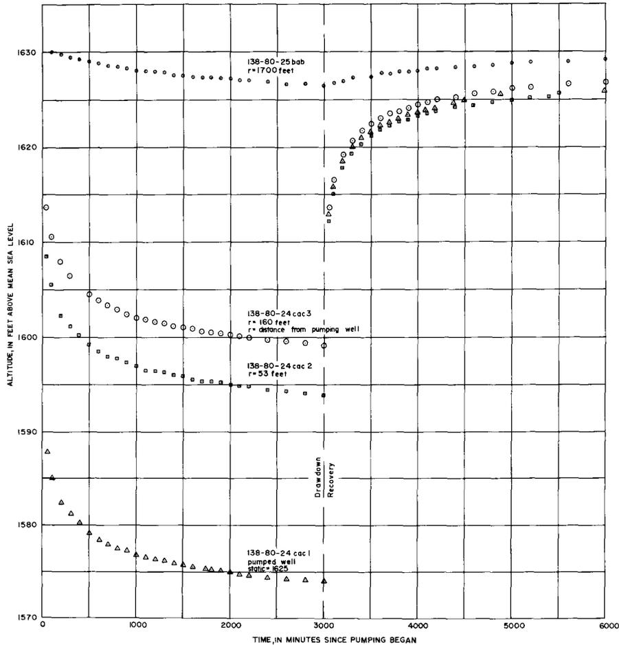
Figure 18.—Drawdown and recovery curves for Lower Apple Creek aquifer test.
