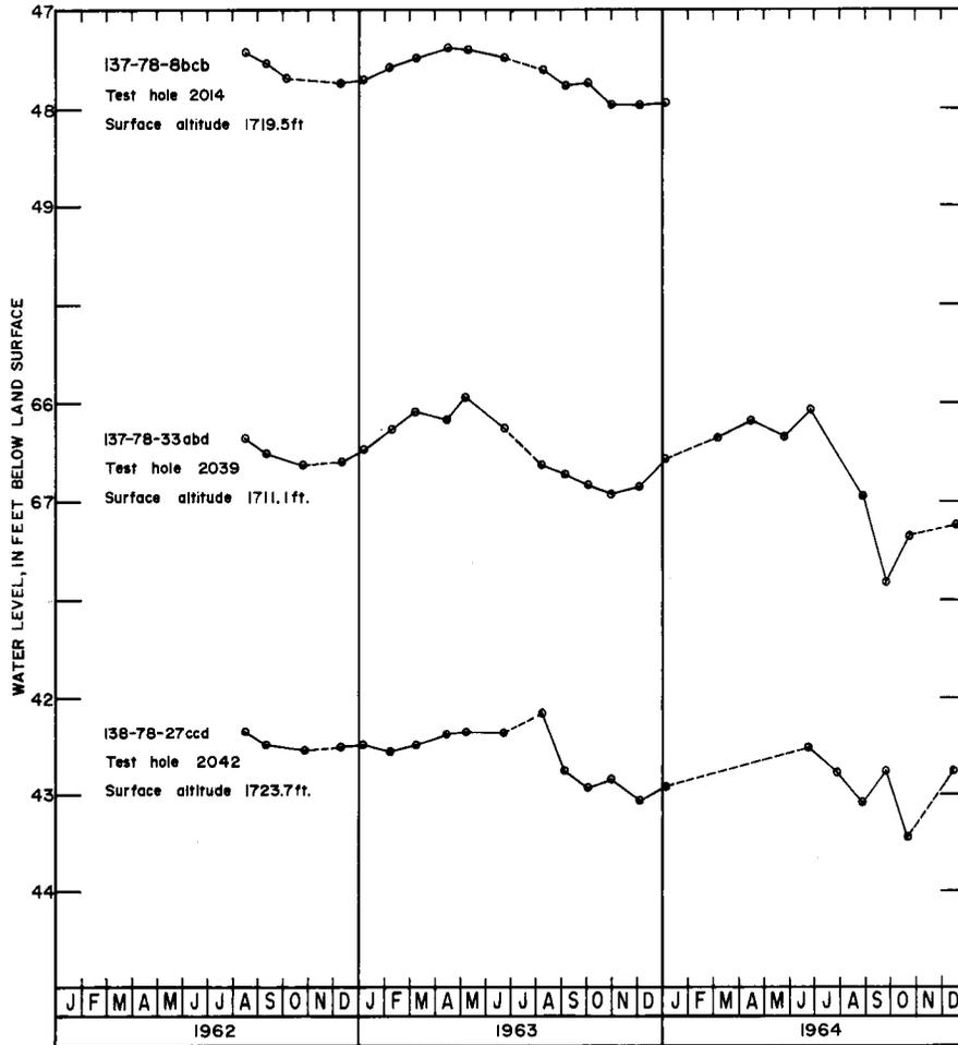
Figure 20.—Water-level fluctuations in wells in the Glencoe Channel aquifer.
