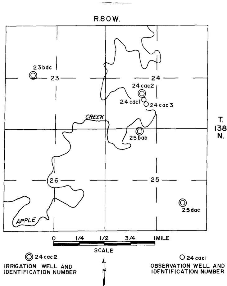
Figure 17.—Location of wells used in Lower Apple Creek and Soo Channel aquifer tests.
