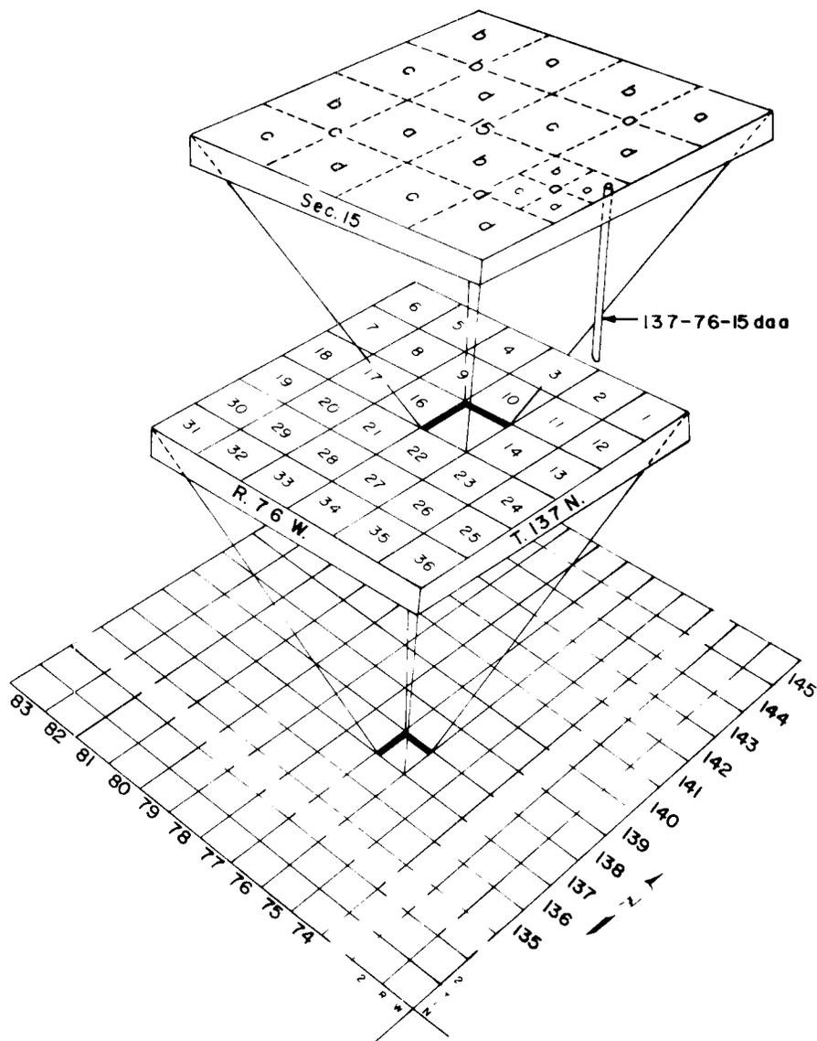
**Figure 2.**—System of numbering wells and test holes.
