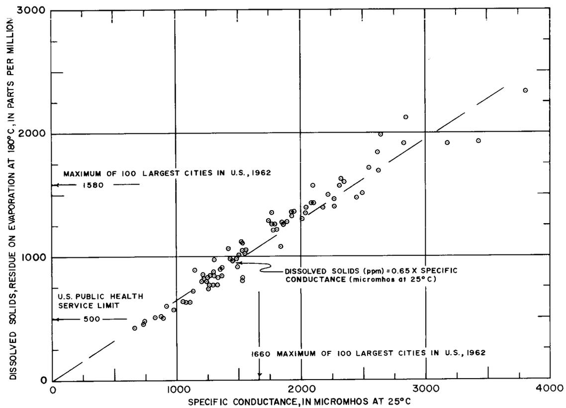
Figure 4.—Specific conductance versus dissolved solids for ground-water samples.
