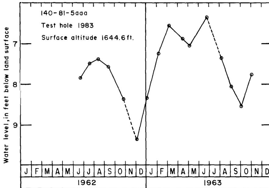
Figure 27.—Water-level fluctuations in a well in the Wagonsport aquifer.
