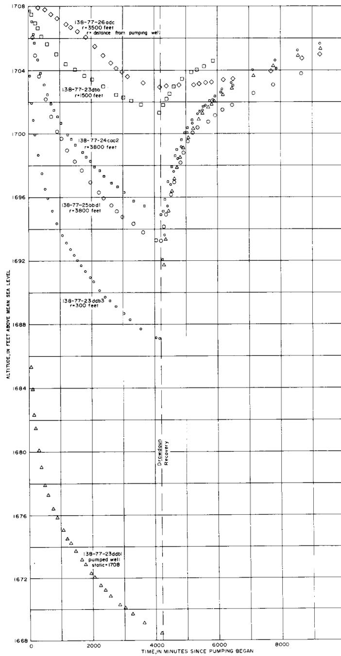
Figure 8.—Drawdown and recovery curves for McKenzie aquifer test 1.
