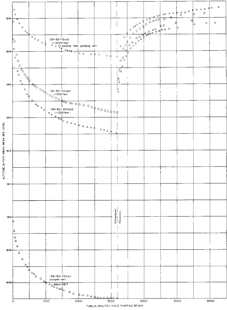
Figure 24.—Drawdown and recovery curves for Bismarck aquifer test 2.
