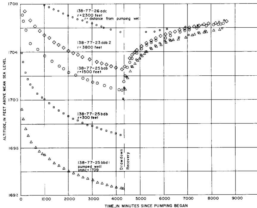
Figure 12.—Drawdown and recovery curves for McKenzie aquifer test 2.
