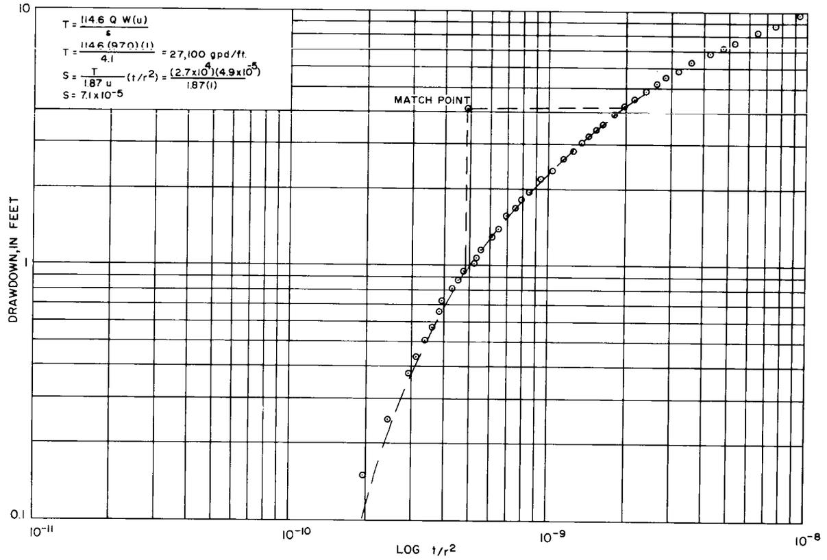
Figure 9.—Log plot of drawdown versus  $t/r^2$  for well 138-77-24caa2, Mc Kenzie aquifer test 1.
