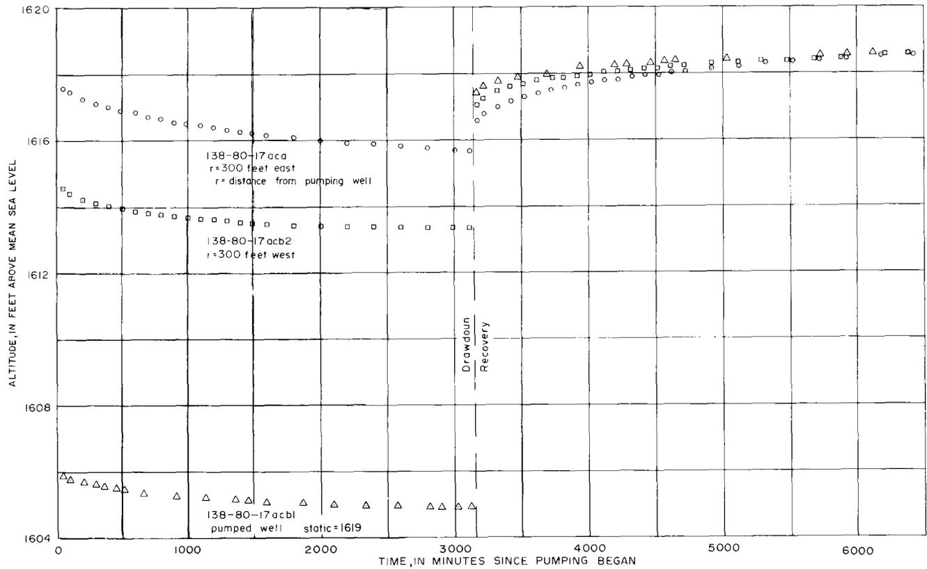
Figure 22.—Drawdown and recovery curves for Bismarck aquifer test 1.
