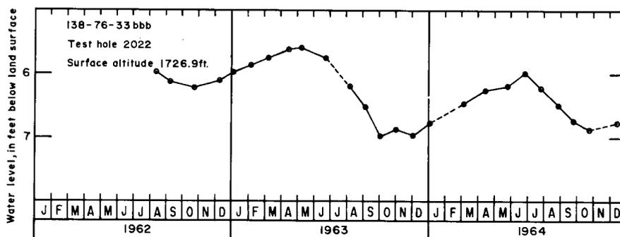
Figure 16.—Water-level fluctuations in a well in the Long Lake aquifer.
