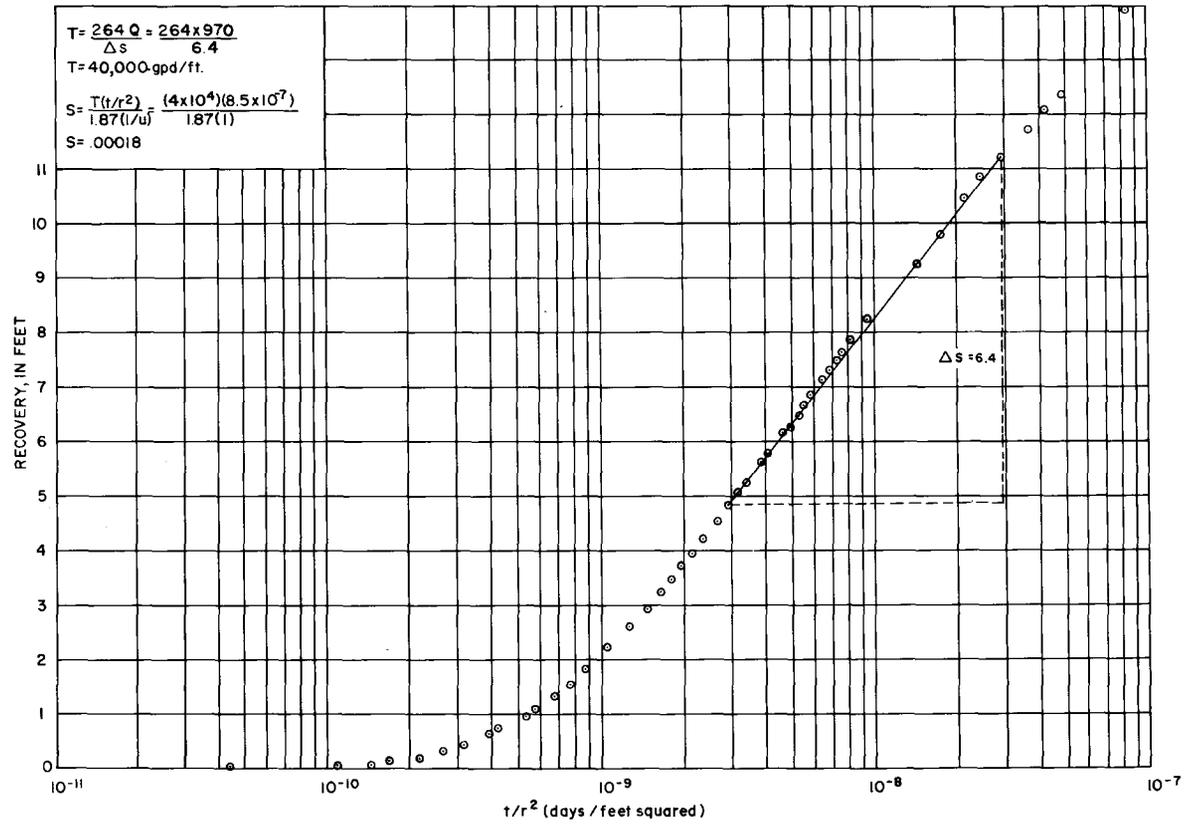
Figure 10.—Semilog plot of recovery versus  $t/r^2$  for well 138-77-25bdbl, McKenzie aquifer test 1.
