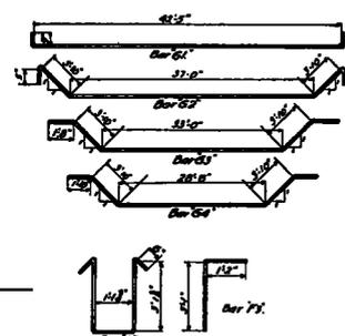
Details of Bent Bars. No scale.
